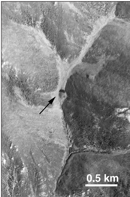
Figure 16. Arrow indicates an open system pingo in a typical setting in the nearly continuous permafrost terrain of Dawson Range. The pingo is situated along the toe of a slope composed of blanket bog, alluvial fans, and colluvial blankets. A cross-section of the deposits comprising the pingo would be similar to that shown in Figure 15. NAPL A11539-360
