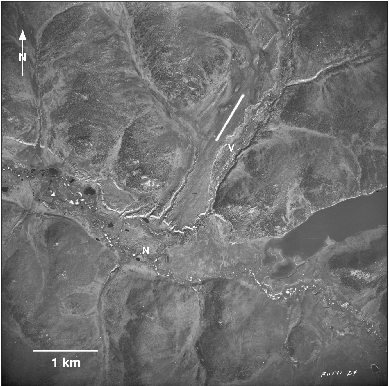
Figure 11. Airphoto of a terrace in the valley of Victoria Creek (V) near the confluence with the west-flowing Nisling River (N). The terrace is underlain by at least 15 m of gravel (see section 2, Map 1876A). Approximately the upper 10 m of the gravel fill was deposited during the Reid Glaciation by Victoria Creek. The Victoria Creek basin was beyond the limit of glacier ice at that time. The gravel fill was graded to the Cordilleran Ice Sheet or a lake dammed by it at the climax of Reid Glaciation. NAPLA11541-24
