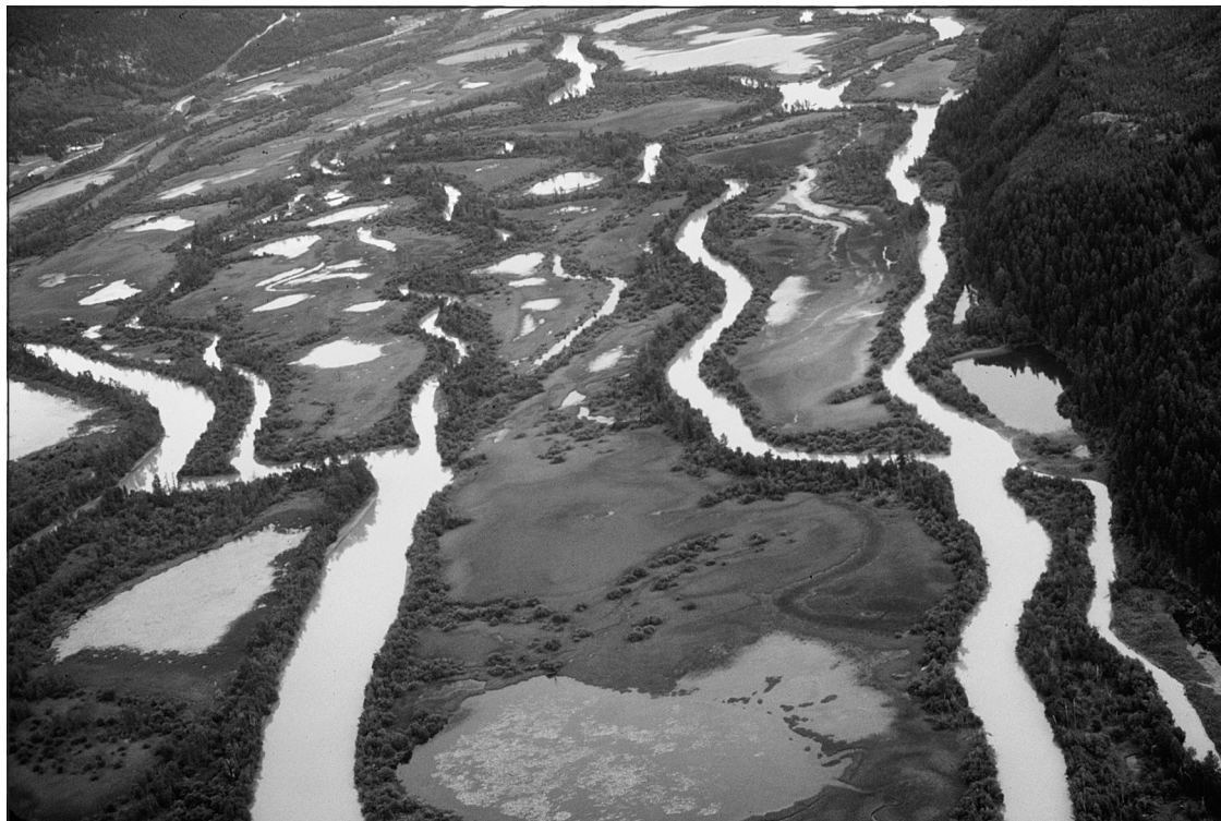
Figure A-1c. Anastomosed channel pattern in fine-grained sediment (upper Columbia River near Golden, British Columbia). Photograph courtesy of D. Smith.
