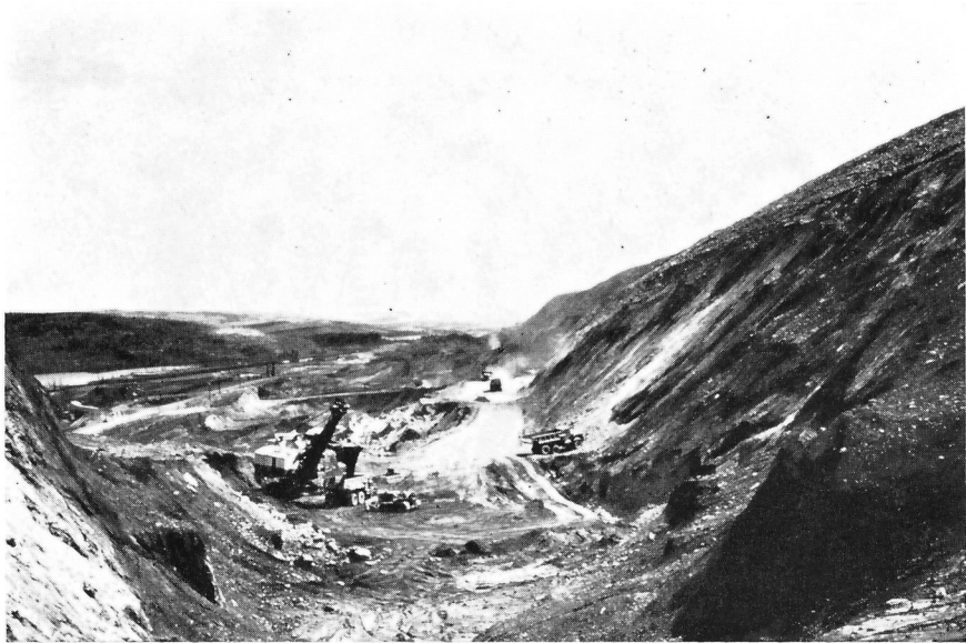
B. Gill mine, Labrador, 1957, southward. The iron ore deposit lies along the east side of a steep dip-slope.
