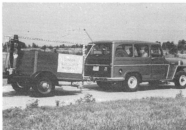
Figure 1. First experimental silver detector, 14-Mev neutron generator and boom carrying scintillation detector are in the trailer; vehicle carries control and readout equipment.
