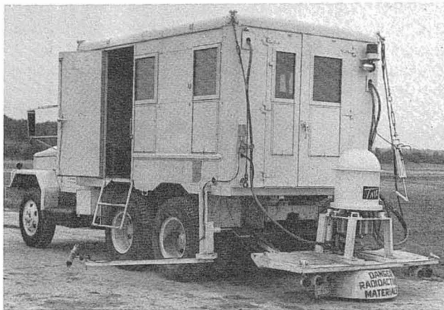
Figure 6. Mobile neutron activation laboratory showing 200-kev accelerator on tailgate in irradiation position and crystal on automatically operated boom.
