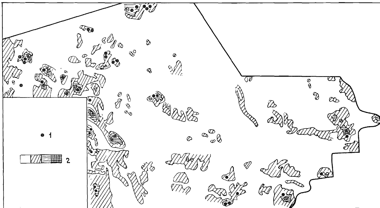
Figure 9. A plan of the distribution of the gamma-field and rare metal mineralization in Altai (according to Smilkstin, 1962). 1 – mineralization; 2 – the intensity scale of the gamma-field: from 5 to 9 microröntgen per hour; from 9 to 14 mcR/h; from 15 to 22 mcR/h; from 22 to 30 mcR/h.
