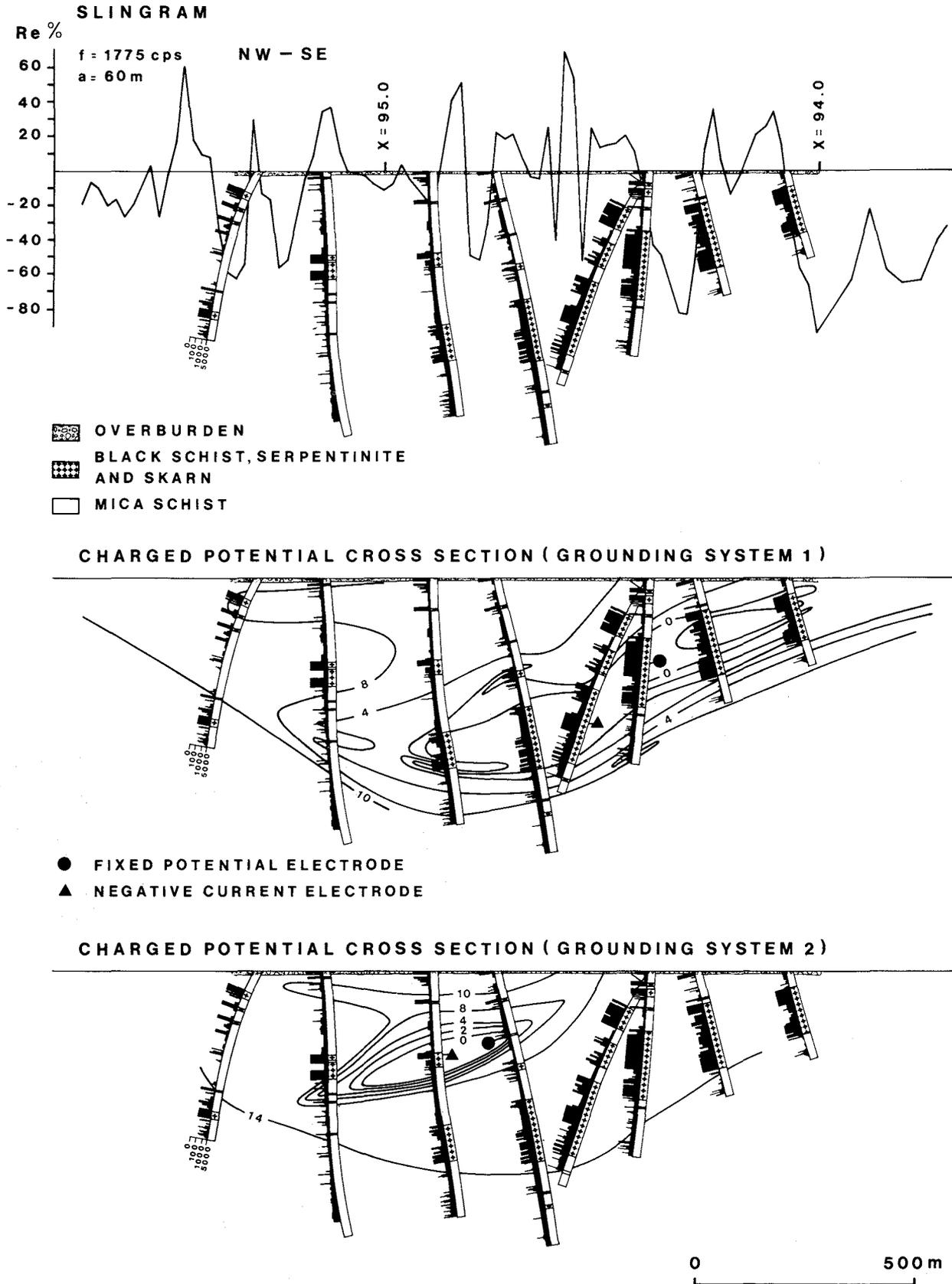
Figure 31.16. Charged potential (*mise-à-la-masse*) and resistivity cross-section  $y = 176.0$  in the Outokumpu area.
