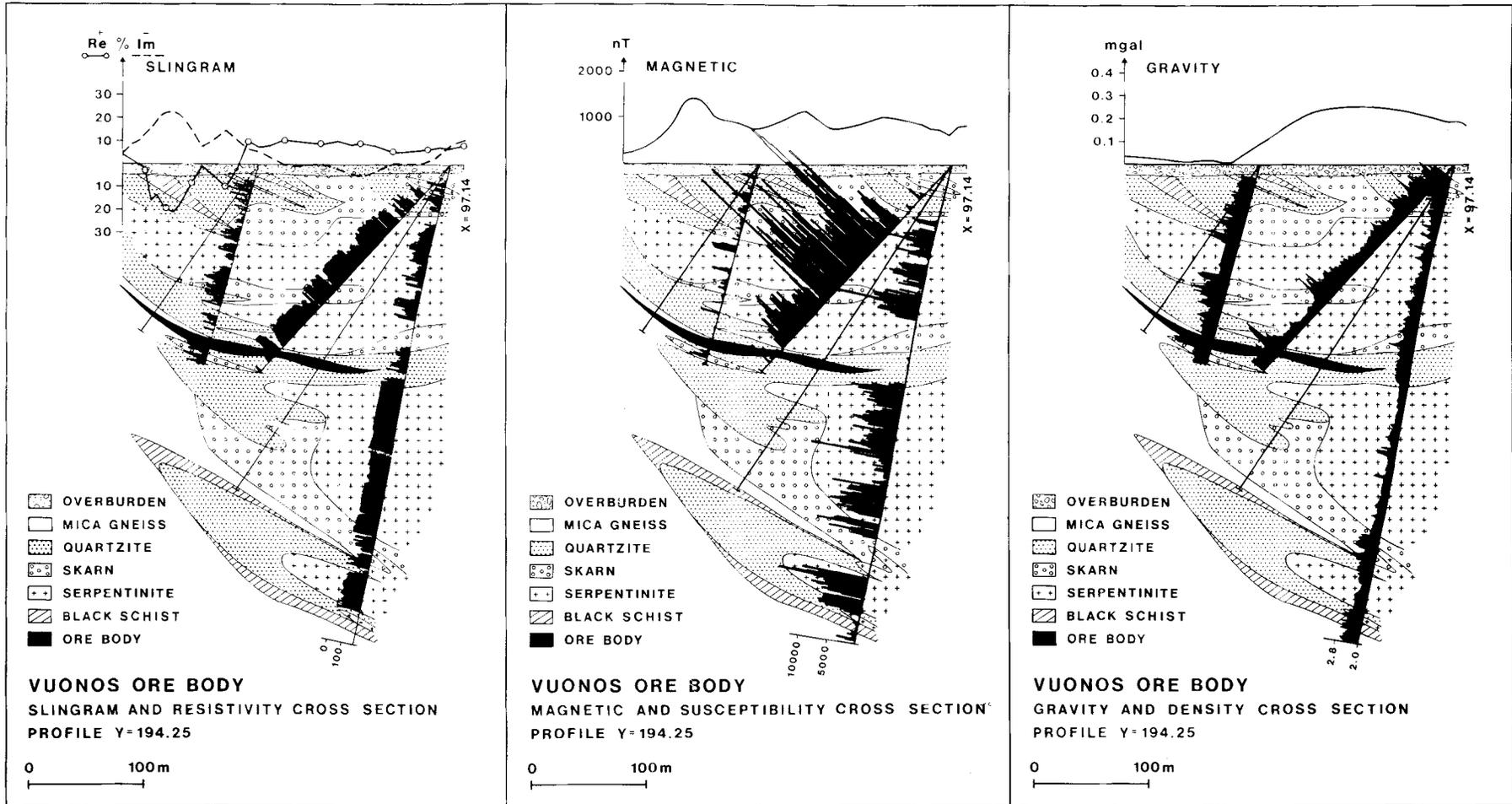
**Figure 31.3.** Geophysical and petrophysical data from profile  $y = 194.25$  in the Vuonos area. The values on the drillhole profiles are respectively in  $\Omega$ ,  $\times 10^{-5} SI$  and  $gm/cc$ .
