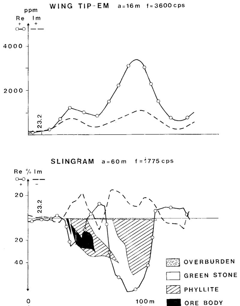
Figure 31.9. Comparison between airborne and ground electromagnetic data from profile  $x = 11.9$  in Pahtavuoma area.
