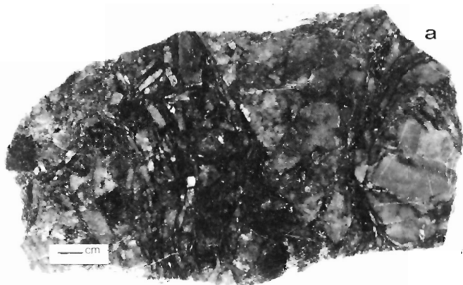
Plate 2. Felsite and ore from Mount Pleasant (17a). (a) Polished slab of felsite ore showing brecciation and arsenopyrite-wolframite-fluorite veinlets. (b) Thin section of a wolframite-fluorite veinlet in 2, showing wolframite (black) interspersed with fluorite (F). The dark grey area to the left is mostly arsenopyrite (A), light grey patches are topaz rock (T), and the remainder is mainly fine-grained quartz. (Partly reflected light, X4; (a) GSC 201964-D, (b) GSC 201964-Y)
