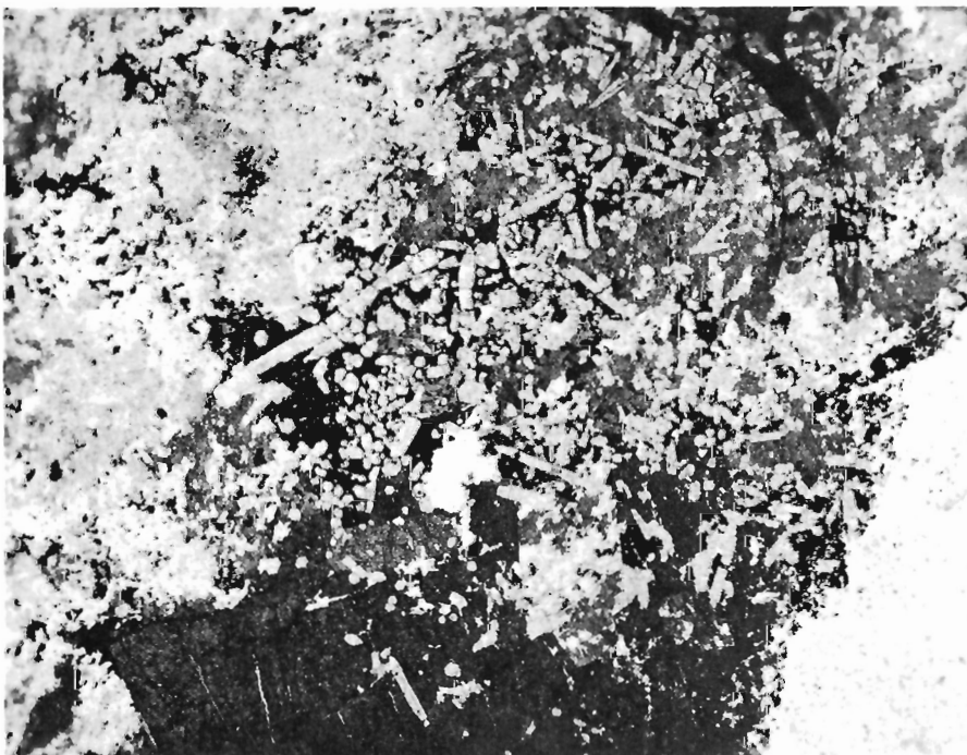
Plate 9. Slab of Canada Tungsten high-grade ore (107g). Reflected light (GSC 201964-A). Ultraviolet fluorescence (GSC 201964-B). Pyrrhotite (lightest reflection) forms a network around the scheelite and dark grains, mainly biotite. (Both X3/4)
