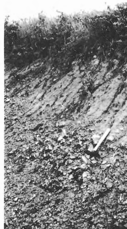
Figure 3B. Open-pit face "gravel-spar" in red soil beneath loess and turf. Dillinger Tract, Washington County, Missouri. GSC 202031-A
