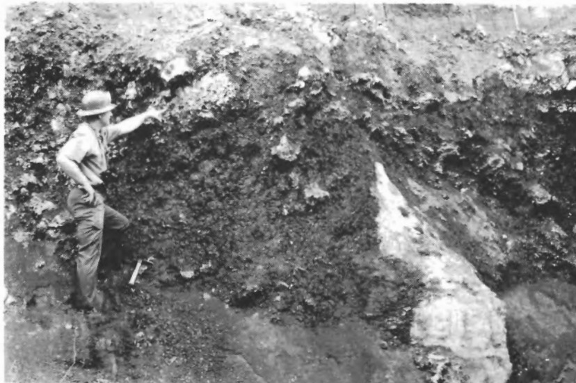
Figure 3A. Open-pit face showing residual barite in red soil and a limestone pinnacle relict of bedrock limestone. Wolf Mine, Washington, County, Missouri. GSC 202886-R
