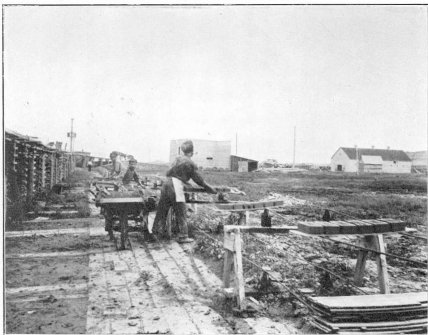
Conveyer and drying racks for soft mud bricks at Alsip's brickyard, Winnipeg, Man.
