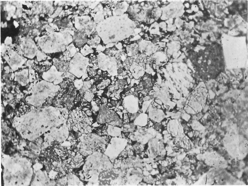
PLATE VII B. Greywacke of unit 9. Abundant fresh augite and lithic fragments, with quartz, feldspar, and carbonate. Grain at right of centre is quartzitic gneiss. Plane-polarized, X27.
