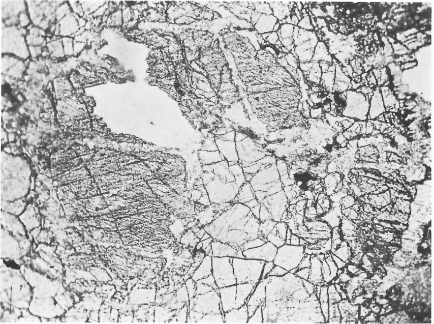
PLATE IX A. Peridotite, unit 11. Fresh olivine (irregular cracks), and lamellar structure of broken, distorted enstatite grains. Plane-polarized, X27.
