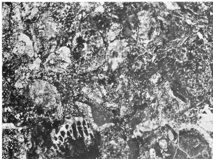
PLATE VIII B. Calcarenite of unit 9 showing rounded composite carbonate grains. Unpolarized light, X7.
