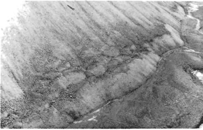
Figure 29. Oblique aerial view of a rock glacier (talus glacier) with multiple transverse ridges near the south shore of Aston Bay. The feature is formed by slow flow caused by deformation of ground ice under the weight of the coarse scree. The active frontal lobe of the rock glacier (light-toned area abutting the small stream) is 8 to 10 m high. GSC 203508-N
