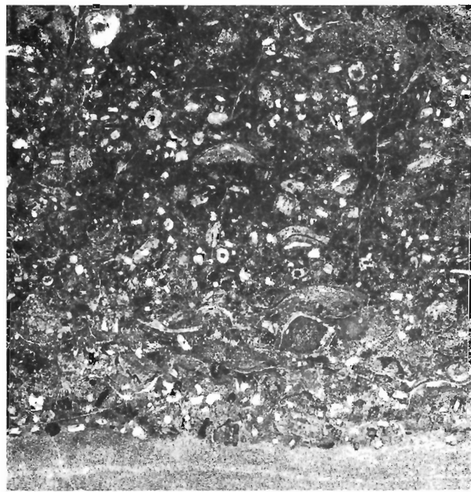
Figure 28. A polished sample from the turbidite bed shown in Figure 27. The light coloured material in the matrix is orange and yellow, argillaceous material derived from the underlying bed (ISPG Photo No. 1451-3).
