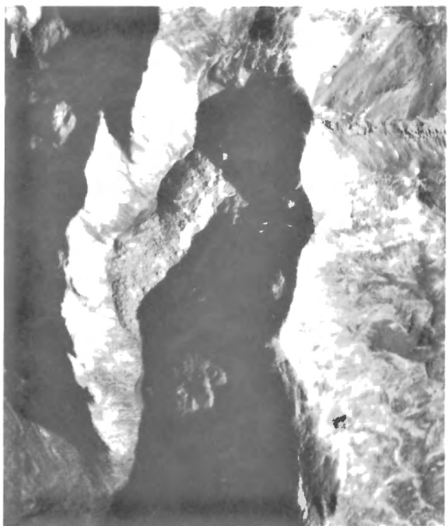
Figure 30. Large rock avalanche in cirque between Hyland River and Little Hyland River valleys (Map 1677A). Individual blocks easily distinguishable on surface. Part of NAPL A12797-60; approximate scale 1:30 000
