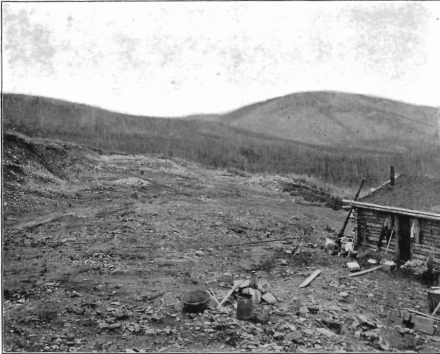
Graham's bench workings on the left side of Barker creek, near the head of the stream. Bedrock on this bench is 85 to 90 feet above the level of the creek opposite. The view shows the nearly flat character of the bedrock, and the shallowness of the gravels, which are from 3 to 6 feet thick in most places. From the cut shown, which is nearly 500 feet long by 100 feet wide, $10,000 in gold is believed to have been obtained.
