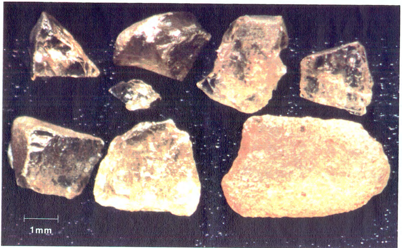
Plate 4: Amber colored, rounded zircon macrocrystals with whitish alteration rims from the (SK) Saskatchewan Sturgeon Lake, kimberlite. Although such zircons are frequently present in Southern African kimberlites, zircon macrocrystals were only present in the SK kimberlite sample.
