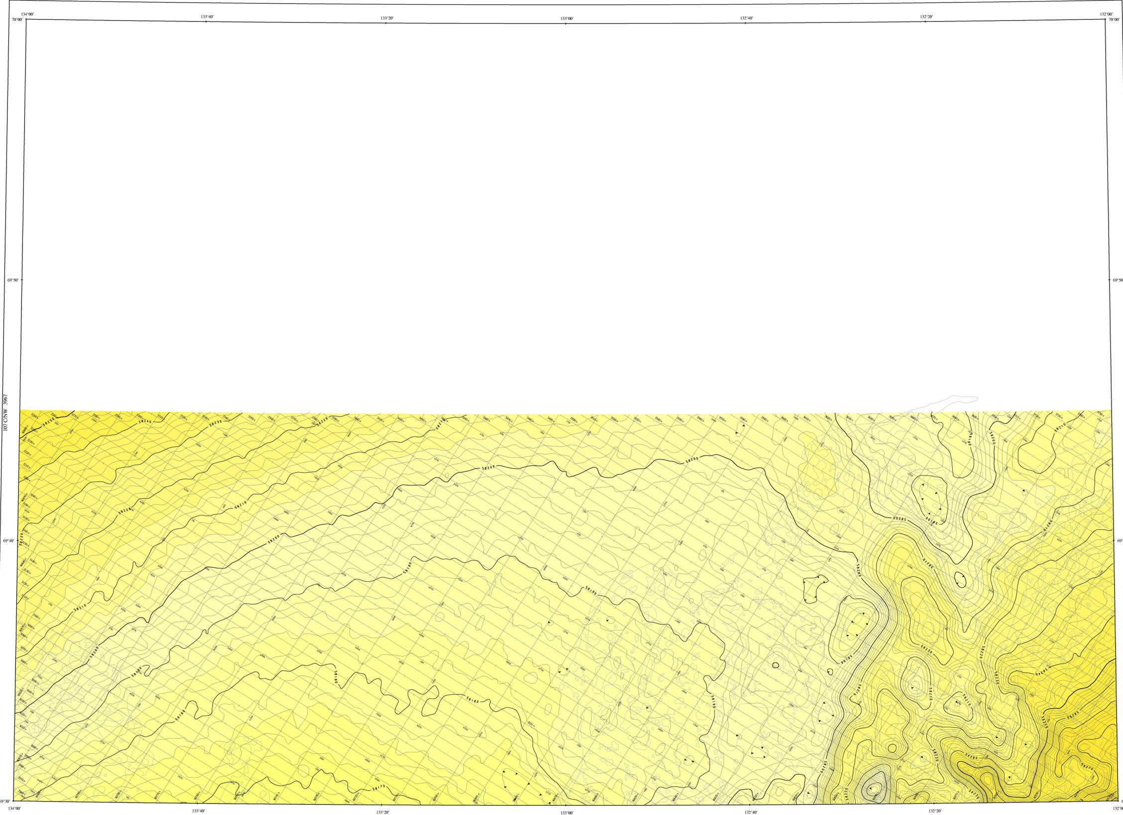
This map was compiled from data obtained as a result of an aeromagnetic survey carried out by Goidak Exploration Ltd. using a Piper PA-31 Navajo (registration C-GUBA) aircraft. A 0.005 nT sensitivity split-beam cesium vapour magnetometer was mounted in the tail boom of the survey aircraft.
