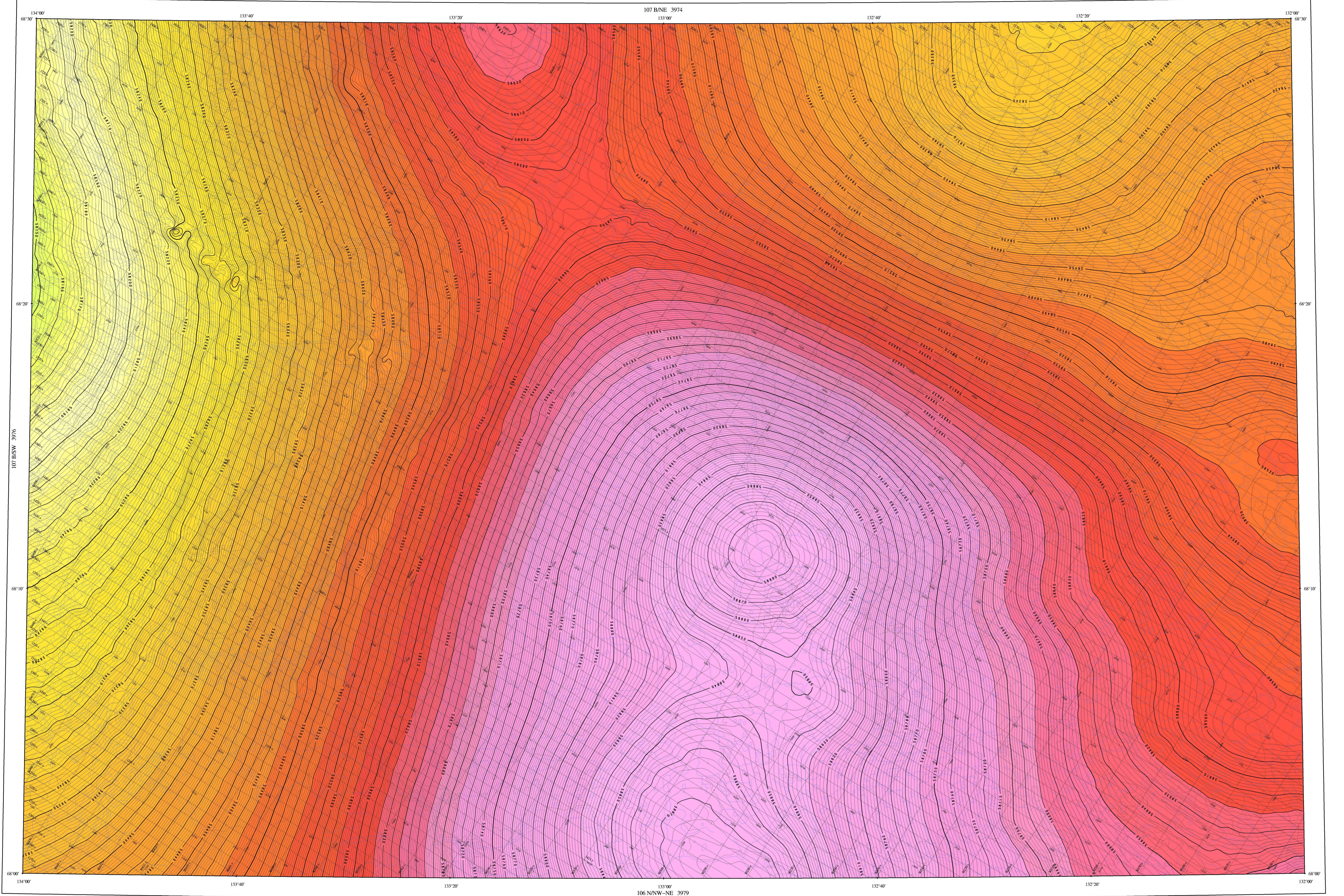
This map was compiled from data obtained as a result of an aeromagnetic survey carried out by Goldak Exploration Ltd. using a Piper PA-31 Navajo (registration C-GJBA) aircraft. A 0.005 nT sensitivity split-beam cesium vapour magnetometer was mounted in the tail boom of the survey aircraft.
