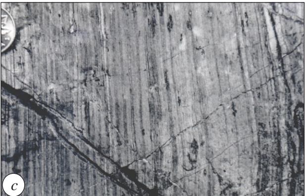
c. Flaser fabric of mylonite of the Nisutlin allochthon in a specimen from near Grass Lakes. The rock consists mostly of quartz and sericite.
