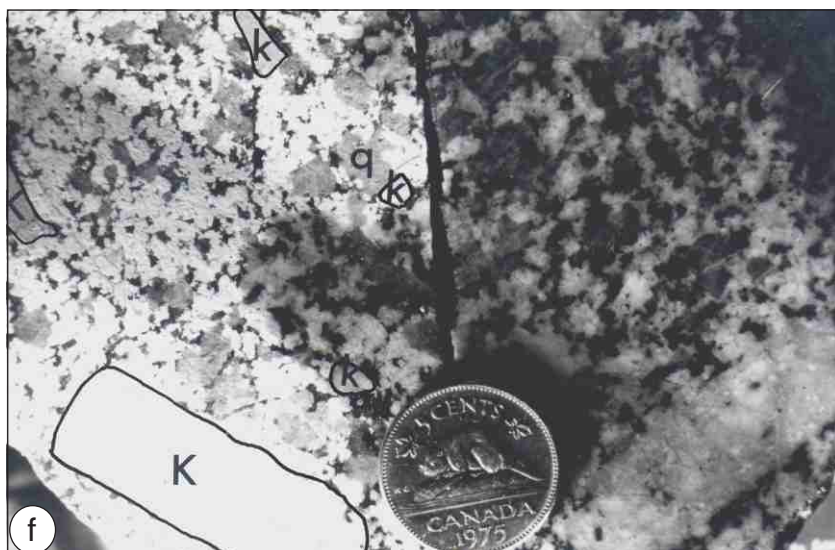
f. Quartz monzonite from the Quiet Lake batholith illustrates the texture of porphyritic rock. The specimen on the left was stained; that on right is the sawn surface. Potassic feldspar (K, k) is outlined; quartz grains (q) are anhedral, equant and medium grey. The small black irregular crystals are biotite; oligoclase is white. Canadian nickel is 2.0 cm diameter.
