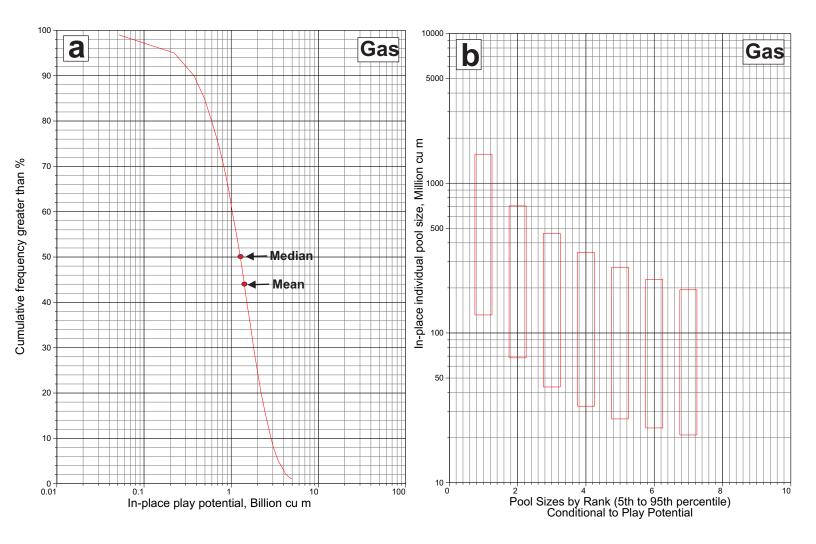
Figure 25. Estimate of in-place gas (a) potential of the Lower Paleozoic carbonate pre-Laramide structural play.. Pool-size-by-rank plot (b) of the play is also displayed.
