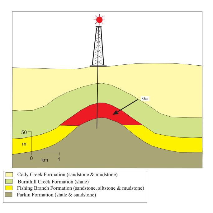
Figure 70. Schematic cross-section illustrating potential trap configurations in the Cretaceous sandstone structural oil and gas play. Illustrated trap is an anticlinal fold. From National Energy Board, 2000.
