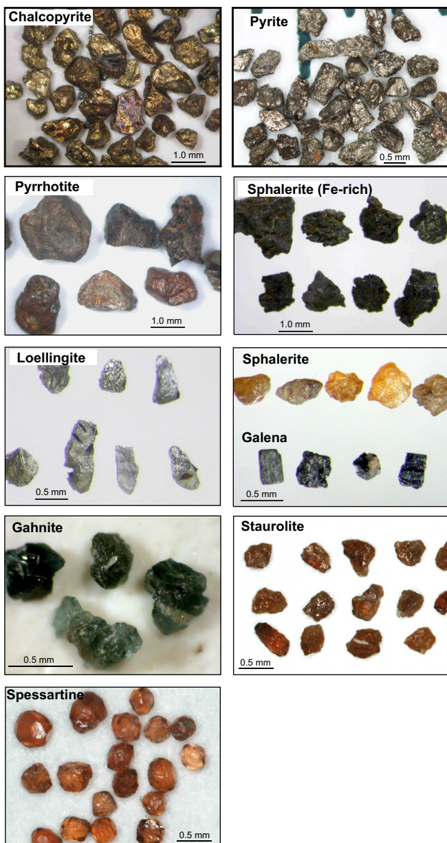
Figure 4. Photographs of selected VMS indicator minerals as they appear in heavy mineral concentrates of till from around VMS deposits.
