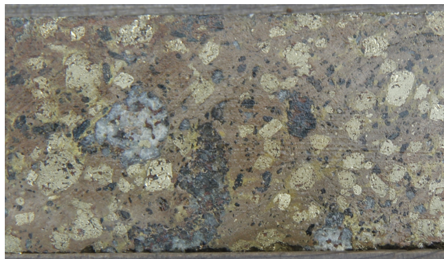
Figure 7. Photograph of classic durchbewegung texture (Craig and Simpson, 1991) in type 1 Fe-Zn-rich massive sulphide ore (DUB195, 809.7 m). The texture shows rounded nodules of hard pyrite and quartz nodules in a matrix of softer sphalerite. NQ drill core (47.6 mm or 1-7/8 in diameter).
