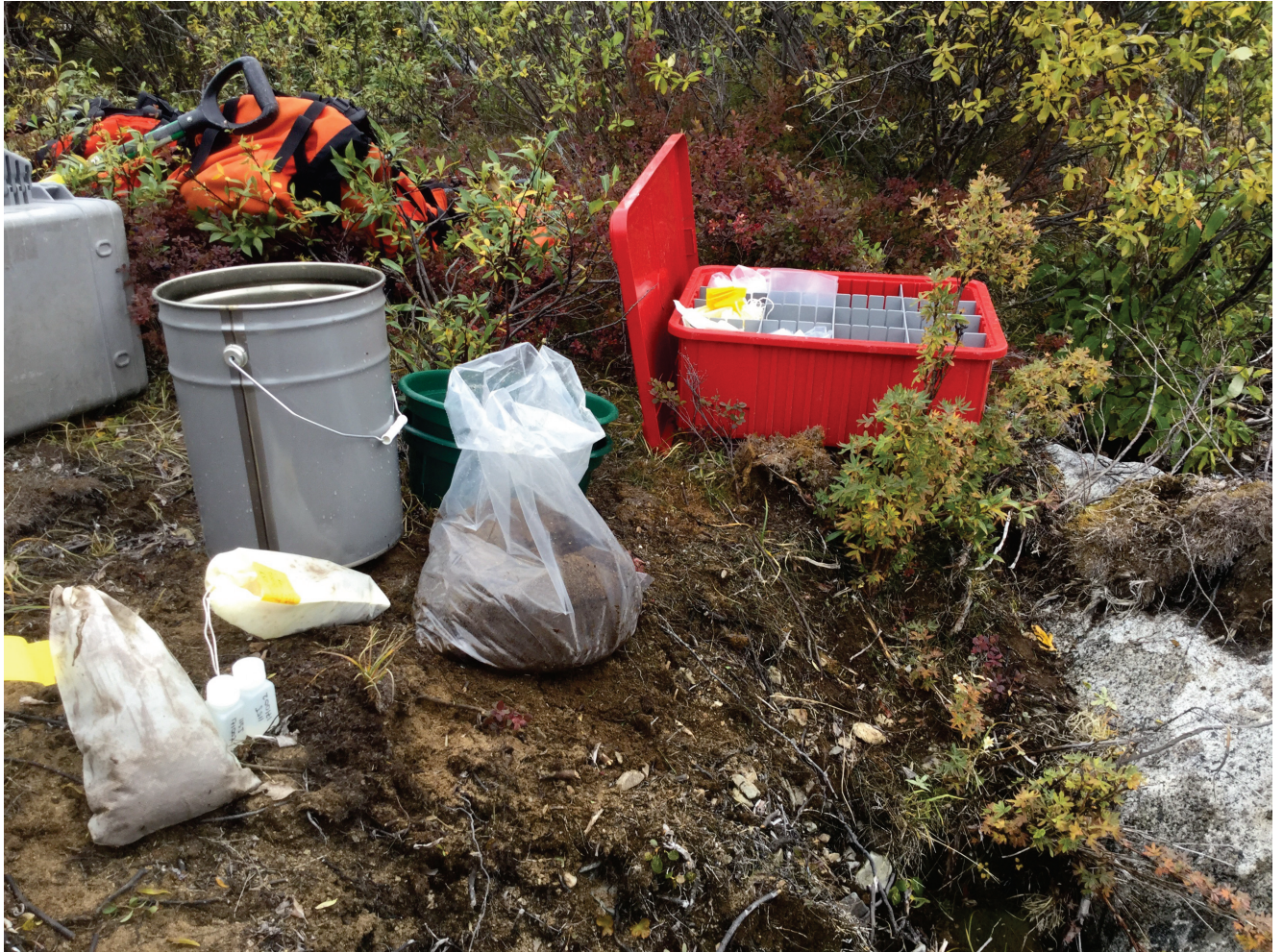
Figure 4. At each site, a stream silt sample (wet mass 1 – 2 kg), two 60-ml filtered stream water samples, a bulk stream sediment sample (wet mass 10-15 kg) and a stream pebble sample (in synthetic bag beside bulk sample) were collected.
