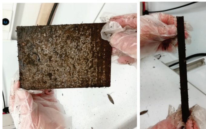
Figure 17: Slicing and sub-sampling protocol devised by the SWAMP laboratory, University of Alberta for MAC cores sliced at 1 cm intervals and showing division of living layer from peat. Photo credit: A. Oleksandrenko, University of Alberta, 2020.
