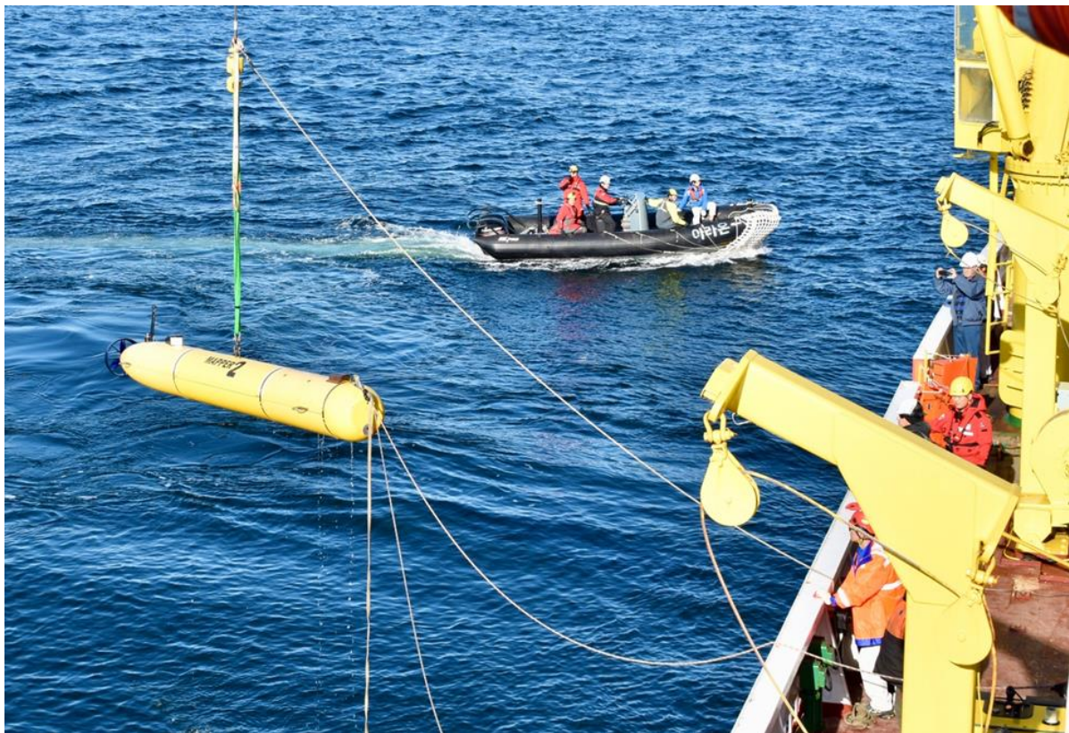
Figure 3.1. Recovery of MBARI Mapping AUV 2 following a mission to survey a mud volcano at 740 m depth during ARA13C. Photo courtesy of Monterey Bay Aquarium Research Institute.
