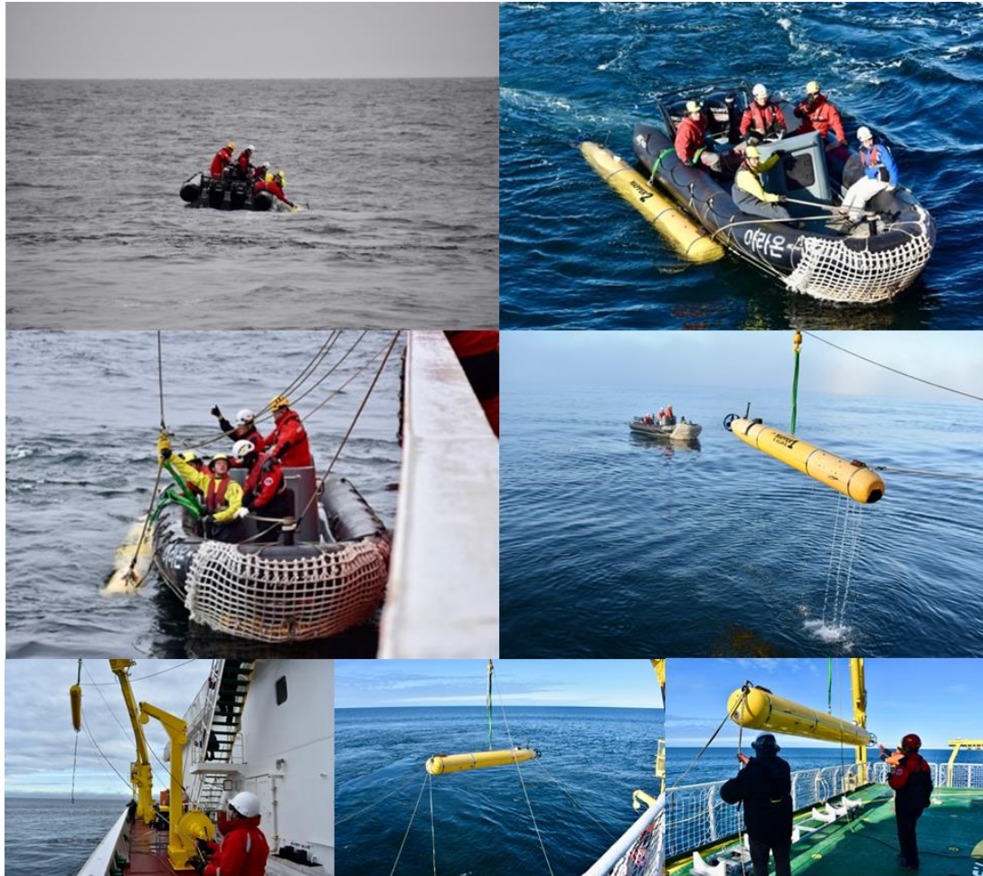
Figure 3.5. AUV recovery sequence. (Top left) After positioning the ship so that the AUV was floating less than 200 m off the starboard side, the small boat was launched with three Araon crew and two MBARI AUV engineers. (Top right) The AUV was secured to the starboard side of the small boat with a line from the top nose bale to the boat's forward cleat, and the towing/recovery line, utilizing a stainless-steel hook, from the main lifting bale, to the boat's aft starboard cleat. It was important to secure the lines to the boat as the AUV's drag was too great for the lines to be held directly. The AUV was then side towed back to the ship. (Middle left) The boat approached the starboard side of the ship and was secured using the boat's fore and aft mooring lines, with the AUV still secured outboard from the ship. Once the boat was stably secure to the ship, the crane head was lowered over the AUV with a double tag line clipped on. The tag line was unclipped from the crane head and clipped onto the AUV top nose bale, and then the towing/lifting strap was attached from the AUV's lifting bale to the crane head hook. (Middle right) After the boat's mooring lines were released, the boat backed away from the ship and the AUV was lifted out of the water. (Bottom) A second tag line was attached to the AUV's tail before it was brought aboard directly to the helideck. Photos courtesy of Monterey Bay Aquarium Research Institute.
