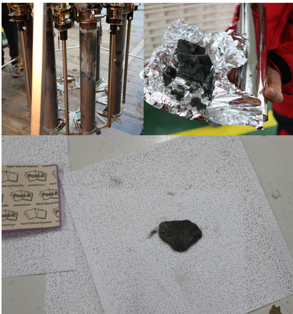
Figure 2.7. Gas hydrate samples, mud volcano 420 m. Photos courtesy of Korea Polar Research Institute.
