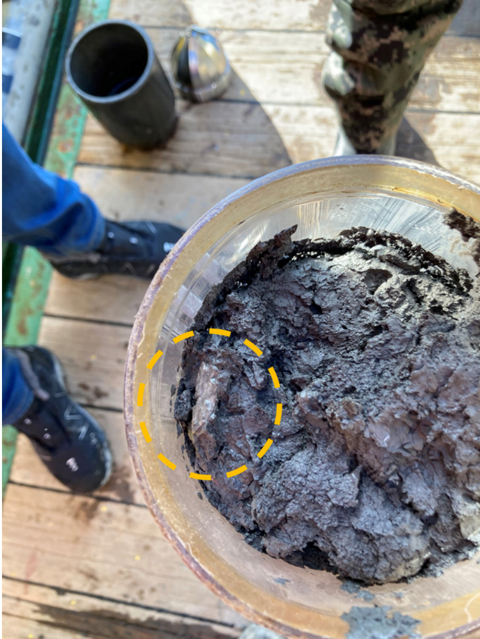
Figure 2.10. Gas hydrate samples, mud volcano 780 m. Orange circle indicates the gas hydrate sample in the gravity coring barrel. Photo courtesy of Korea Polar Research Institute.
