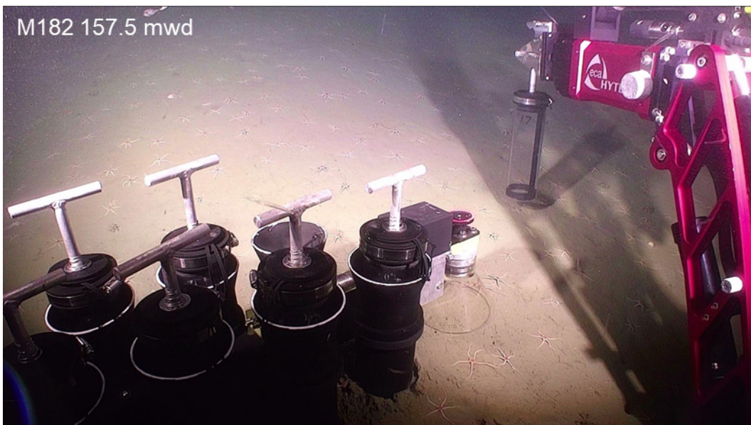
Figure 4.14. The ROV collecting push cores. Photo courtesy of Monterey Bay Aquarium Research Institute.
