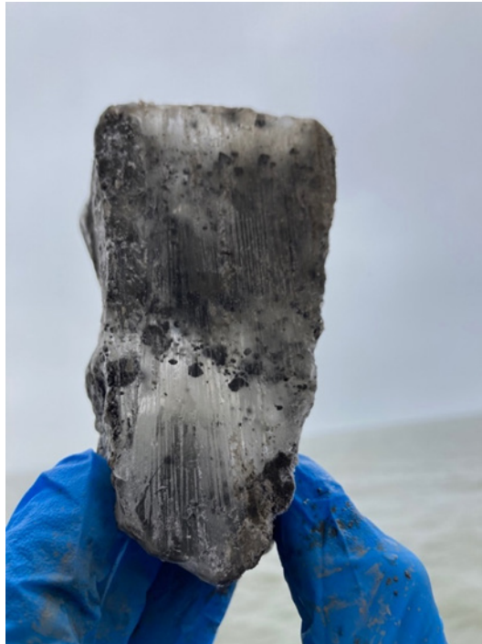
Figure 4.88. Ice was 4 cm thick, transparent and had opaque inclusions. Photo courtesy of Monterey Bay Aquarium Research Institute.
