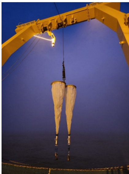
Figure 8.3. Bongo nets (150- \mu\text{m} ) used for plankton sampling. Photo courtesy of Korea Polar Research Institute.
