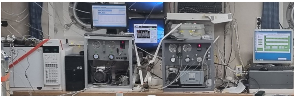
Figure 7.3. CH 4 analysis systems. Gas chromatographic system (left) and cavity ring-down spectroscopic system (CRDS) (right) were operated to measure the methane dissolved in the seawater and the air. Photo courtesy of Korea Polar Research Institute.
