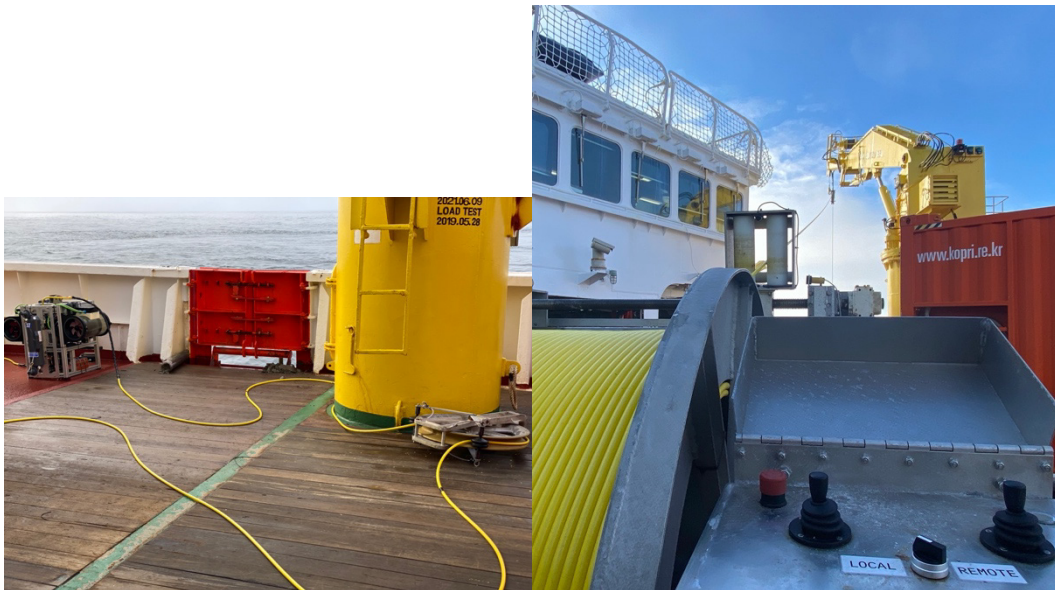
Figure 4.4. Photos showing the smart clump (cube shaped device) and turning block (wheel and cable) on the deck used to feed the tether to the ROV. The winch is shown in the foreground with the turning block suspended from the crane in the background. After the ROV is launched the tether between the ship and the clump weight is passed through the turning block suspended below the crane. The winch was operated using control box with instructions communicated via hand held radio from the control room. Photos courtesy of Monterey Bay Aquarium Research Institute.
