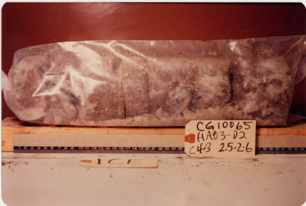
PHOTO 6: Massive ground ice (ICE), with very minor inclusions of soil (Borehole HA83-D2, Sample C4).
