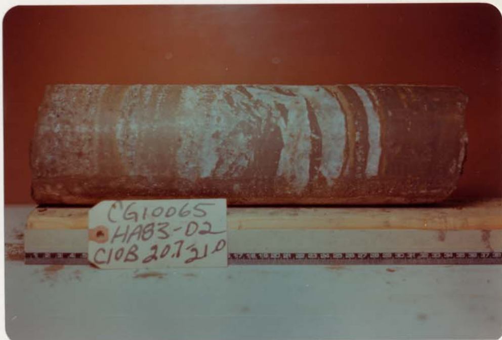
PHOTO 7: Ice-rich silty, low plastic, clay (ICE+); upper 5 cm of core consists of ice-rich sand. Note: light brown, organic-rich interbeds towards bottom of core (Borehole HA83-D2 Sample C10).
