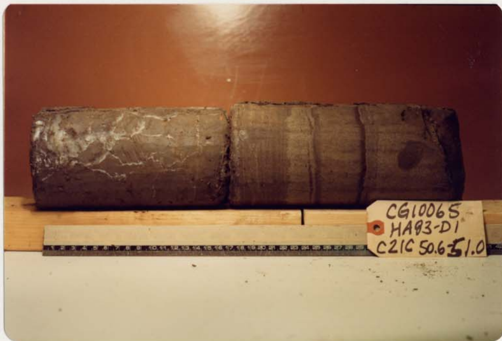
PHOTO 3: Medium plastic silty clay lens, with random and reticulate ice veins (Vr), overlying fine to medium, low ice content (Nbn) sand with silt interbeds and organic inclusions (Borehole HA83-C1, Sample C21).
