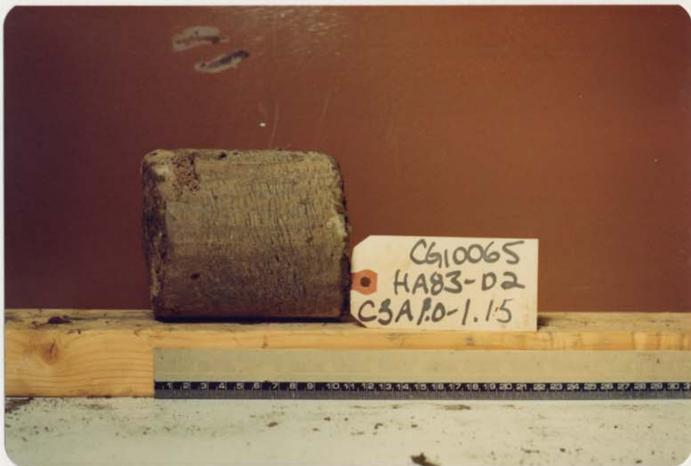
PHOTO 5: Silty low plastic clay, with prominent stratified visible ice (Vs) (Borehole HA83-D2, Sample C3).
