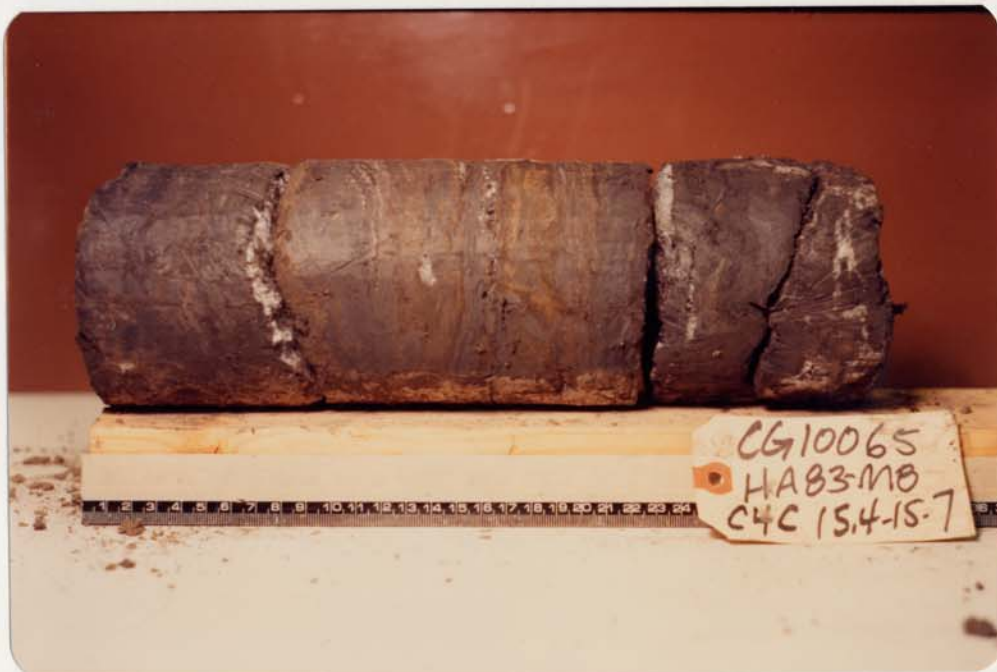
PHOTO 10: Silty clay, with brown silt lenses and random ice veins, up to 10 mm thick (Vr) (Borehole HA83-M8, Sample C4).
