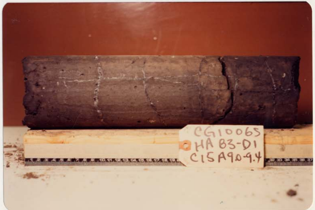
PHOTO 2: Silty clay till/diamicton, with reticulate ice veins (Vr) (Borehole HA83-D1, Sample C15).
