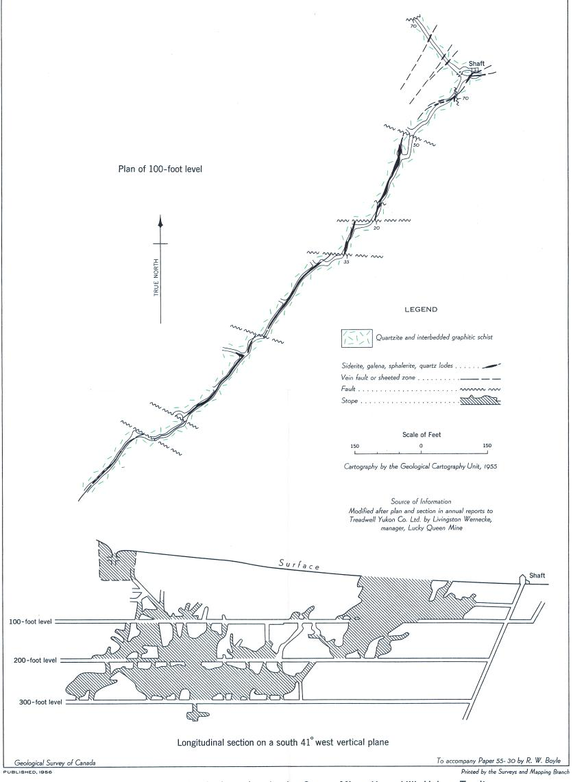
Figure 6. Plan and longitudinal section, Lucky Queen Mine, Keno Hill, Yukon Territory
