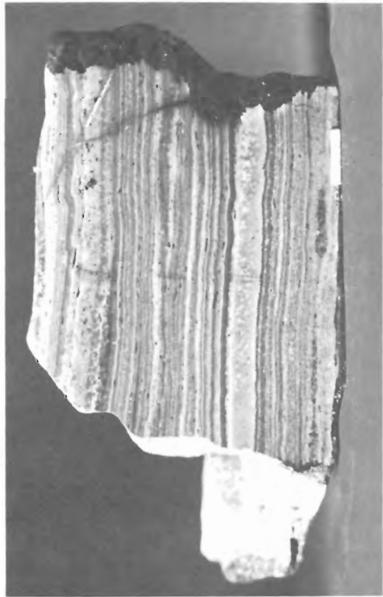
Figure 45.10. Chert- and carbonate-rich laminae and bands in iron-rich carbonate rocks; Brunswick No. 12 mine area. Length = 8 cm. GSC 202229-R
