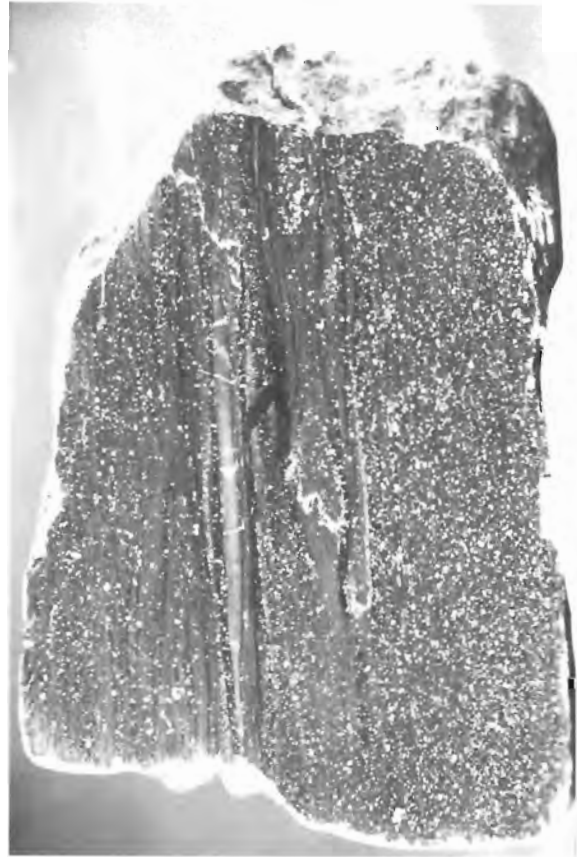
Figure 45.6. Photomicrograph showing laths and fine grains of albite, other minerals are magnetite, chlorite, quartz and carbonate; cherty magnetite iron formation, Key Anacon mine area.
