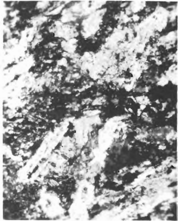
Figure 45.7. Photomicrograph showing grunerite and magnetite; cherty magnetite iron formation, from the new trench of Atlantic Coast Copper.
