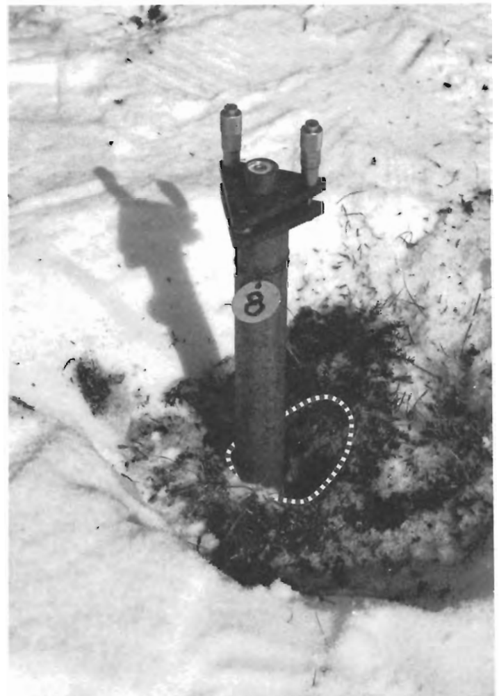
Figure 42.3. Steel tube number 8 located on the ridge of a low centre polygon. Note the cavity which has developed since 1966. The tiltmeter, on top of the tube, has been used to measure changes in tilt.
