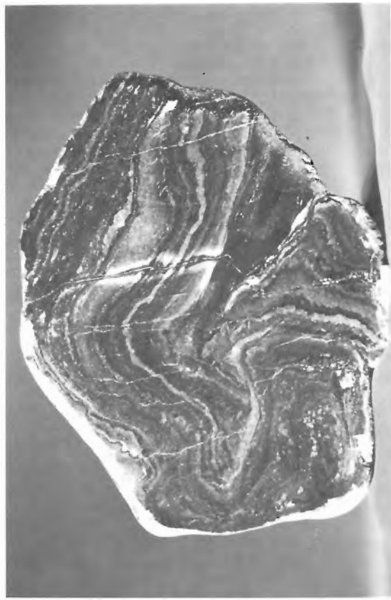
Figure 45.5. Folded and refolded (by two different phases of deformation) bands and laminae of chert alternate with magnetite-rich bands and laminae; cherty magnetite iron formation, Brunswick No. 12 mine area. Length 13 cm. GSC 202229-W
