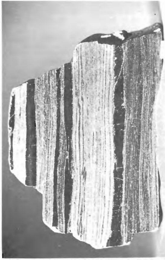
Figure 45.3. Fine laminae and thick bands of jasper alternate with magnetite-rich laminae and bands; cherty magnetite iron formation, Austin Brook iron mine area. Length = 13 cm. GSC 202229-Q
