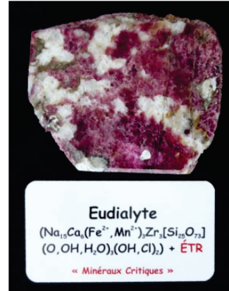
Figure 2.8: Sample of eudialyte (pink minerals) from the Kipawa deposit, located in Témiscamingue, Quebec (donated by V. Bécu and P. Mercier-Langevin). Eudialyte can contain rare earth elements, or REEs, which are essential for the manufacture of many common electronic products.
