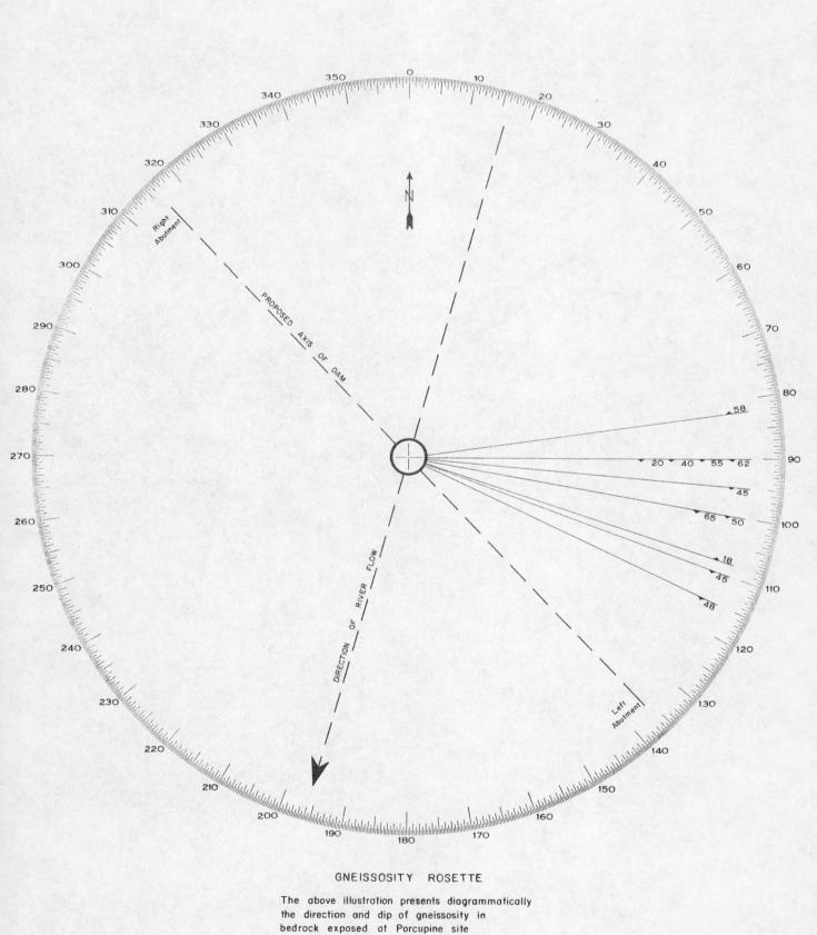
The above illustration presents diagrammatically the direction and dip of gneissosity in bedrock exposed at Porcupine site
