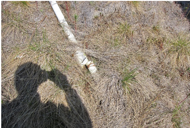
Photo 7: Break in pipe to blue lysimeter BC-70
