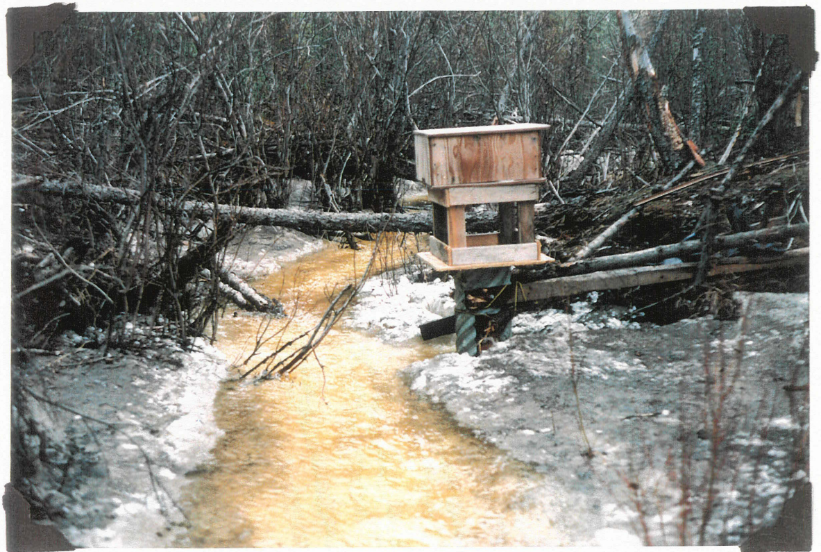
May 13, 1994. Williams Creek Data Logger station. Flows remain on top of ice. Ice decreased a further 0.4 meters.
