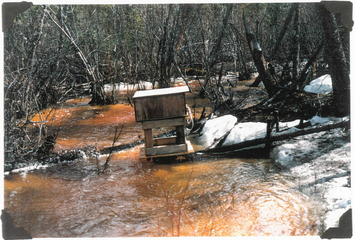
May 2, 1994. Williams Creek Data Logger Station. Extension to instrument housing to permit logger installation. Flow remain on top of channel ice. Ice decreased by 0.4 meters.
