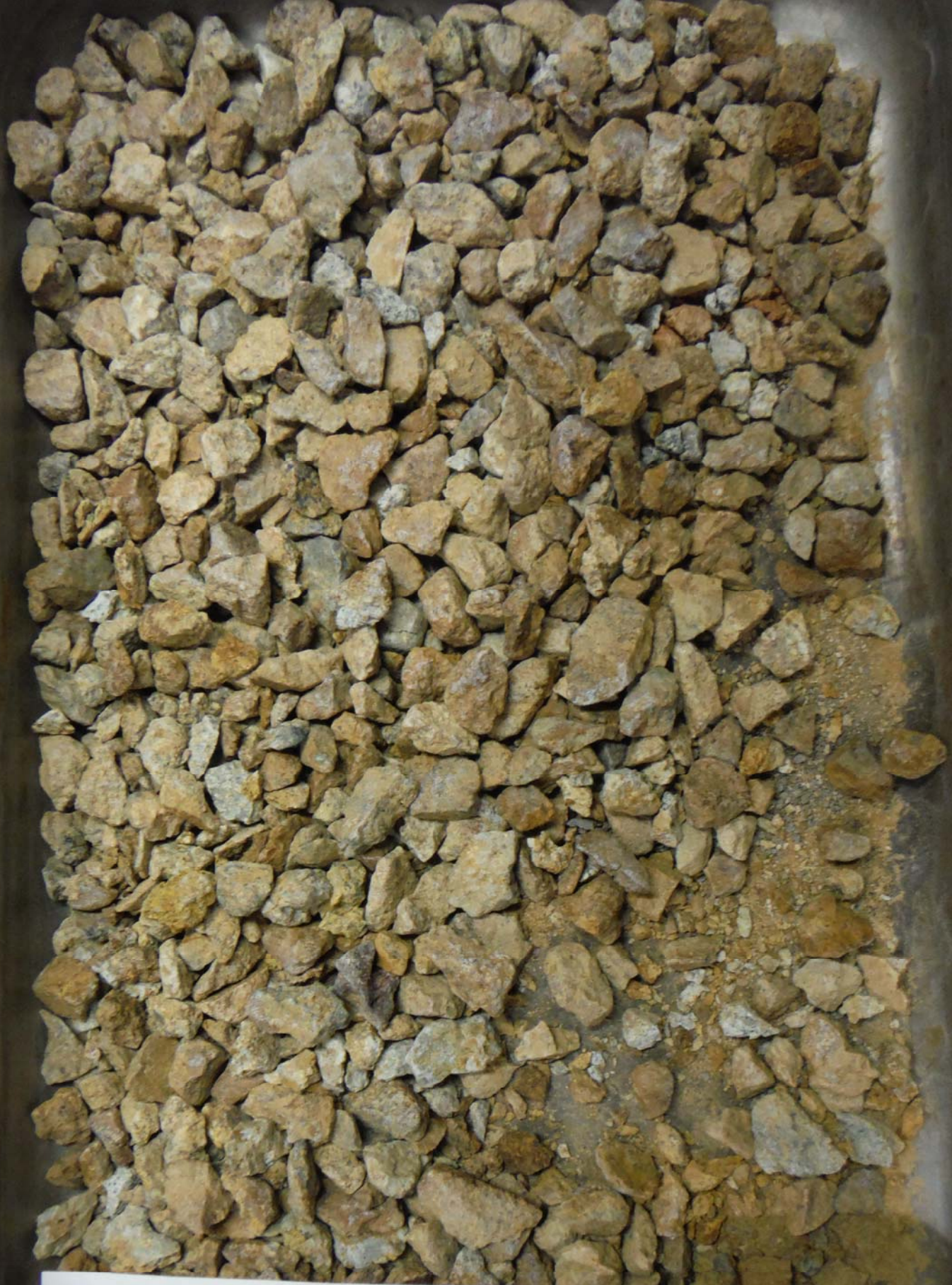
Casino Gold VA101-00325/18 CL-05 No.4 Material Post Freeze-Thaw after 25 Cycles
