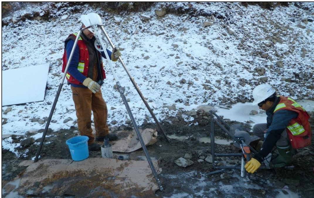
Photograph 1: Bailer-winch system used to develop monitoring wells MW14-03A, MW14-03B, MW14-05A, MW14-05B and MW14-06A. System setup pictured at MW14-06A.
