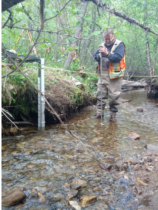
Figure 2-5: Photo showing hydrometric station instrumentation, including metric staff gauge, perforated and screened stilling well and water level recorder.
