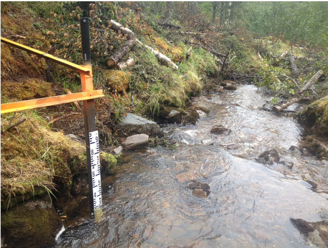
Figure 2-4: T-24-2 Hydrometric station
