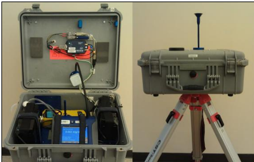
Figure 3-1: DustTrak 8533 installed in an Environmental Enclosure with Inlet
