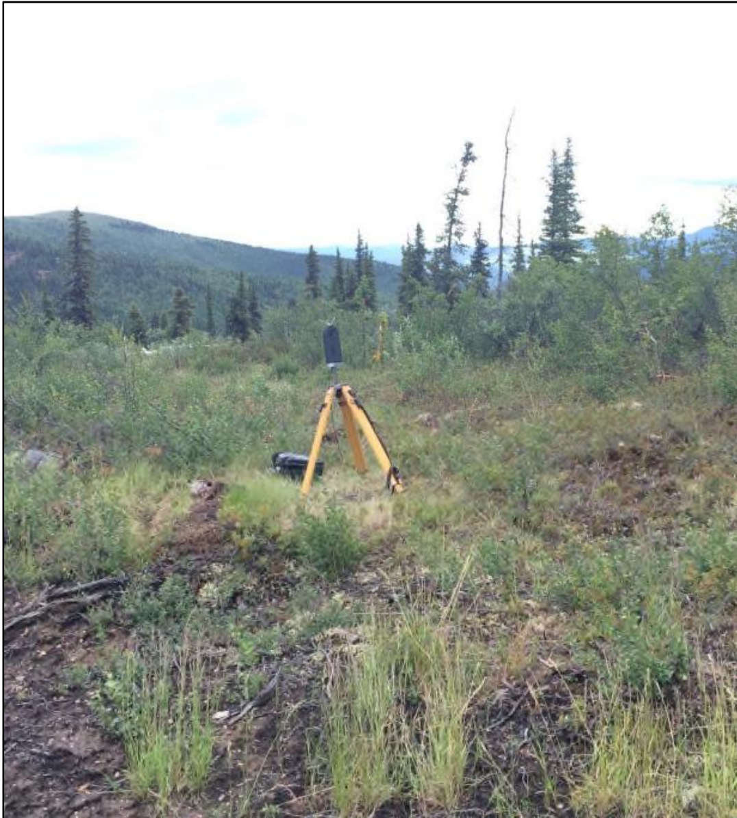
Figure 3-9: Casella Noise Sampler at Station ROM, June 2015
