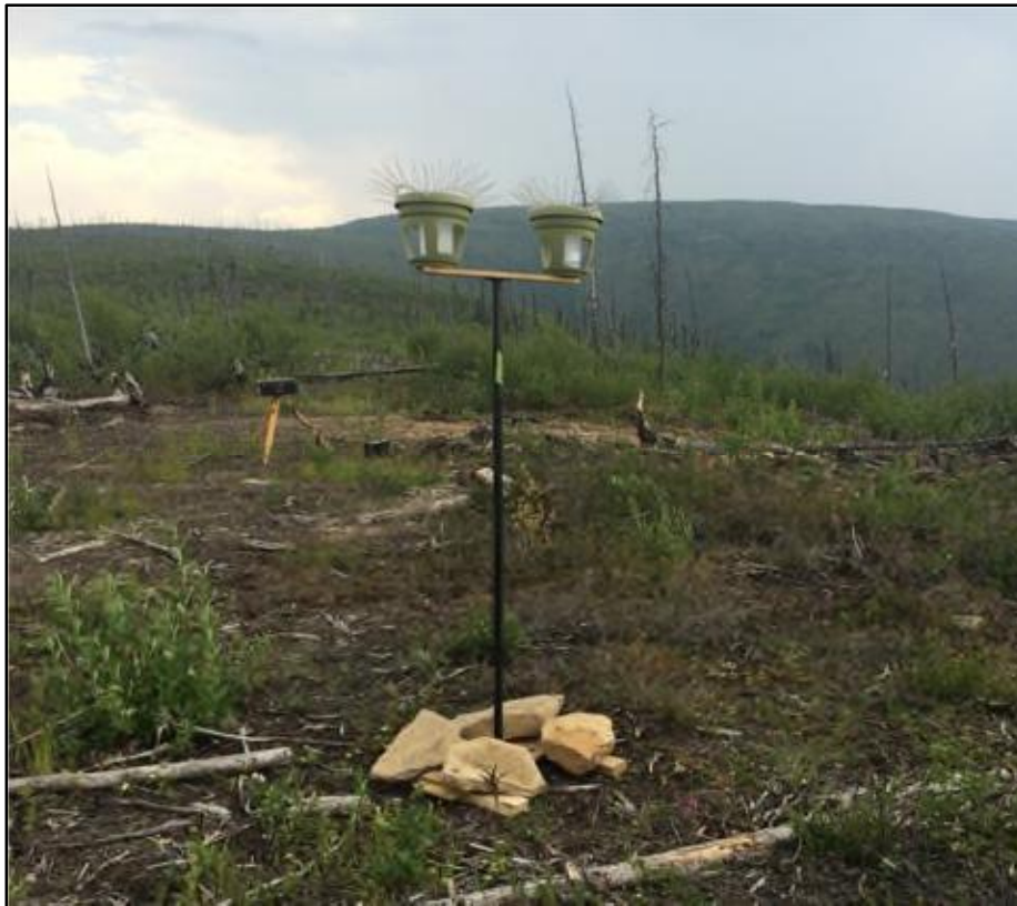
Figure 3-22: Dust Collection Canisters at Monitoring Location H6, June 2015
