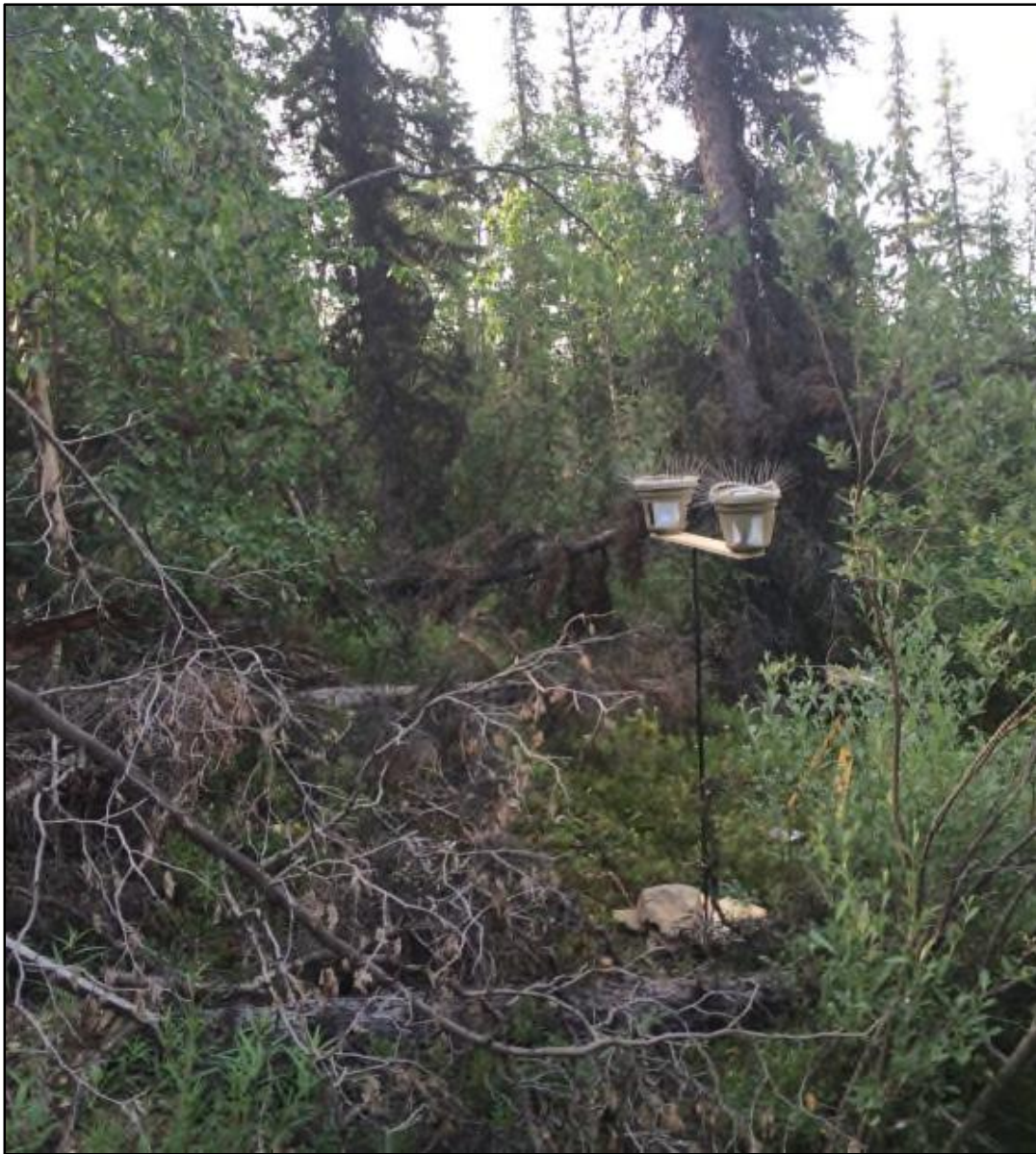
Figure 3-8: Dust Collection Canisters and Air Quality Sampler (behind shrub) at Monitoring Location DD, June 2015
