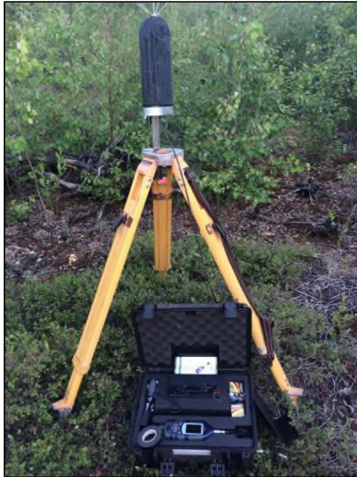
Figure 3-2: Casella CEL-633 Noise Meter installed in an Environmental Enclosure with Microphone and Wind Screen
