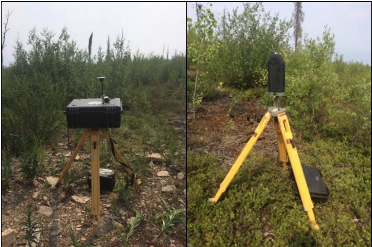
Figure 3-6: Air Quality and Noise Samplers at Monitoring Station MET, June 2015
