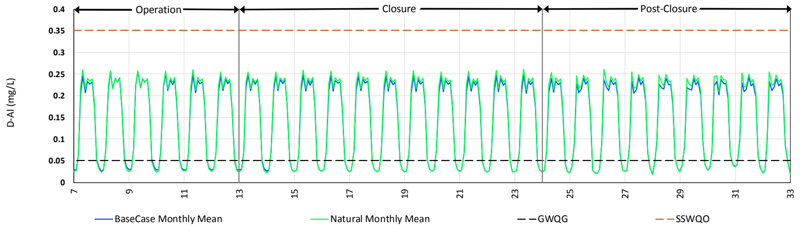
Figure 4.4-2 Dissolved Aluminum Base Case compared to Natural case at CC-3.5 through Operation, Closure, and Post-Closure Mine Phases. GWQG = generic CCME long-term water quality guideline for the protection of freshwater aquatic life. SSWQO = preliminary site-specific water quality objective.
