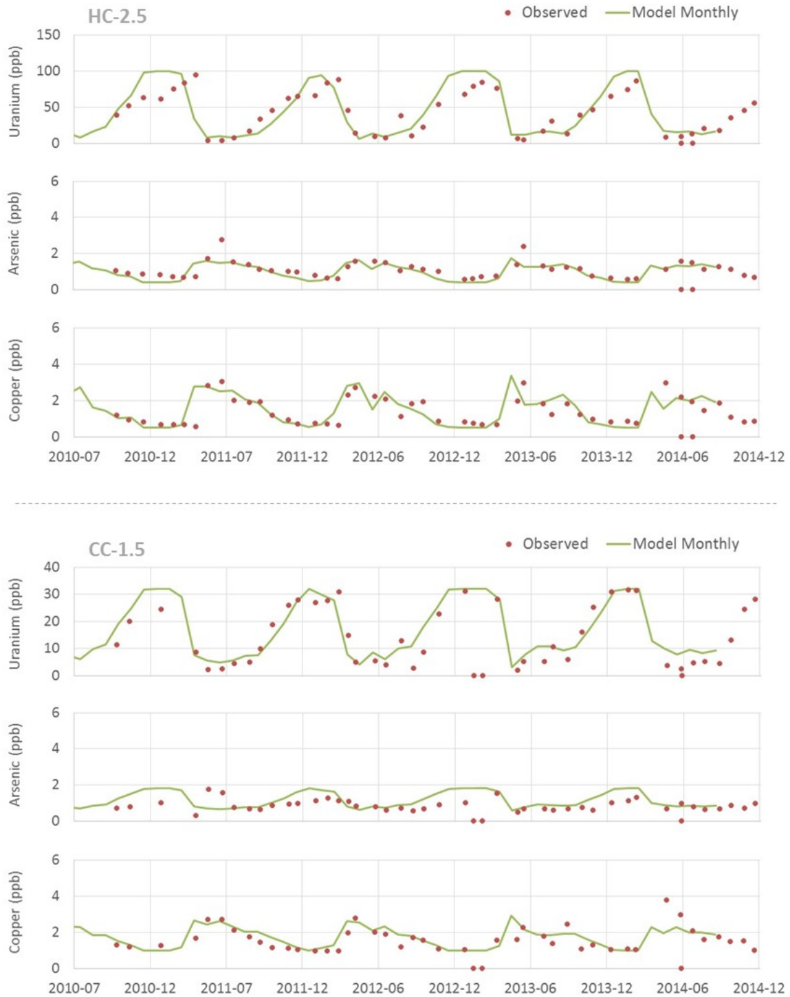
Figure 4-2: Modelled and observed total uranium, total arsenic and total copper concentration ( \mu\text{g/L} ) over the calibration time period. The upper panel presents calibration results for HC-2.5, whereas the lower panel presents calibration results for the CC-1.5 model node.
