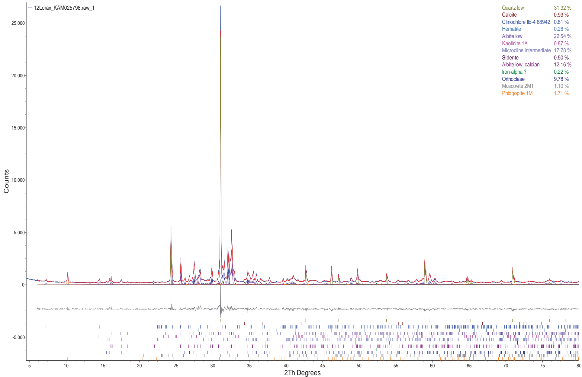
Figure 12. Rietveld refinement plot of sample Lorax Environmental “KAM025798” (blue line - observed intensity at each step; red line - calculated pattern; solid grey line below – difference between observed and calculated intensities; vertical bars - positions of all Bragg reflections). Coloured lines are individual diffraction patterns of all phases.
