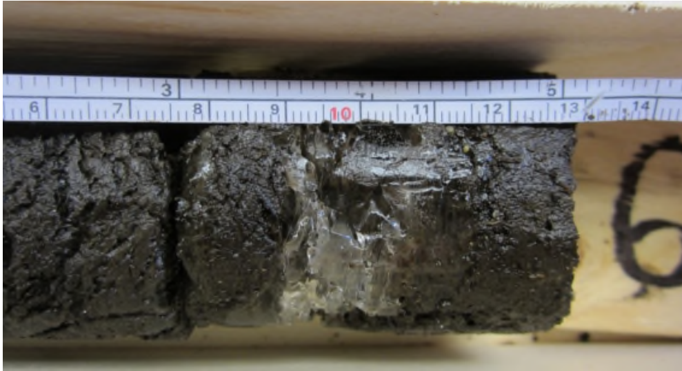
Photo 6: 15 mm thick horizontal ice lens in frozen silt at 5.95 m depth BGL; GT-66, Halfway Pond. Photo taken on September 24, 2016.
