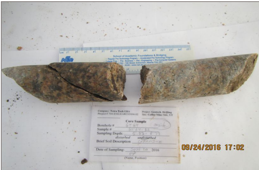
Photo 116E: Tested rock core sample GT64-R2; Depth: 5.53 - 5.73 m; Valid test
