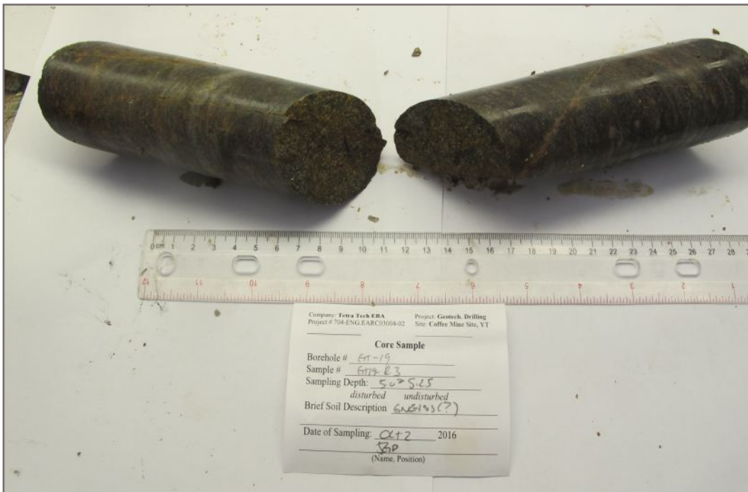
Photo 42E: Tested rock core sample GT19-R3; Depth: 5.00 - 5.25 m; Valid test
