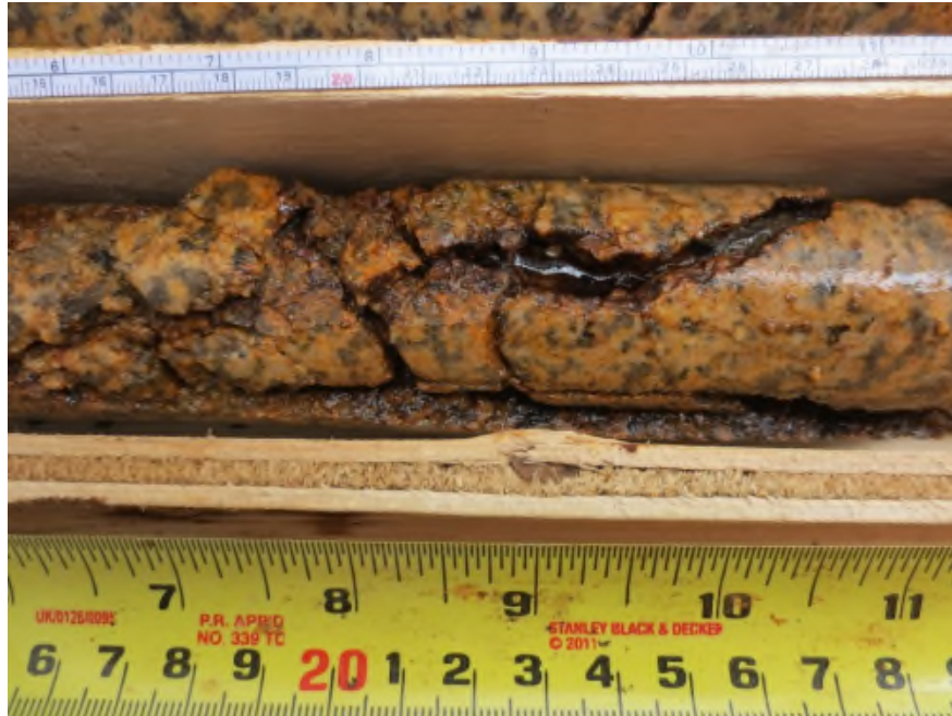
Photo 15: Ground ice infilling a fracture in oxidized granite at 13.7 m depth BGL; GT-47, Kona Pond. Photo taken on September 14, 2016.
