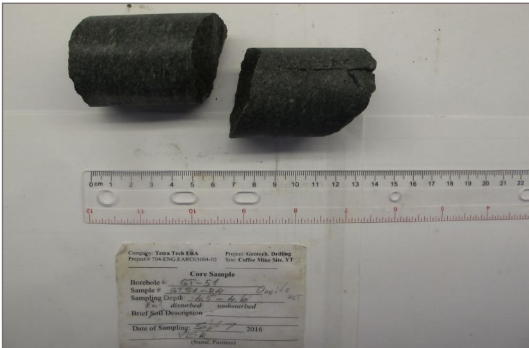
Photo 70E: Tested rock core sample GT51-R4; Depth: 4.50 - 4.60 m; Valid test
