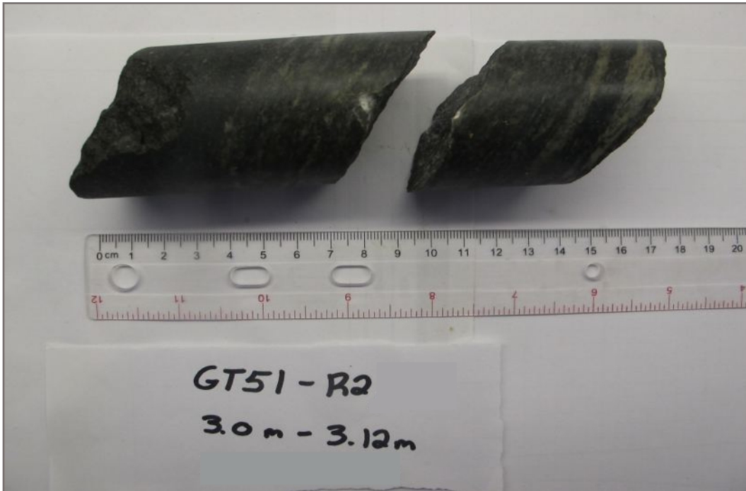
Photo 69E: Tested rock core sample GT51-R2; Depth: 3.00 - 3.12 m; Valid test
