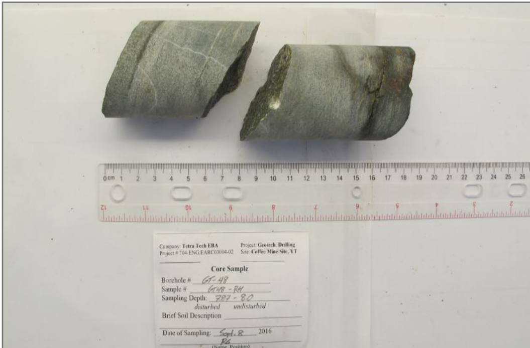
Photo 61E: Tested rock core sample GT48-R4; Depth: 7.87 - 8.00 m; Valid test
