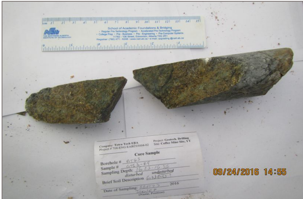
Photo 113E: Tested rock core sample GT63-R9; Depth: 16.23 - 16.35 m; Invalid test
