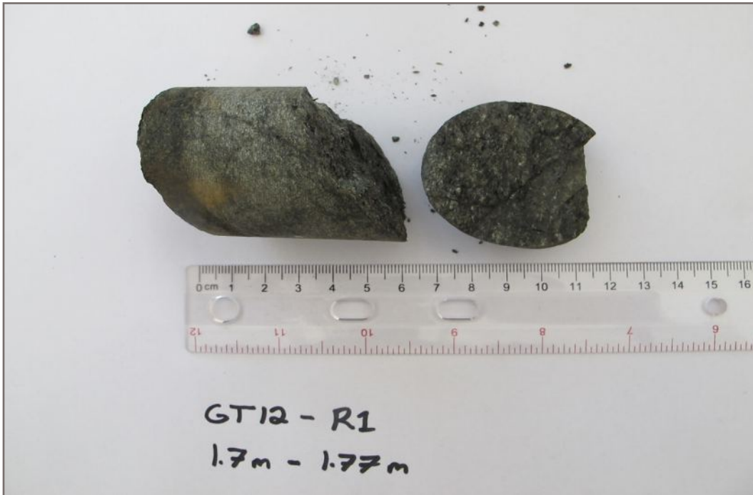
Photo 13E: Tested rock core sample GT12-R1; Depth: 1.70 - 1.77 m; Invalid test
