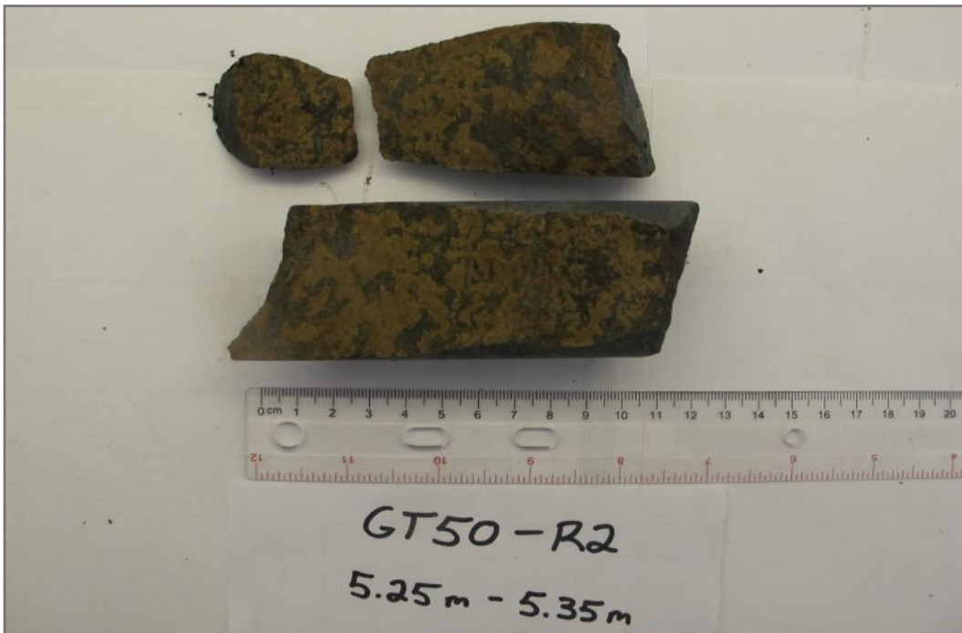
Photo 64E: Tested rock core sample GT50-R2; Depth: 5.25 - 5.35 m; Invalid test
