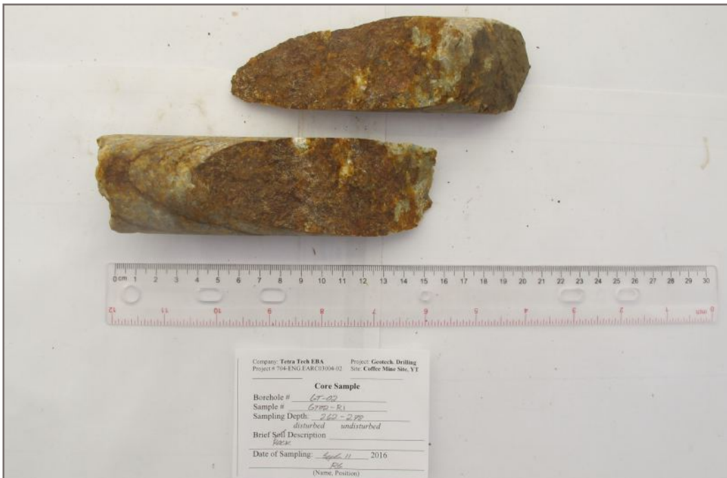
Photo 4E: Tested rock core sample GT02-R1; Depth: 2.62 - 2.78 m; Valid test
