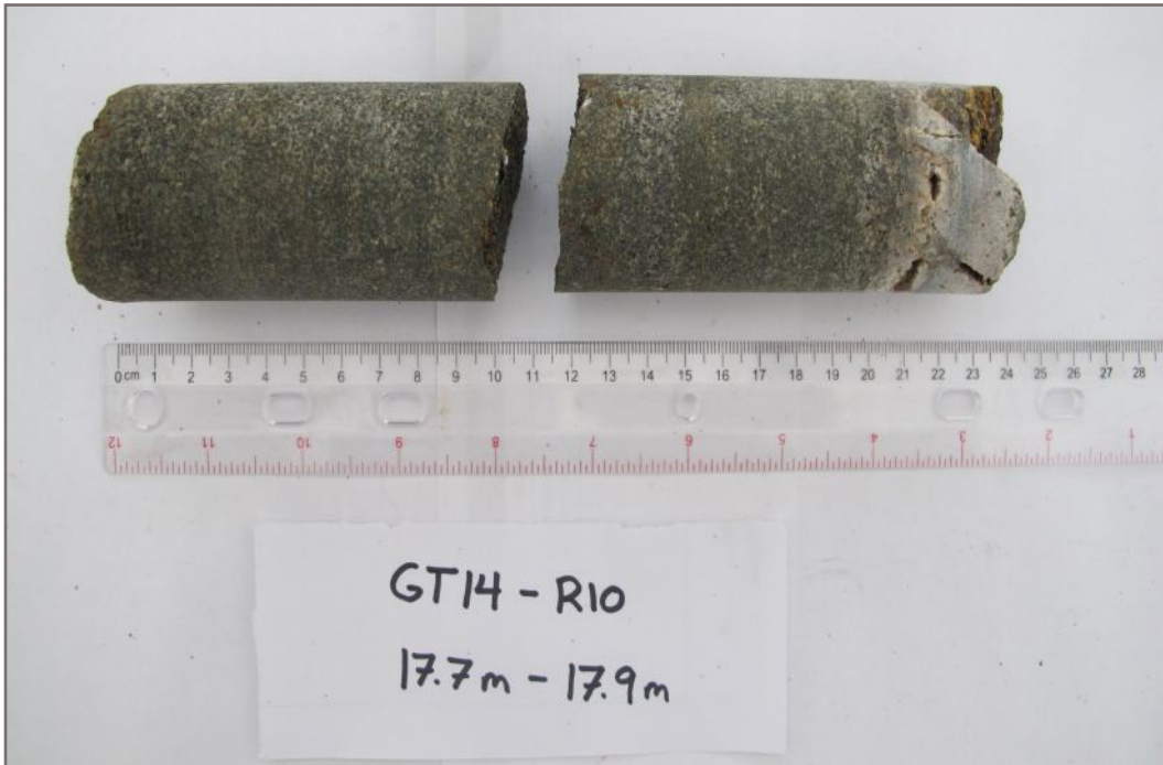
Photo 27E: Tested rock core sample GT14-R10; Depth: 17.70 - 17.90 m; Valid test
