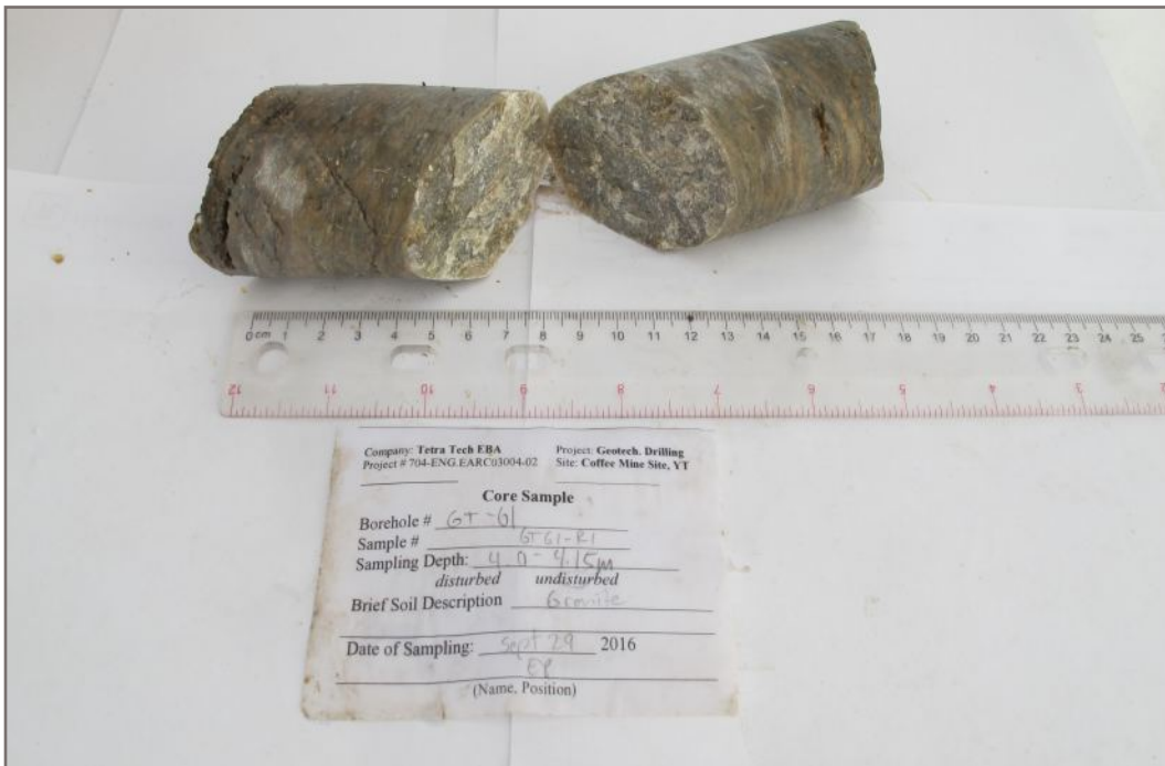
Photo 100E: Tested rock core sample GT61-R1; Depth: 4.00 - 4.15 m; Valid test
