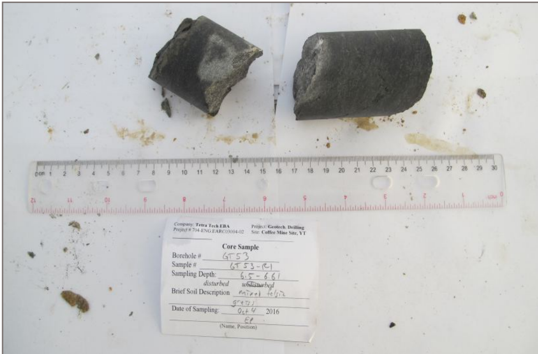
Photo 81E: Tested rock core sample GT53-R1; Depth: 6.50 - 6.61 m; Valid test
