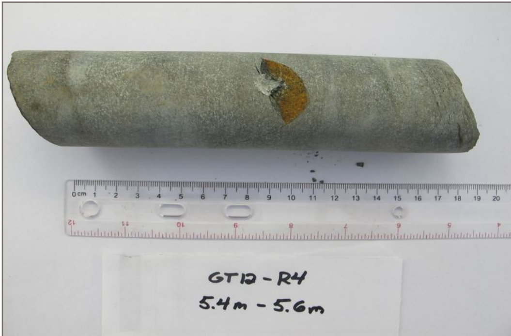
Photo 15E: Tested rock core sample GT12-R4; Depth: 5.40 - 5.60 m; Invalid test
