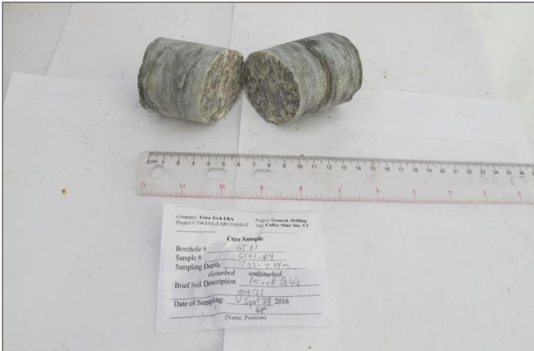
Photo 103E: Tested rock core sample GT61-R4; Depth: 7.33 - 7.44 m; Valid test
