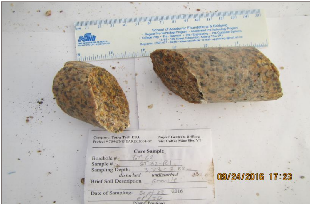
Photo 104E: Tested rock core sample GT62-R1; Depth: 3.73 - 3.82 m; Valid test
