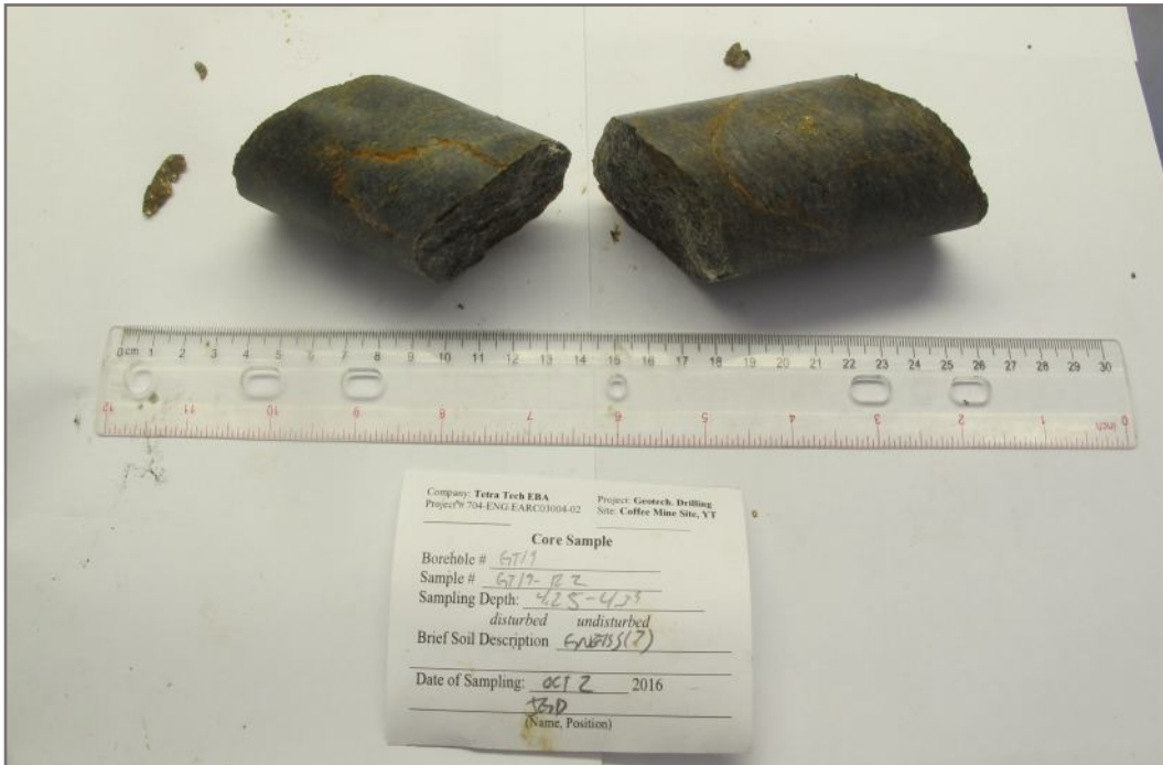
Photo 41E: Tested rock core sample GT19-R2; Depth: 4.25 - 4.39 m; Valid test
