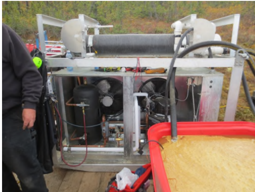
Photo 3: Drilling fluid refrigeration unit (chiller) with a mixing tank filled with Perma-Drill ES mixed with water.
