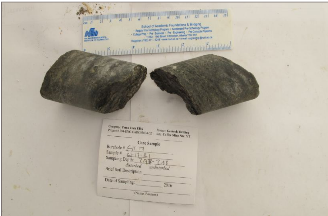
Photo 36E: Tested rock core sample GT17-R1; Depth: 2.72 - 2.88 m; Invalid test
