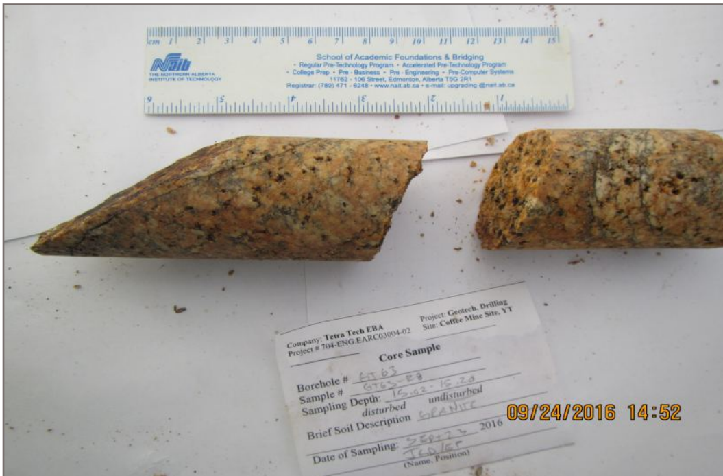
Photo 112E: Tested rock core sample GT63-R8; Depth: 15.02 - 15.20 m; Valid test
