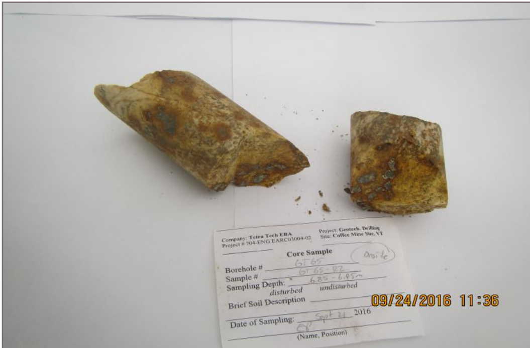
Photo 119E: Tested rock core sample GT65-R2; Depth: 6.85 - 6.95 m; Valid test
