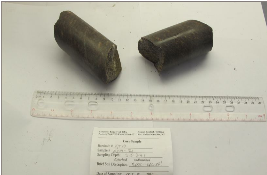
Photo 40E: Tested rock core sample GT19-R1; Depth: 3.50 - 3.71 m; Valid test
