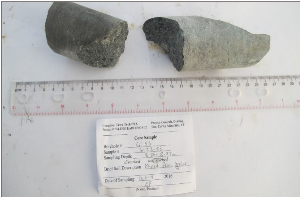
Photo 83E: Tested rock core sample GT53-R3; Depth: 8.86 - 8.97 m; Valid test
