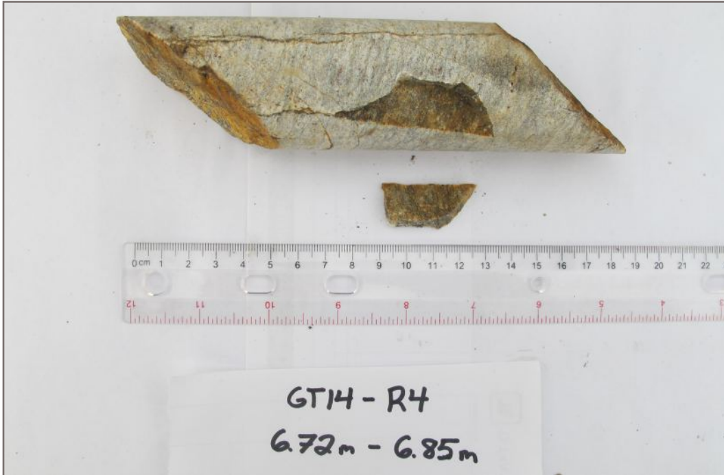
Photo 21E: Tested rock core sample GT14-R4; Depth: 6.72 - 6.85 m; Invalid test
