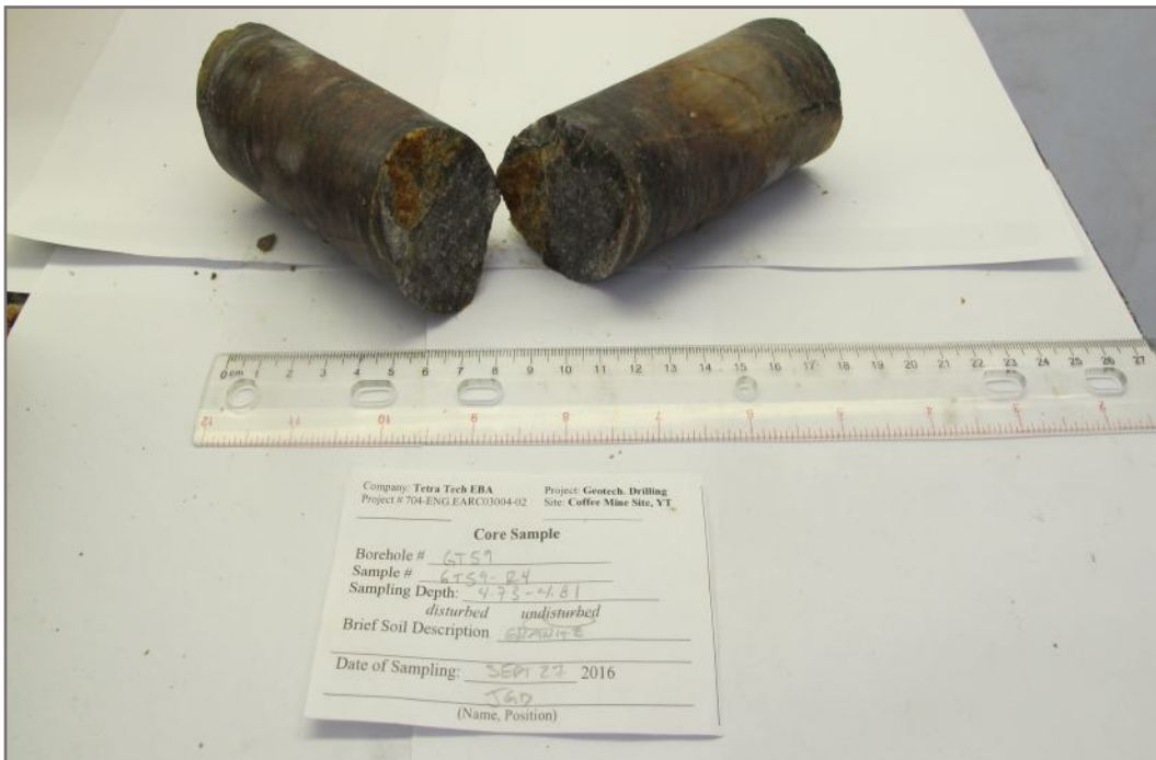
Photo 96E: Tested rock core sample GT59-R4; Depth: 4.73 - 4.81 m; Valid test
