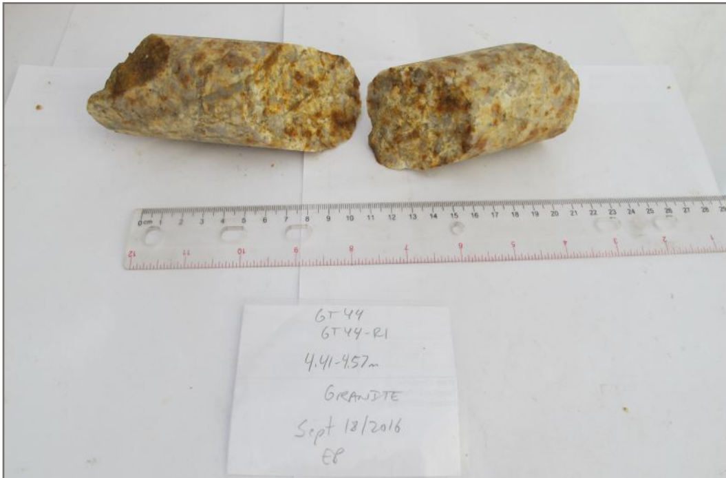
Photo 47E: Tested rock core sample GT44-R1; Depth: 4.41 - 4.57 m; Valid test
