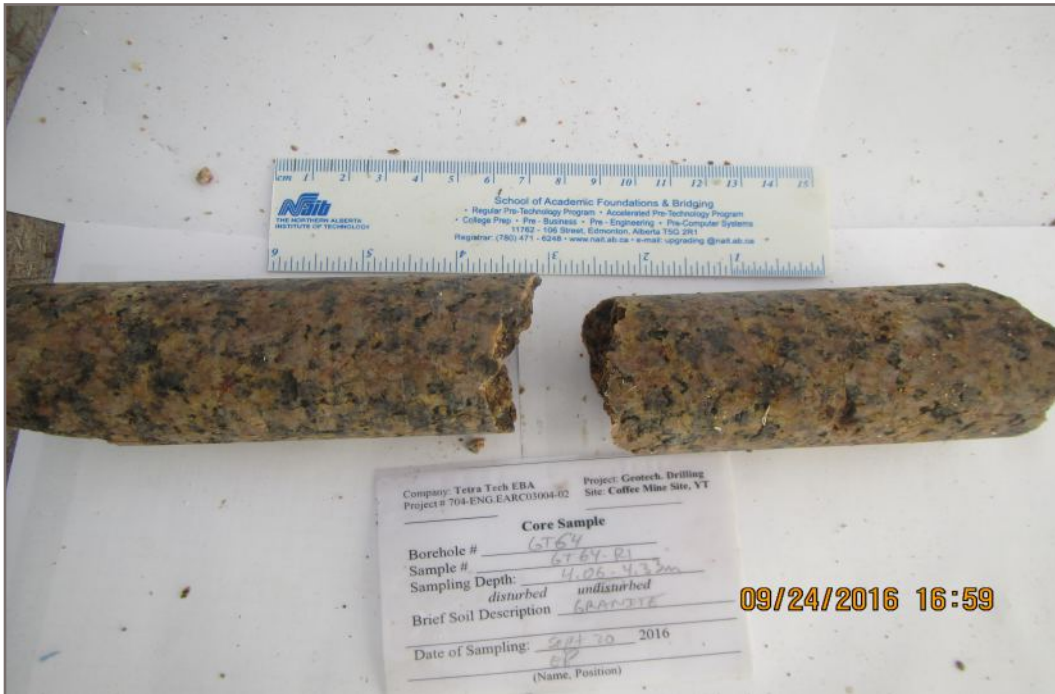
Photo 115E: Tested rock core sample GT64-R1; Depth: 4.06 - 4.33 m; Valid test
