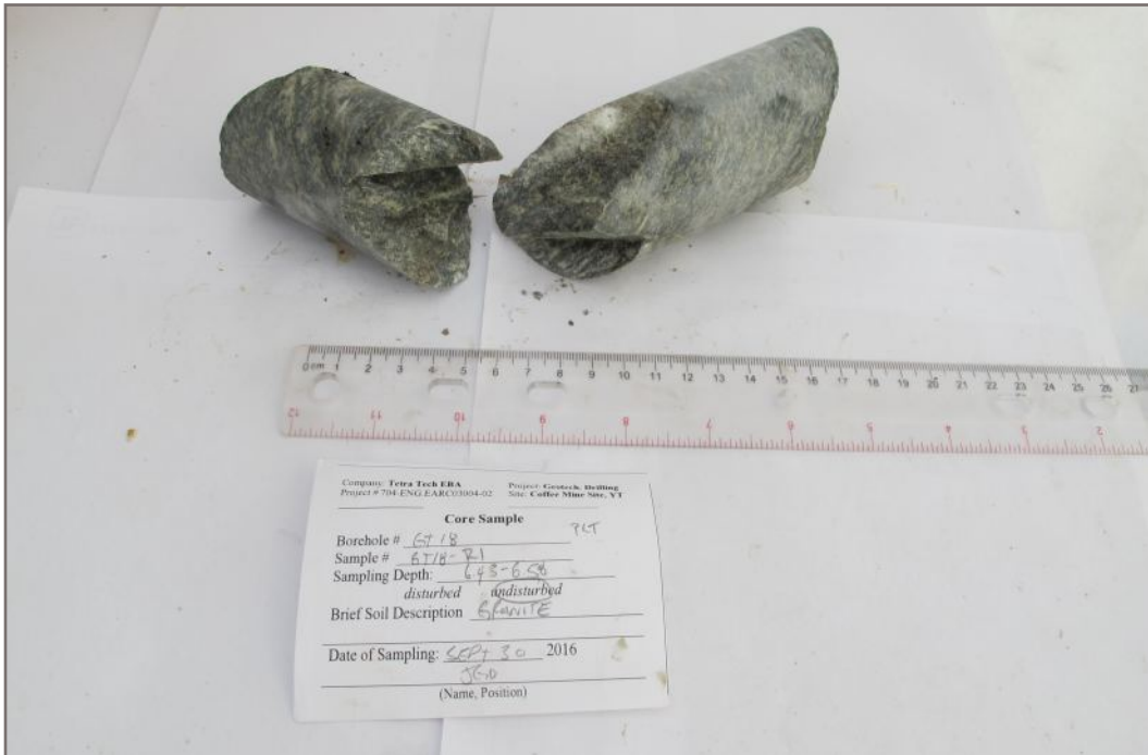
Photo 39E: Tested rock core sample GT18-R1; Depth: 6.43 - 6.58 m; Valid test
