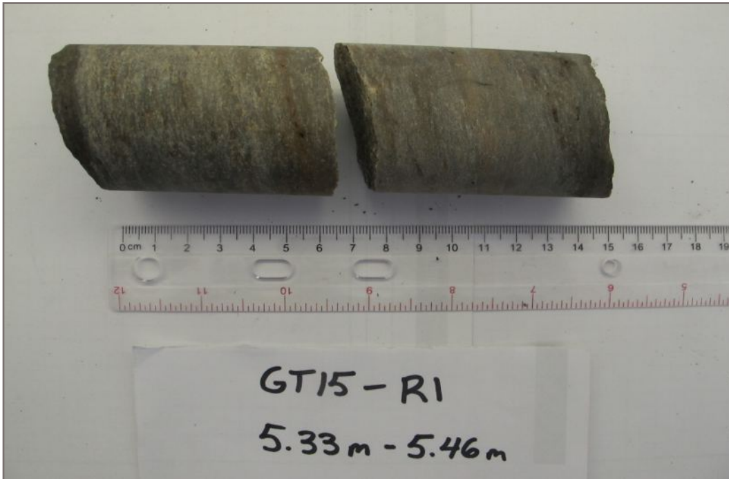
Photo 29E: Tested rock core sample GT15-R1; Depth: 5.33 - 5.46 m; Valid test
