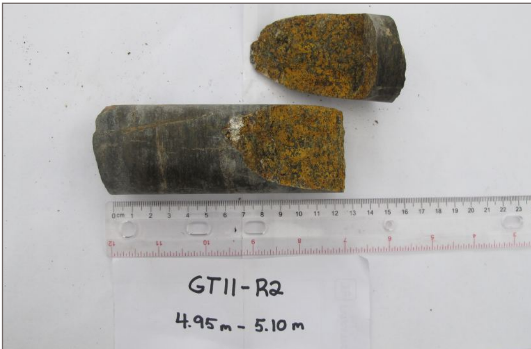
Photo 12E: Tested rock core sample GT11-R2; Depth: 4.95 - 5.10 m; Invalid test
