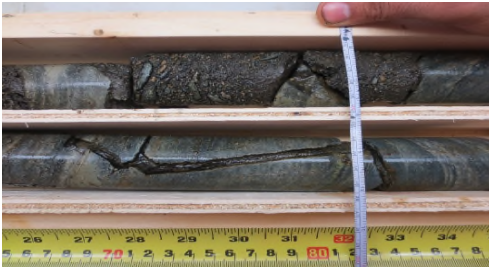
Photo 7: Ice infilling vertical fracture in gneiss bedrock at 2.65 m depth BGL; GT-51, North Pond. Photo taken on September 6, 2016.
