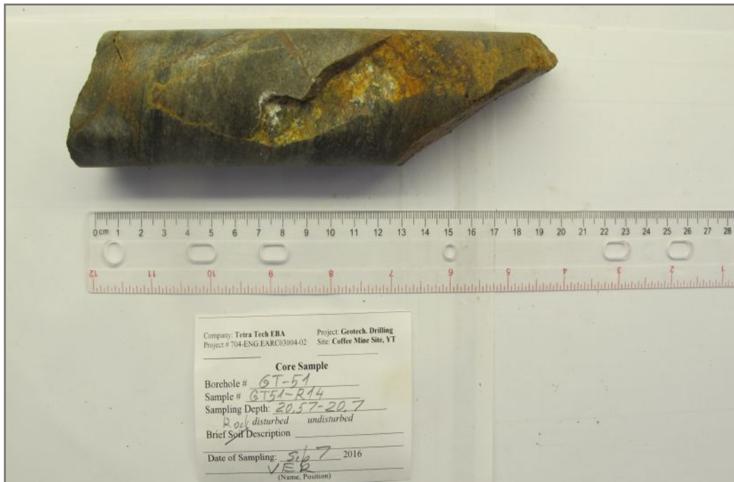
Photo 80E: Tested rock core sample GT51-R14; Depth: 20.57 - 20.70 m; Invalid test
