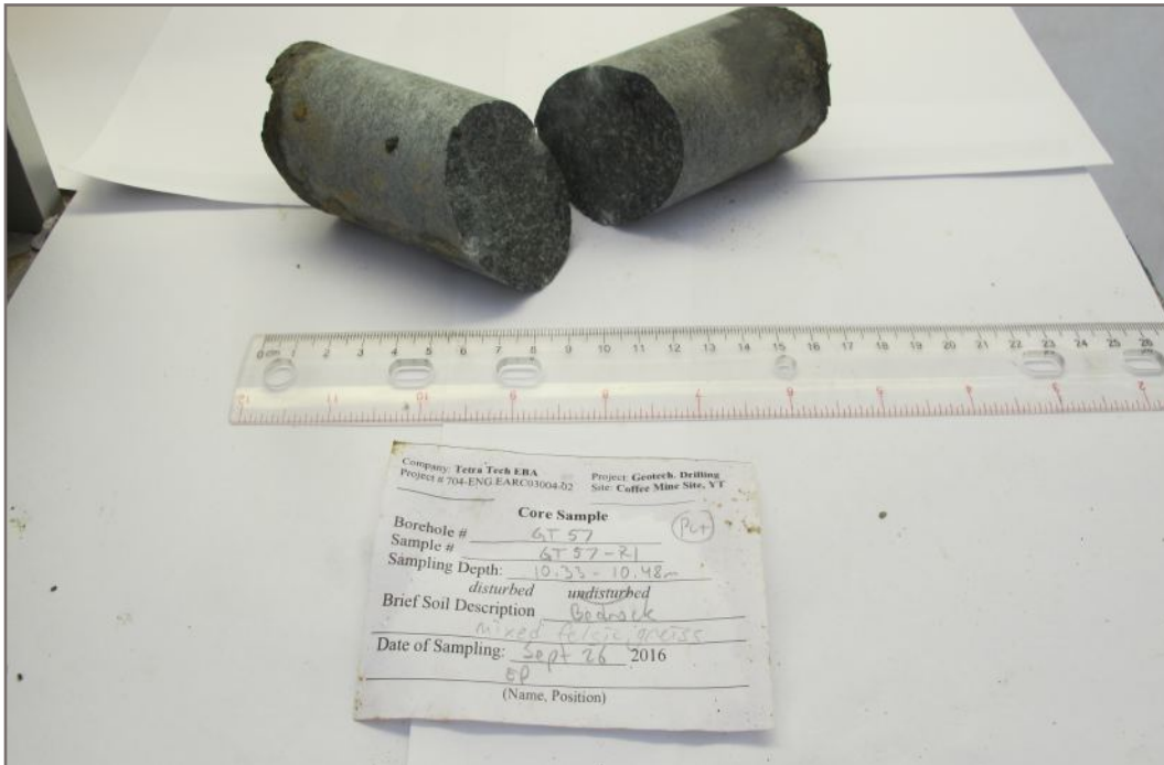
Photo 87E: Tested rock core sample GT57-R1; Depth: 10.33 - 10.48 m; Valid test
