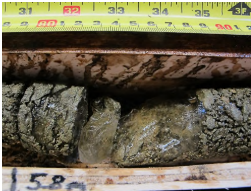
Photo 25: Ice lenses (Vs) and inclusions (Vx) in frozen sand with some gravel and silt at a depth of 5.8 m BGL in Borehole GT-15, North WRSF. Photo taken on September 4, 2016.
