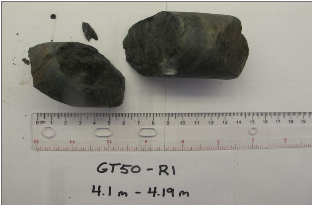
Photo 63E: Tested rock core sample GT50-R1; Depth: 4.10 - 4.19 m; Invalid test
