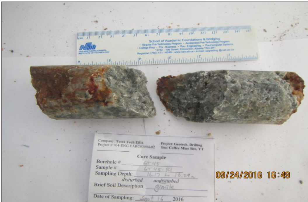
Photo 48E: Tested rock core sample GT45-R1; Depth: 16.17 - 16.29 m; Valid test
