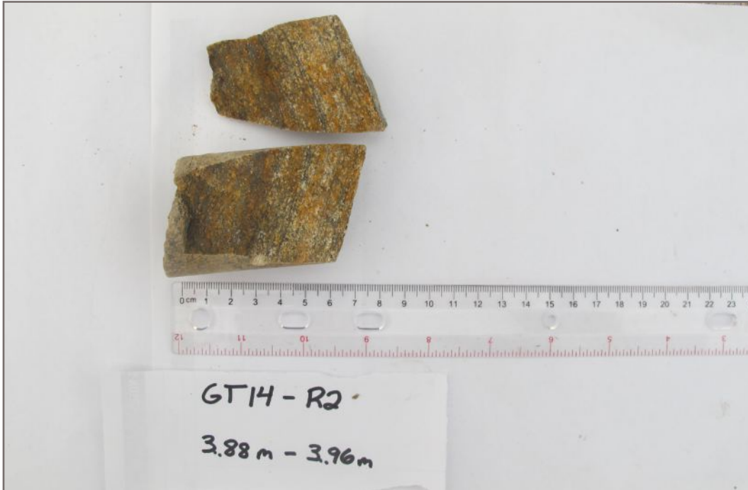
Photo 19E: Tested rock core sample GT14-R2; Depth: 3.88 - 3.96 m; Valid test
