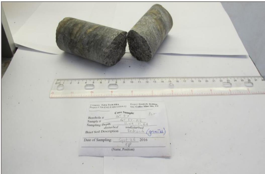
Photo 88E: Tested rock core sample GT57-R2; Depth: 11.49 - 11.66 m; Valid test
