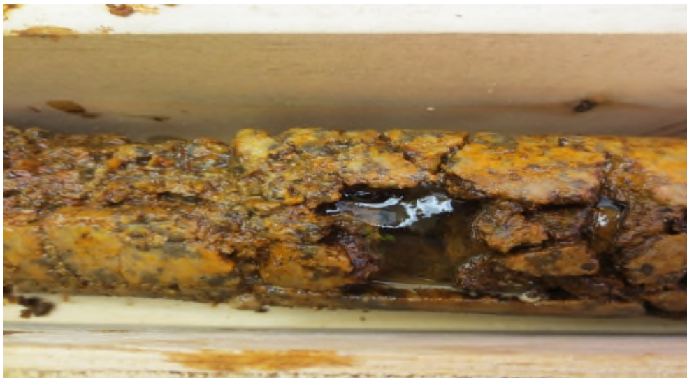
Photo 8: Ice inclusion (Vx) in fractured upper bedrock at 13.2 m depth BGL; GT-47, Kona Pond. Photo taken on September 14, 2016.
