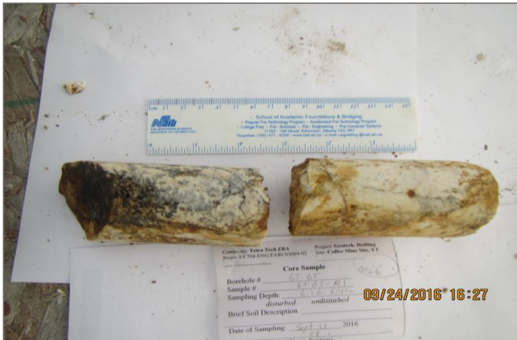
Photo 118E: Tested rock core sample GT65-R1; Depth: 6.26 - 6.41 m; Valid test
