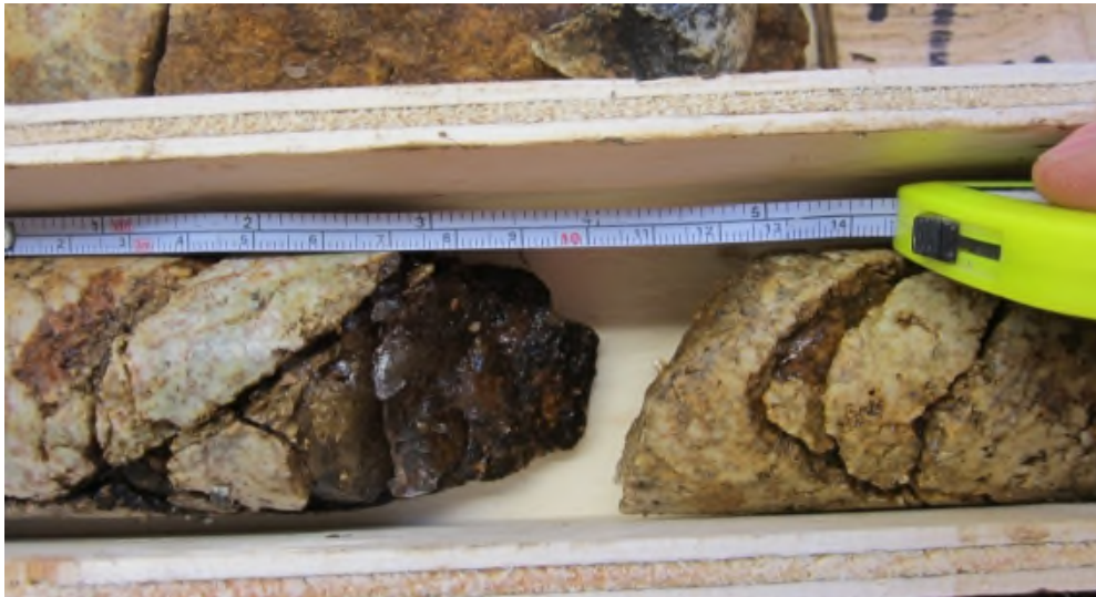
Photo 19: Ground ice infilling joints in granite at 7.9 m depth BGL; GT-65, Halfway Pond. Photo taken on September 21, 2016.
