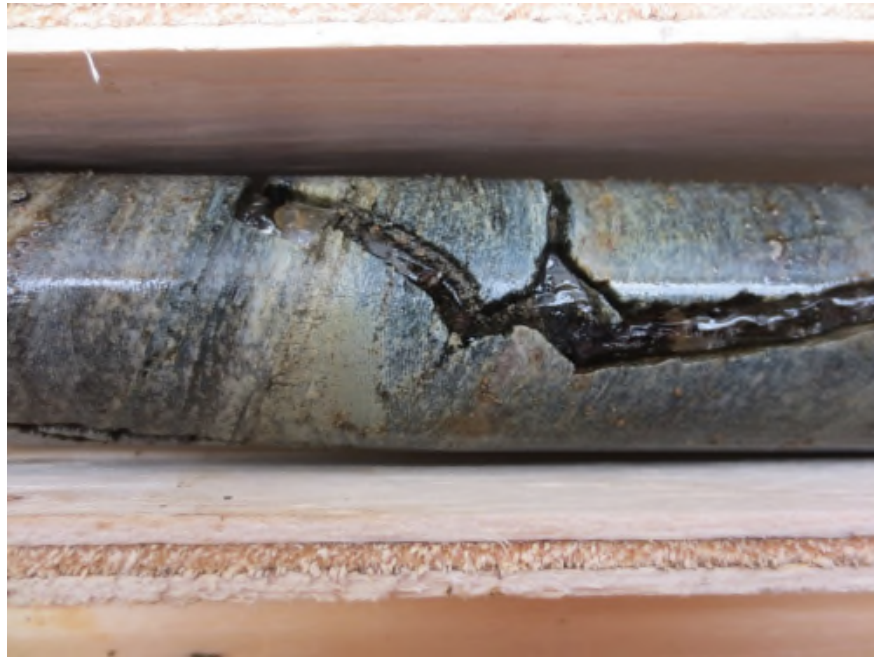
Photo 30: Ice infilling subvertical fracture in gneiss at a depth of 2.7 m BGL in GT-51, North Pond. Photo taken in September 6, 2016.
