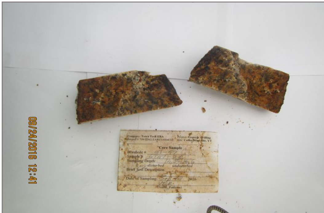
Photo 54E: Tested rock core sample GT47-R1; Depth: 14.50 - 14.60 m; Valid test
