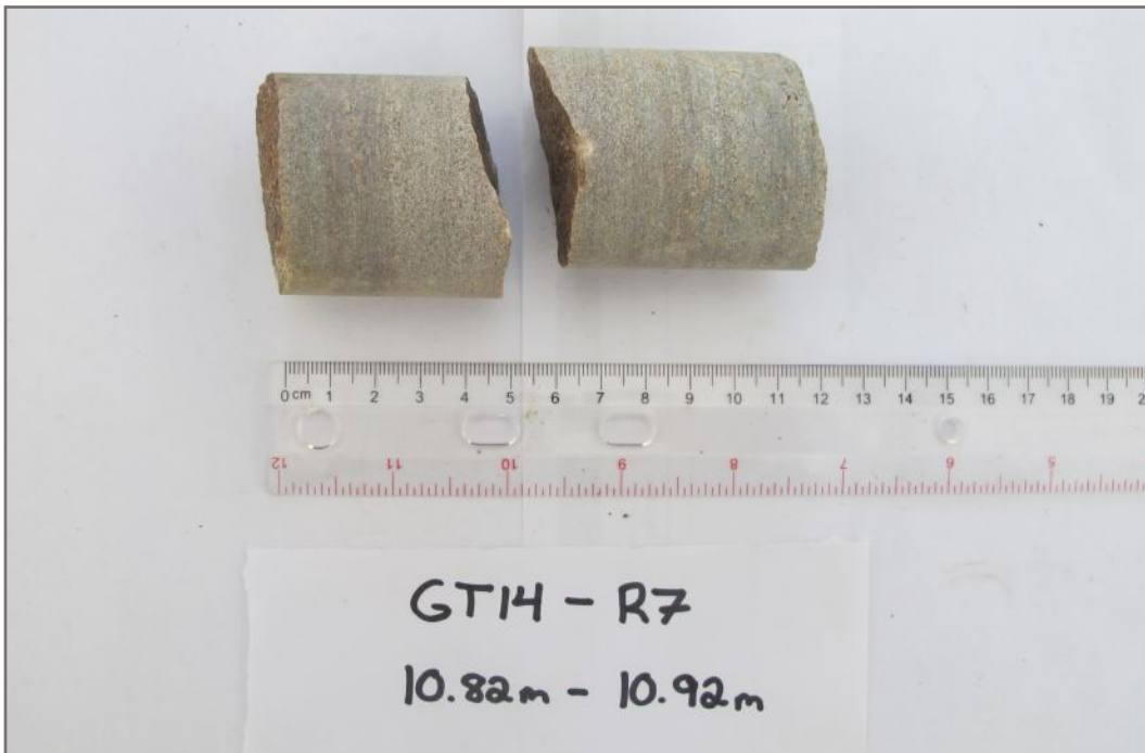
Photo 24E: Tested rock core sample GT14-R7; Depth: 10.82 - 10.92 m; Valid test
