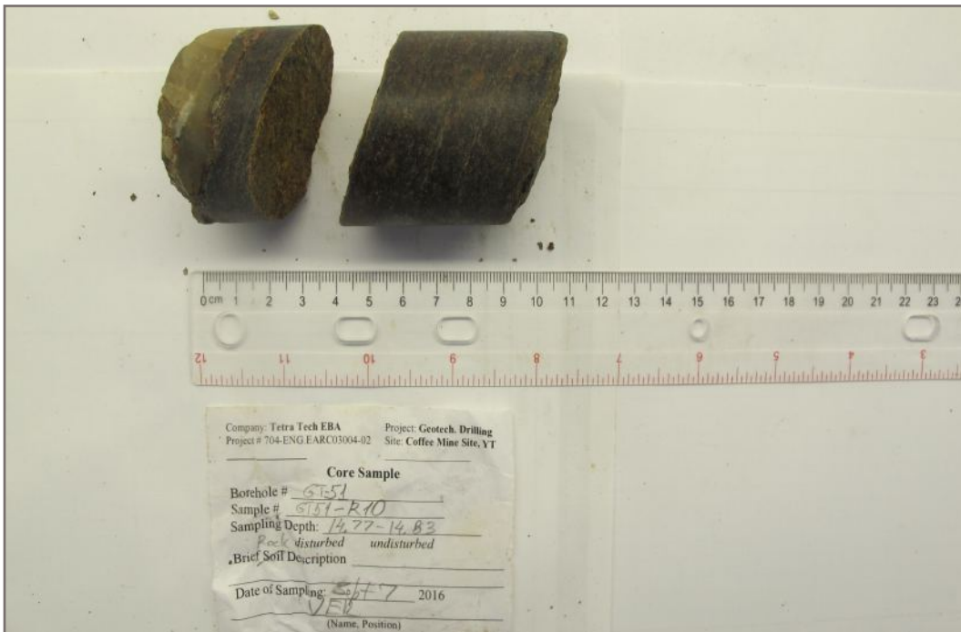
Photo 76E: Tested rock core sample GT51-R10; Depth: 14.77 - 14.83 m; Invalid test
