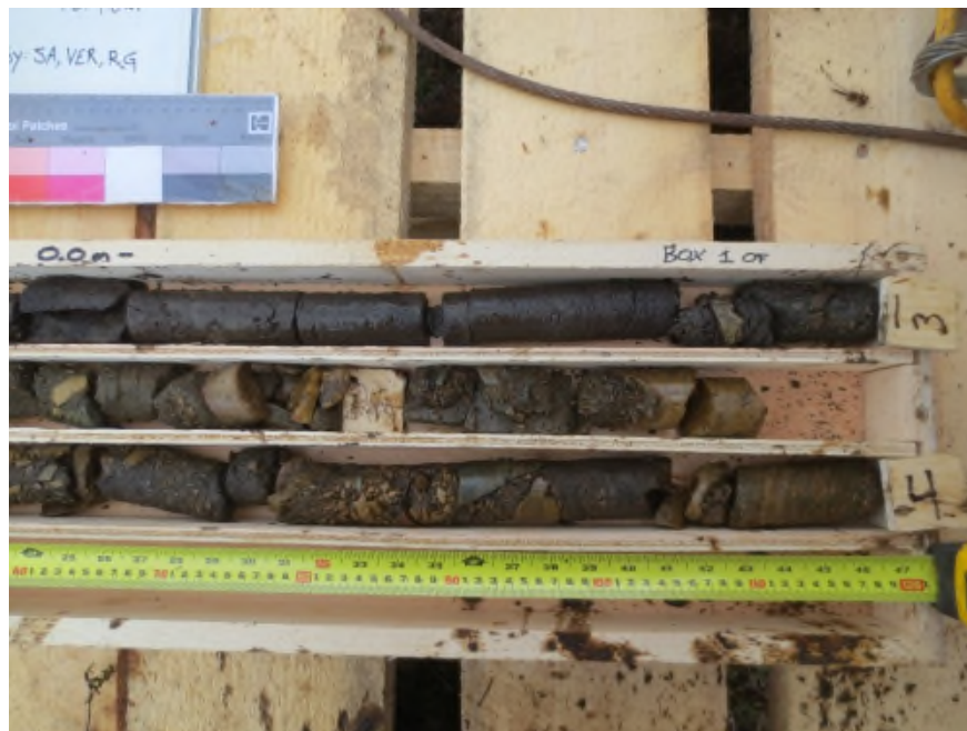
Photo 5: Good quality intact frozen overburden core recovered with chilled Perma-Drill SE drilling fluid in Borehole GT-10 (0.3 m to 4.0 m depth interval). Photo taken on September 1, 2016.
