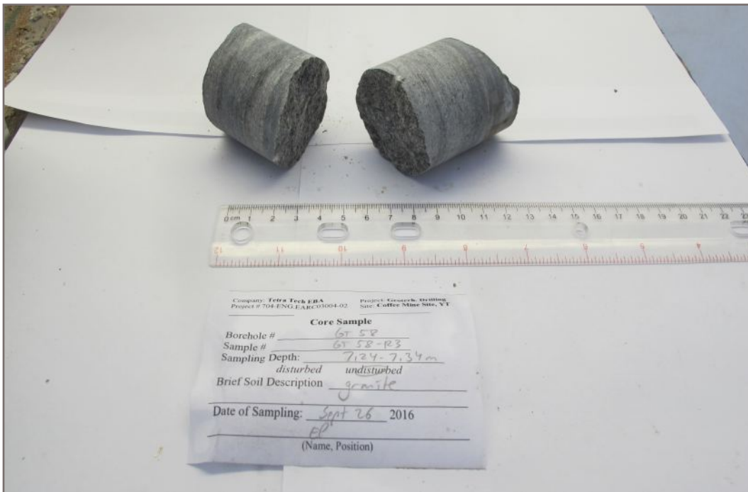
Photo 92E: Tested rock core sample GT58-R3; Depth: 7.24 - 7.34 m; Valid test
