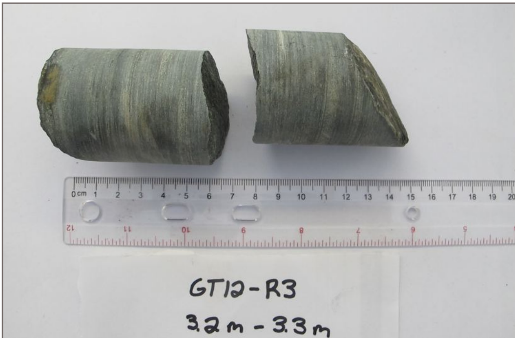
Photo 14E: Tested rock core sample GT12-R3; Depth: 3.20 - 3.30 m; Valid test
