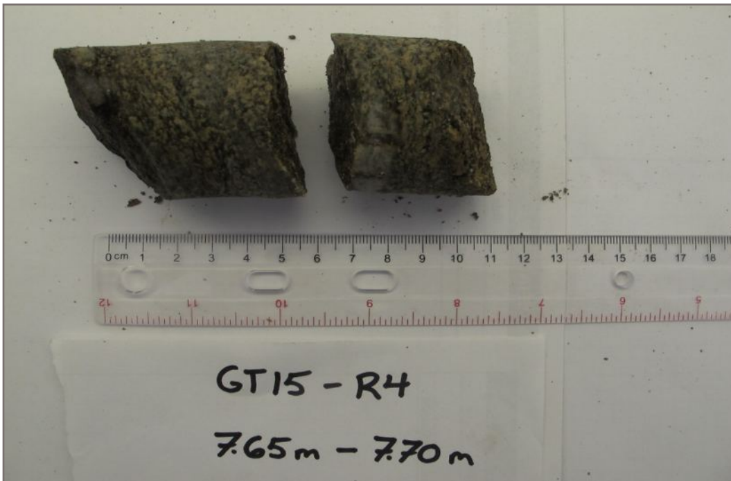
Photo 32E: Tested rock core sample GT15-R4; Depth: 7.65 - 7.70 m; Invalid test
