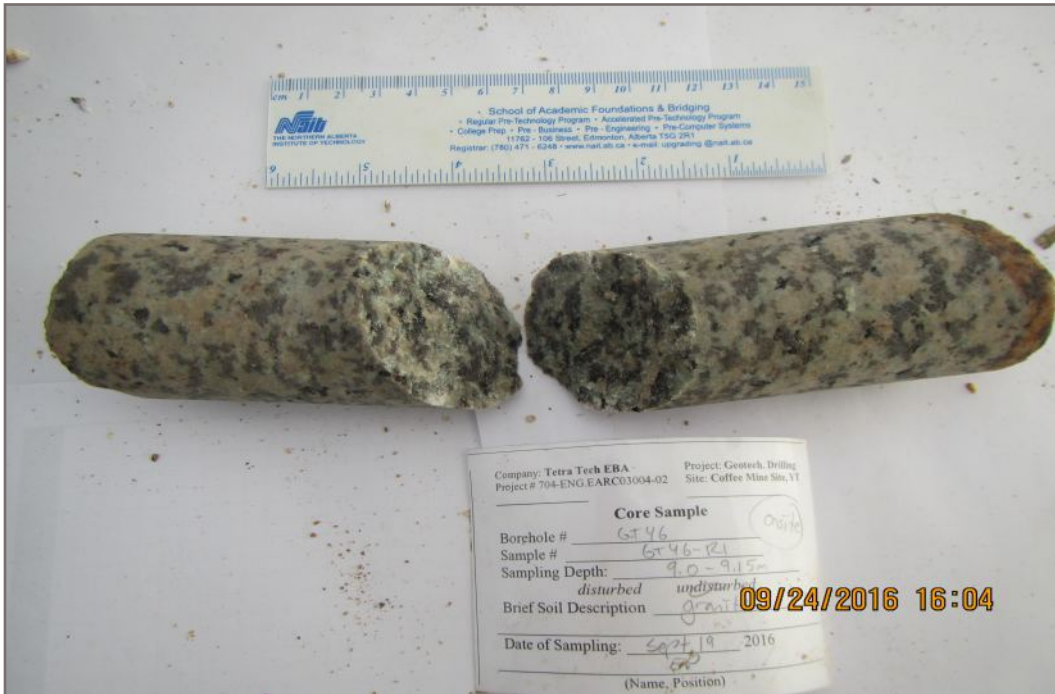
Photo 51E: Tested rock core sample GT46-R1; Depth: 9.00 - 9.15 m; Valid test
