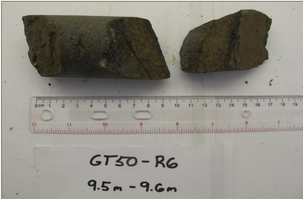
Photo 67E: Tested rock core sample GT50-R6; Depth: 9.50 - 9.60 m; Invalid test
