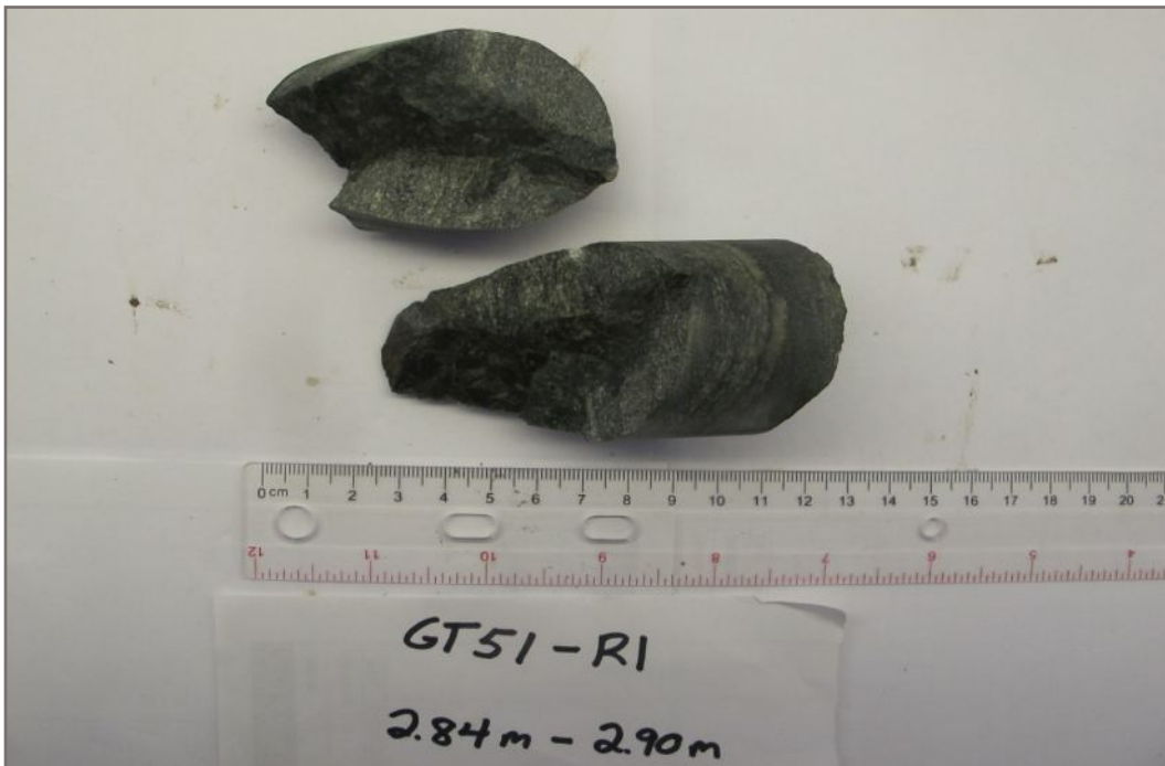
Photo 68E: Tested rock core sample GT51-R1; Depth: 2.84 - 2.90 m; Valid test
