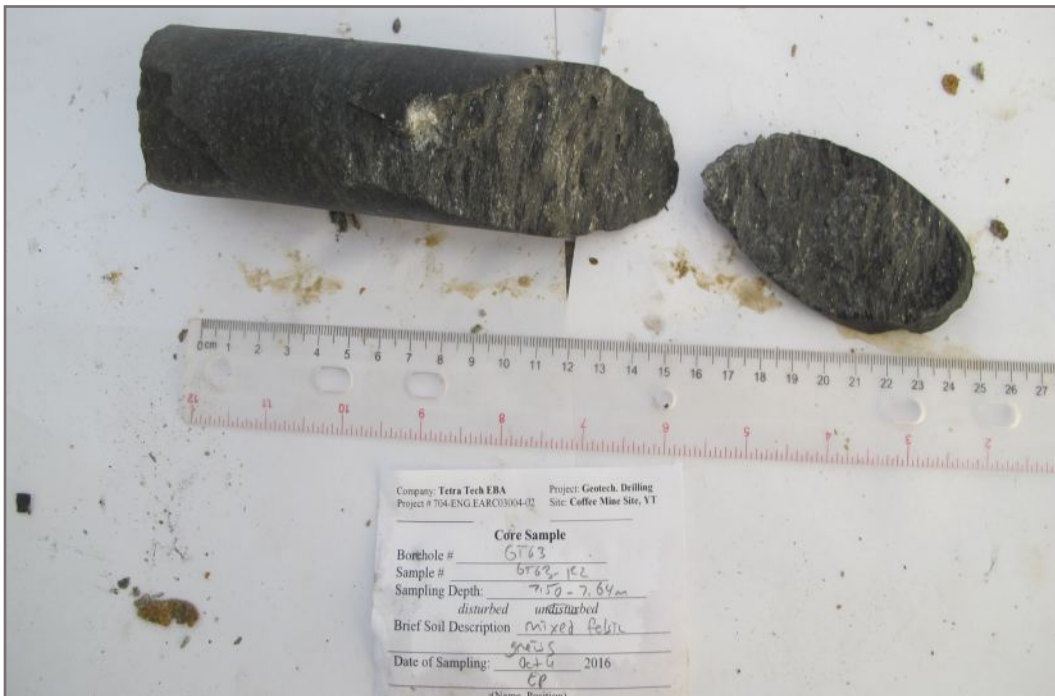
Photo 82E: Tested rock core sample GT53-R2; Depth: 7.50 - 7.64 m; Invalid test
