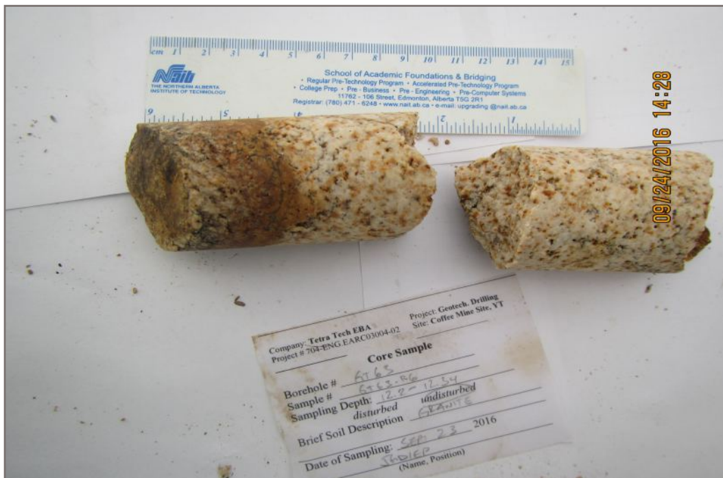
Photo 110E: Tested rock core sample GT63-R6; Depth: 12.20 - 12.34 m; Invalid test
