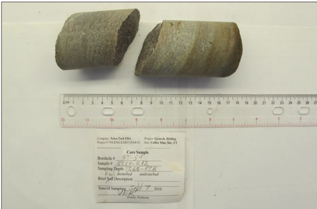
Photo 78E: Tested rock core sample GT51-R12; Depth: 17.68 - 17.80 m; Invalid test
