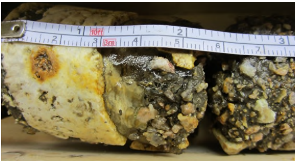
Photo 18: Ice inclusion (Vx) in frozen sand and gravel at 5.1 m depth BGL, GT-65, Halfway Pond. Photo taken on September 21, 2016.
