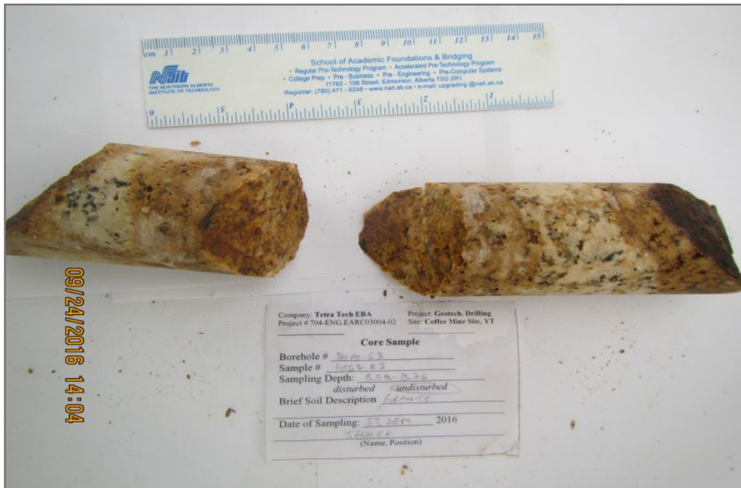
Photo 108E: Tested rock core sample GT63-R3; Depth: 8.85 - 8.76 m; Valid test
