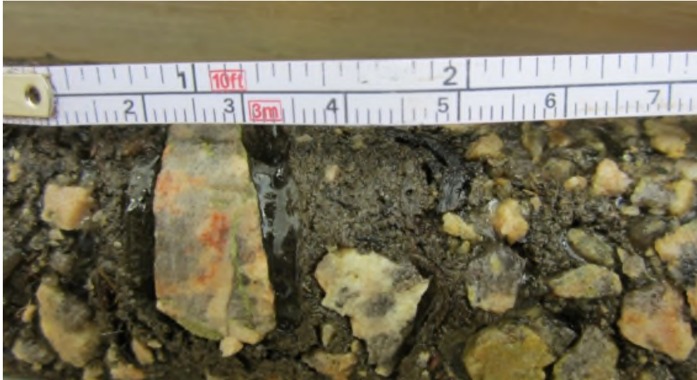
Photo 17: Ice coating on a piece of gravel at 2.8 m depth BGL, GT-65, Halfway Pond. Photo taken on September 21, 2016.
