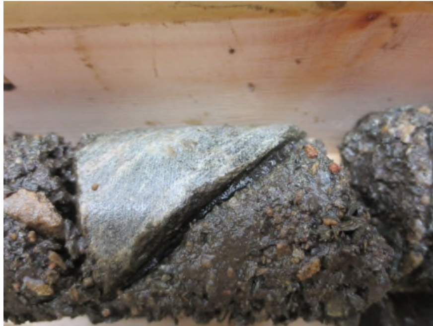
Photo 29: Ice coating on gravel (Vc) in silty sand with a trace of gravel at a depth of approximately 1.5 m BGL in Borehole GT-51, North Pond. Photo taken on September 6, 2016.
