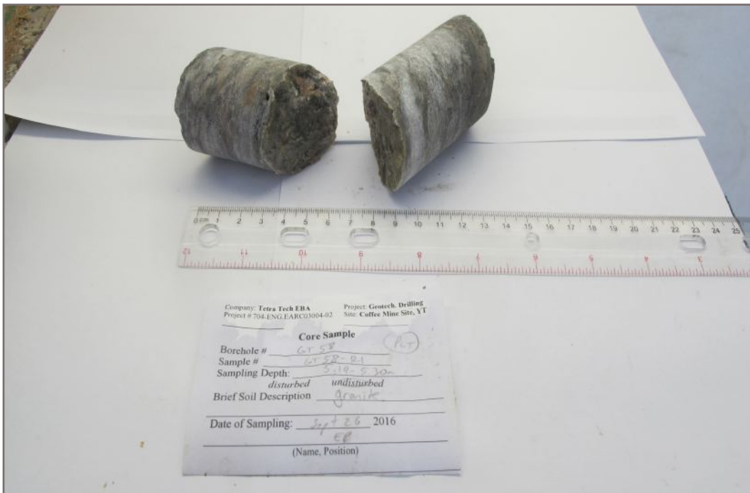
Photo 90E: Tested rock core sample GT58-R1; Depth: 5.19 - 5.30 m; Valid test
