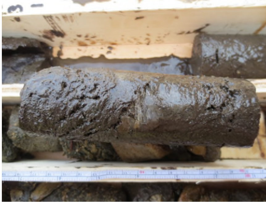
Photo 24: ICE and SILT with organics (black muck) encountered at a depth BGL of 0.6 m in Borehole GT-10, North WRSF. Photo taken on September 1, 2016.
