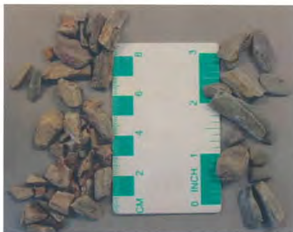
Figure 2. Quartz-mica schist and mica schist particles, which exhibit particle shapes trending towards flat and elongated.
