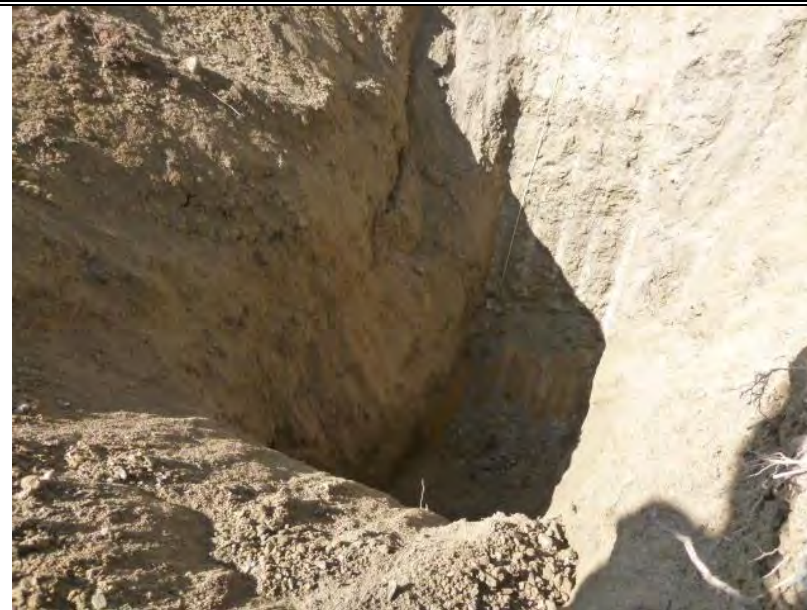
TP-BGC11-103 – Back wall of test pit; pit completed at a depth of 6.0 m.
