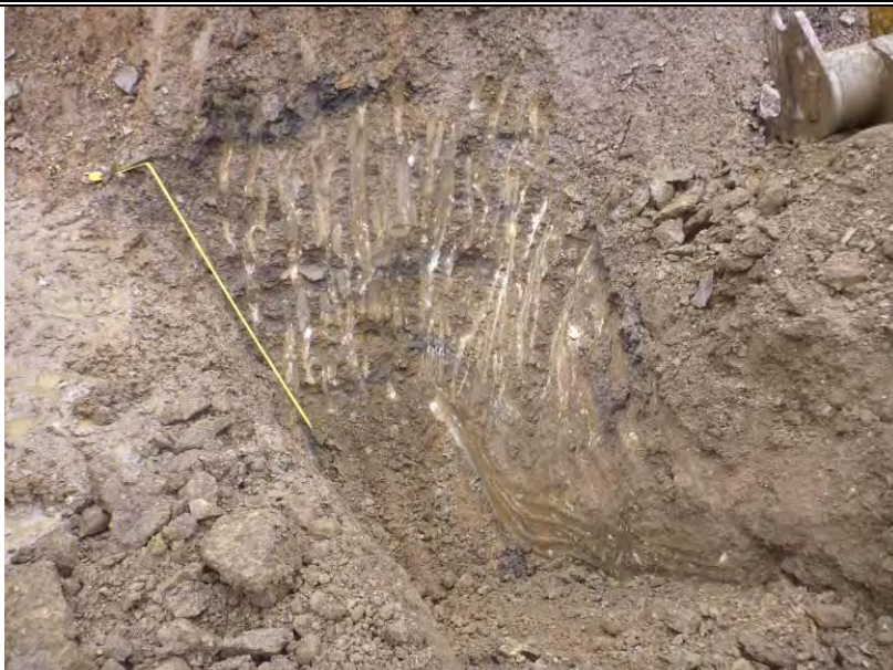
TP-BGC11-107 – Back wall of test pit; pit completed at a depth of 3.2 m.
