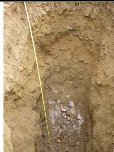
TP-BGC11-110 – Back wall of test pit; pit completed at a depth of 5.0 m.
