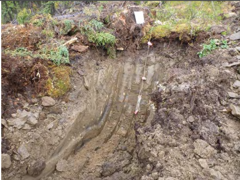
TP-BGC11-85 – Back wall of test pit; pit completed at a depth of 2.5 m.
