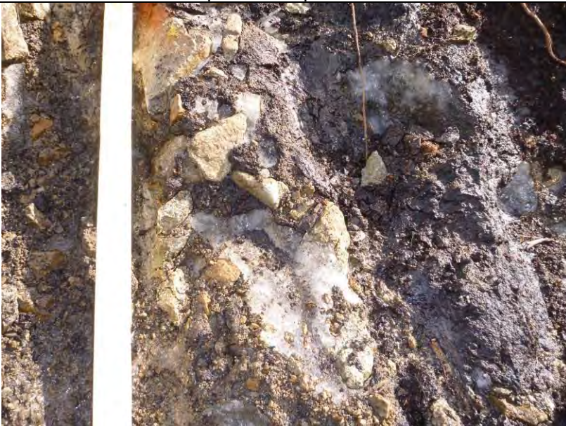
TP-BGC11-106 – Detail of visible ice in pit wall.
