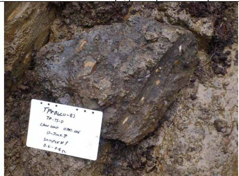
TP-BGC11-83 – Detail of frozen soil sample taken from 0.6-0.8 m.
