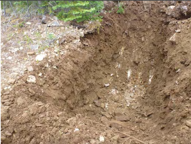
TP-BGC11-98 – Back wall of test pit; pit completed at a depth of 2.2 m.
