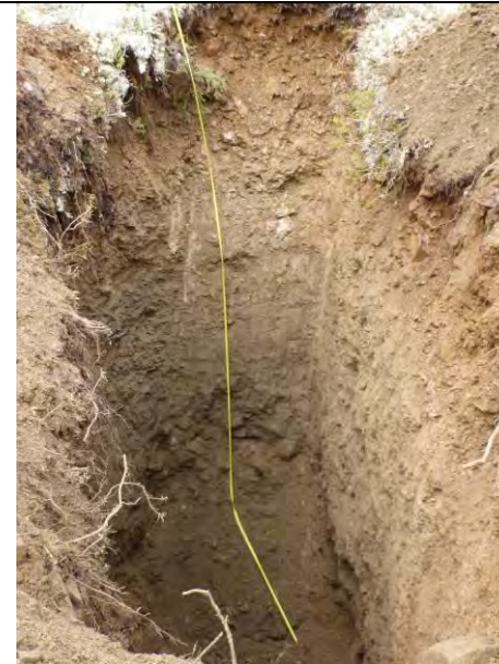
TP-BGC11-109 – Back wall of test pit; pit completed at a depth of 5.3 m.
