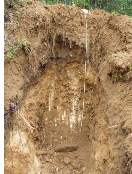
TP-BGC11-81 – Back wall of test pit; pit completed at a depth of 3.9 m.
