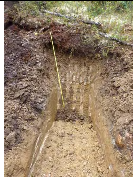
TP-BGC11-112 – Back wall of test pit; pit completed at a depth of 2.5 m.
