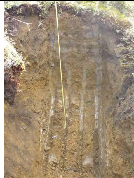
TP-BGC11-114 – Back wall of test pit; pit completed at a depth of 3.2 m.
