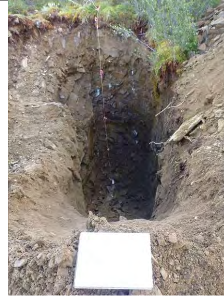
TP-BGC11-102 – Back wall of test pit; pit completed at a depth of 4.6 m.
