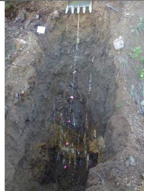
TP-BGC11-65 – Back wall of test pit; pit completed at depth of 8.0 m.
