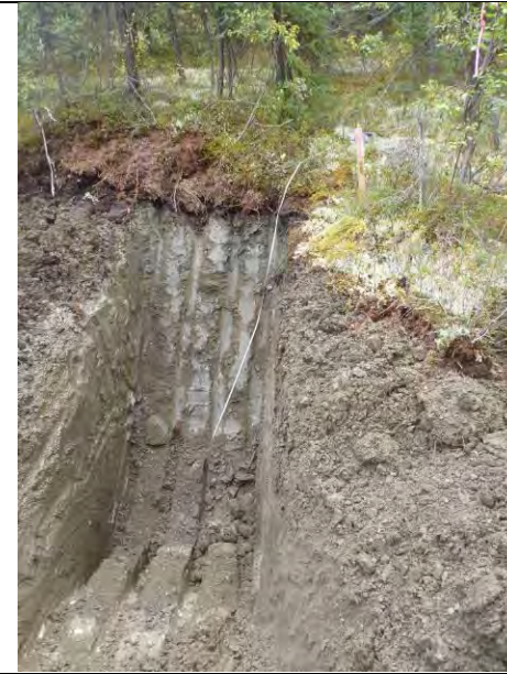
TP-BGC11-123 – Back wall of test pit; pit completed at a depth of 2.4 m.
