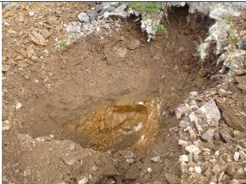
TP-BGC11-99 – Back wall of test pit; pit completed at a depth of 2.5 m.
