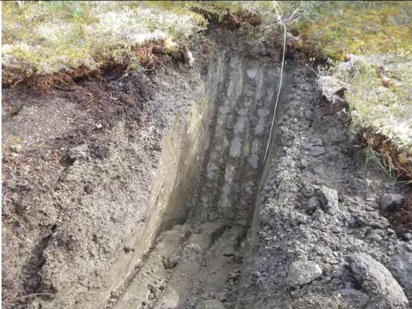
TP-BGC11-128 – Back wall of test pit; pit completed at a depth of 3.0 m.
