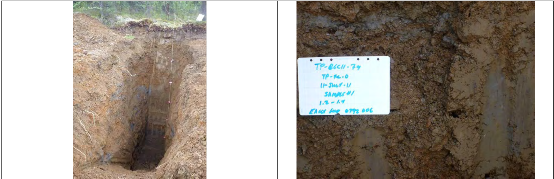
TP-BGC11-74 – Back wall of test pit; pit completed at 5.5 m.
