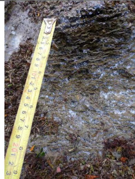
TP-BGC11-121 – Detail of lensed ice in pit wall.
