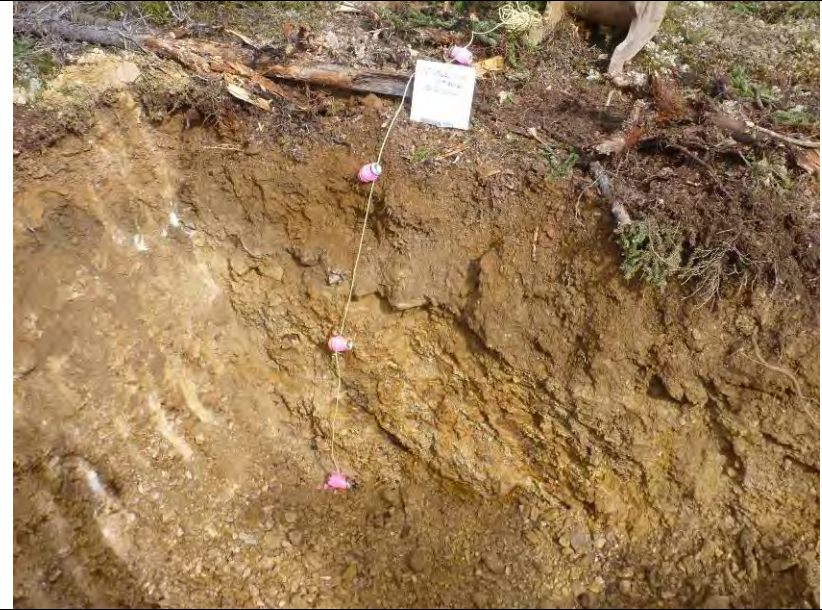
TP-BGC11-55 – Back wall of test pit; pit completed at depth of 2.0 m.
