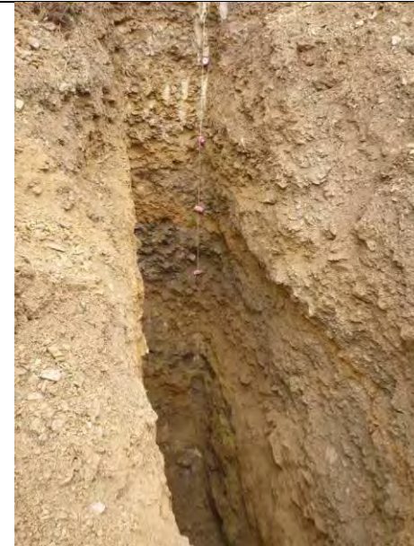
TP-BGC11-86 – Back wall of test pit; pit completed at a depth of 7.5 m.
