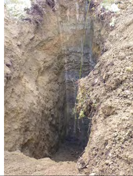
TP-BGC11-118 – Back wall of test pit; pit completed at a depth of 5.3 m.
