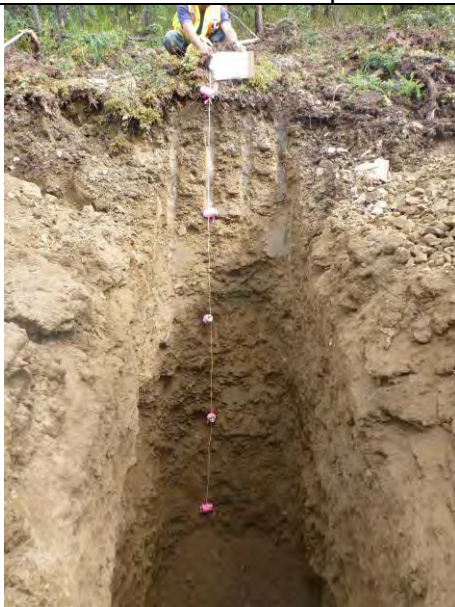
TP-BGC11-51 – Pit back wall; pit completed at a depth of 4.7 m.
