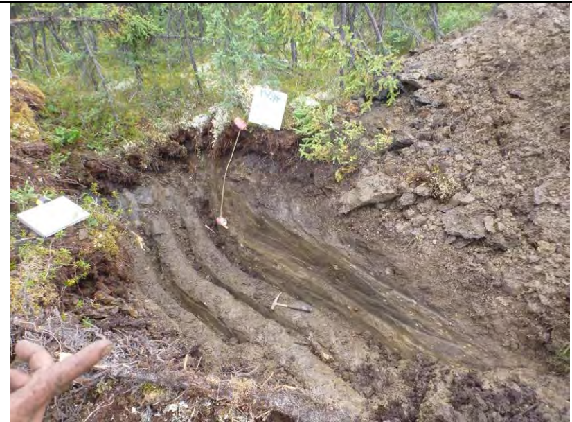
TP-BGC11-83 – Back wall of test pit; pit completed at a depth of 1.3 m.
