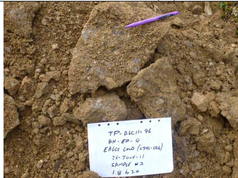
TP-BGC11-96 – Detail of frozen soil sample taken from 1.8-2.0 m.
