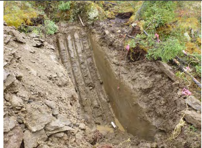
TP-BGC11-93 – Back wall of test pit; pit completed at a depth of 1.85 m.
