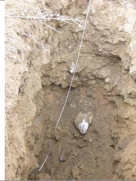
TP-BGC11-134 – Back wall of test pit; pit completed at a depth of 4.2 m.
