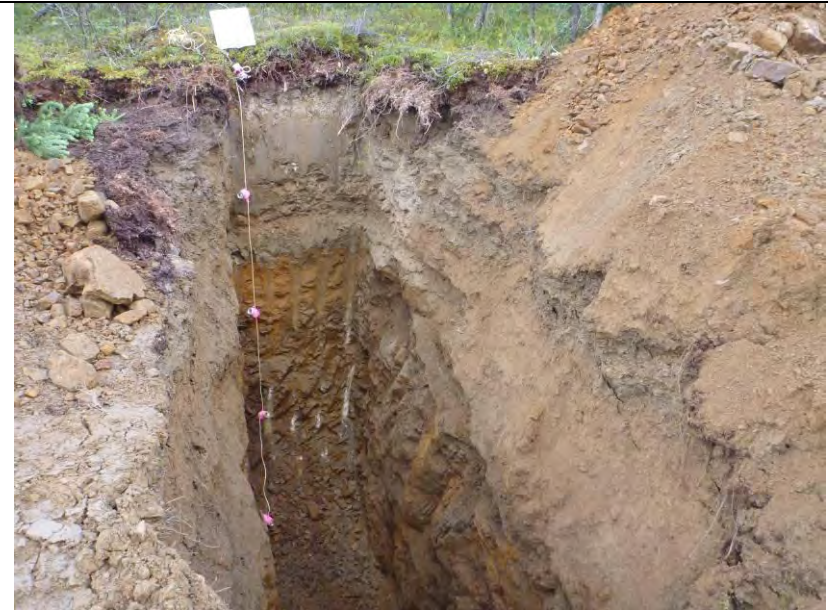
TP-BGC11-64 – Back wall of test pit; pit completed at depth of 4.7 m.
