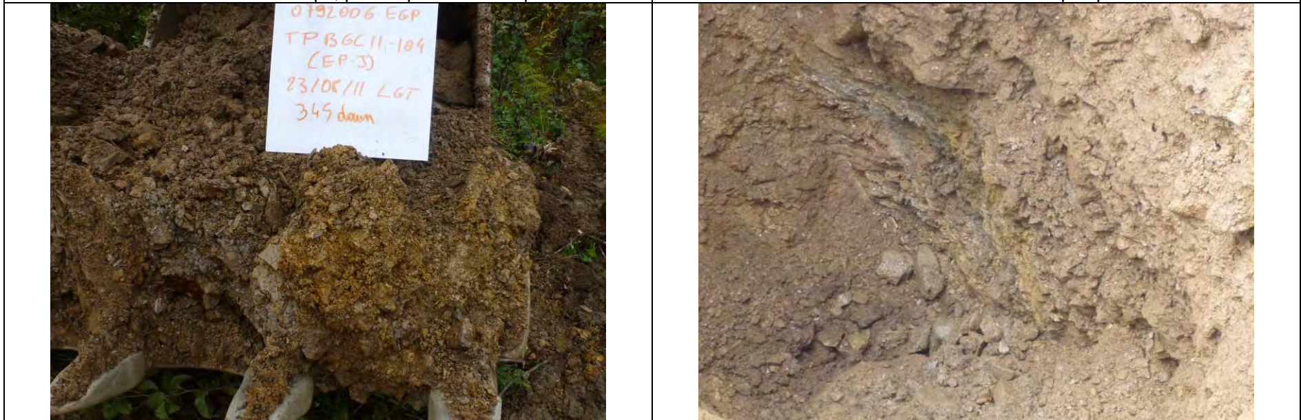
TP-BGC11-104 – Detail of an excavated bucket from below 3.45 m.
