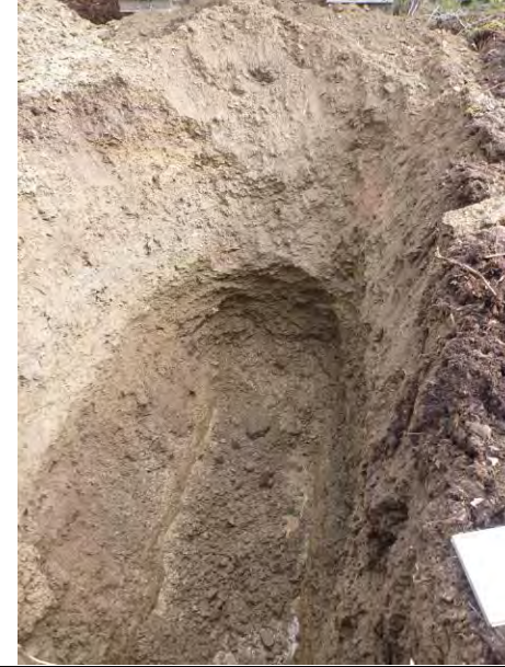
TP-BGC11-126 – Back wall of test pit; pit completed at a depth of 3.1 m.
