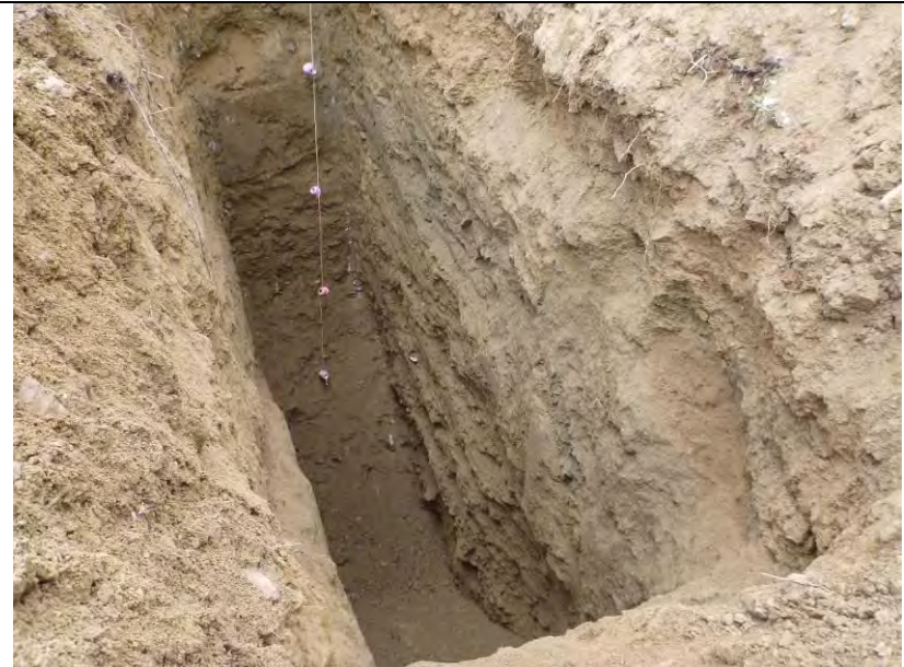
TP-BGC11-62 – Bottom of test pit; pit completed at depth of 6.2 m.
