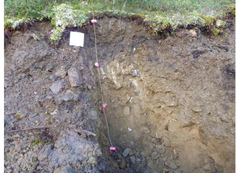
TP-BGC11-59 – Cut slope and test pit; pit completed at depth of 2.6 m.
