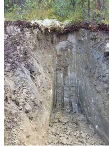
TP-BGC11-121 – Back wall of test pit; pit completed at a depth of 3.3 m.
