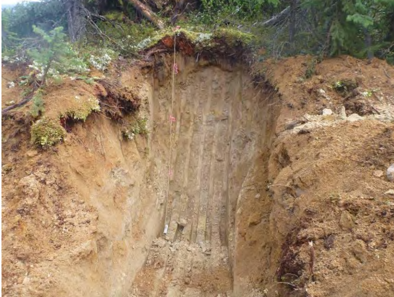
TP-BGC11-95 – Back wall of test pit; pit completed at a depth of 3.2 m.
