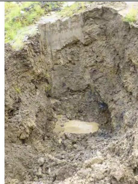
TP-BGC11-113 – Back wall of test pit; pit completed at a depth of 2.5 m.
