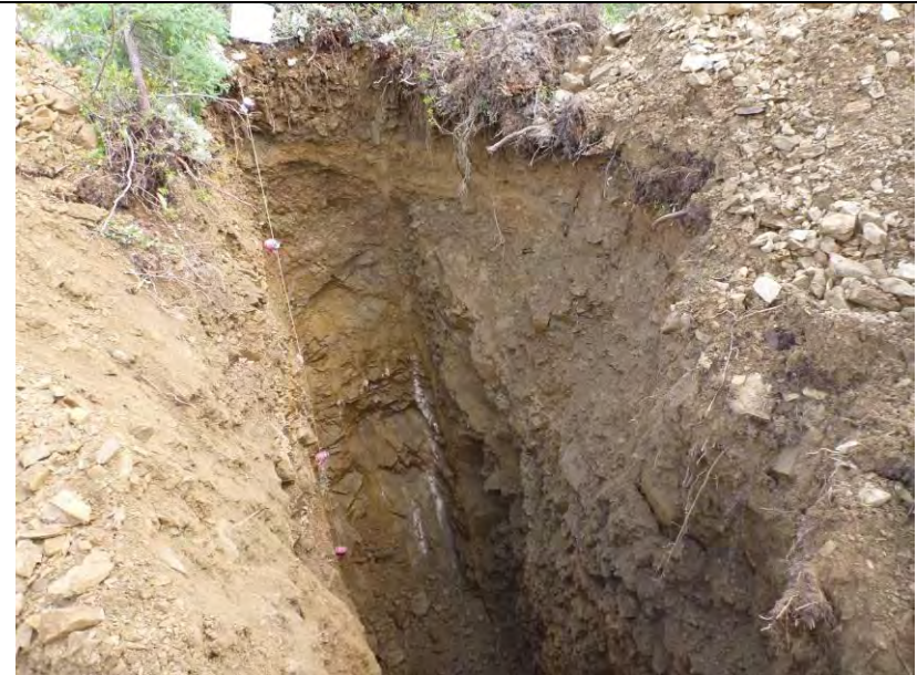
TP-BGC11-63 – Back wall of test pit; pit completed at depth of 4.6 m.
