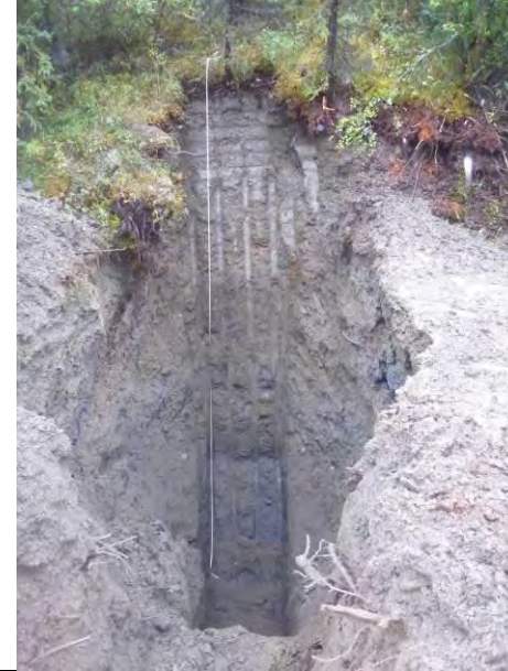
TP-BGC11-129 – Back wall of test pit; pit completed at a depth of 6.8 m.
