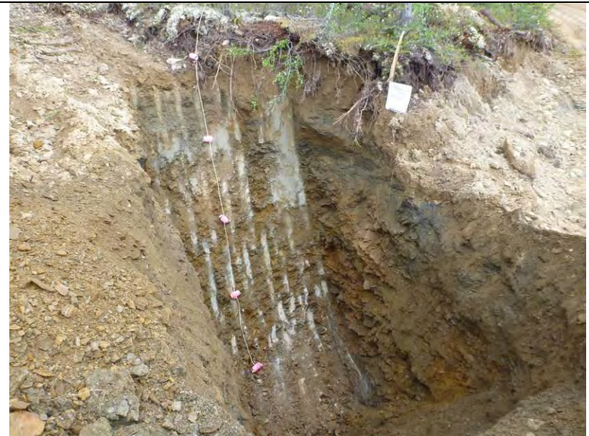
TP-BGC11-53 – Cut slope and test pit; pit completed at depth of 4.0 m.
