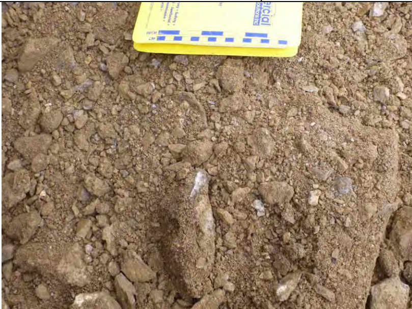
TP-BGC11-112 – Detail of a bucket excavated from 2.5 m.
