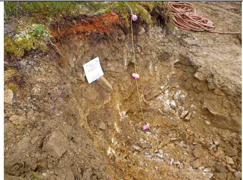
TP-BGC11-54 – Back wall of test pit; pit completed at depth of 2.0 m.
