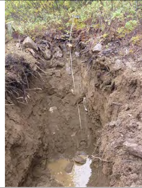
TP-BGC11-131 – Back wall of test pit; pit completed at a depth of 3.5 m.
