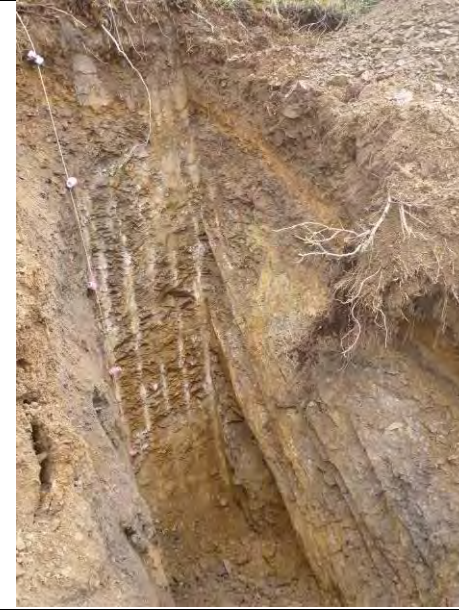
TP-BGC11-77 – Back wall of test pit; pit completed at a depth of 5.5 m.
