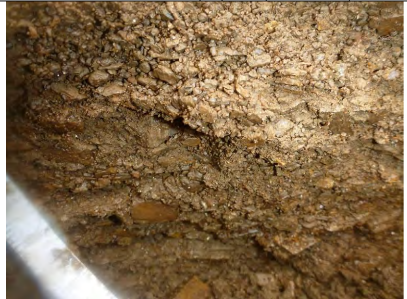
TP-BGC11-131 – Detail of fluvial material in pit wall.
