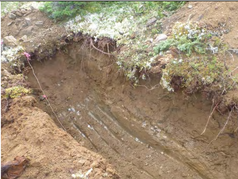
TP-BGC11-96 – Back wall of test pit; pit completed at a depth of 2.0 m.
