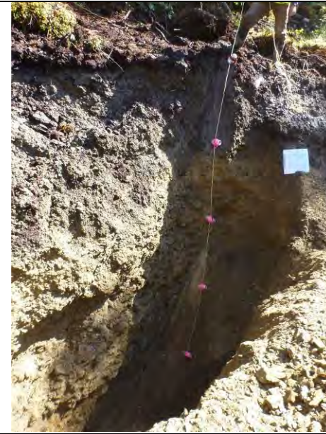
TP-BGC11-72 – Back wall of test pit; pit completed at depth of 4.3 m.
