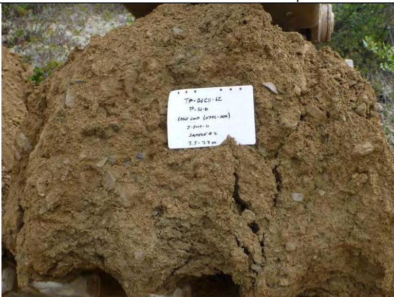
TP-BGC11-62 – Detail of a bucket excavated from 3.5-3.7 m.
