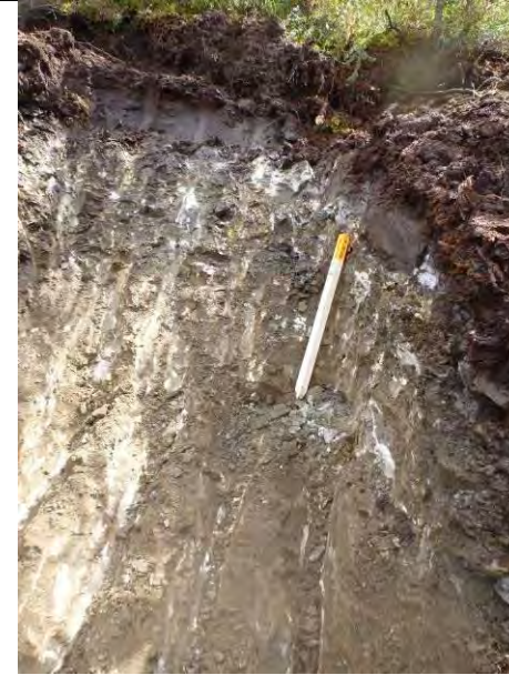
TP-BGC11-101 – Back wall of test pit; pit completed at a depth of 2.4 m.
