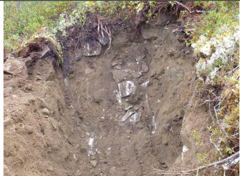
TP-BGC11-111 – Back wall of test pit; pit completed at a depth of 2.0 m.
