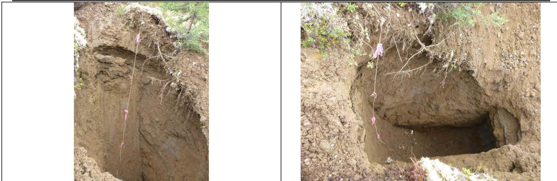
TP-BGC11-90 – Back wall of test pit; pit completed at a depth of 6.5 m.
