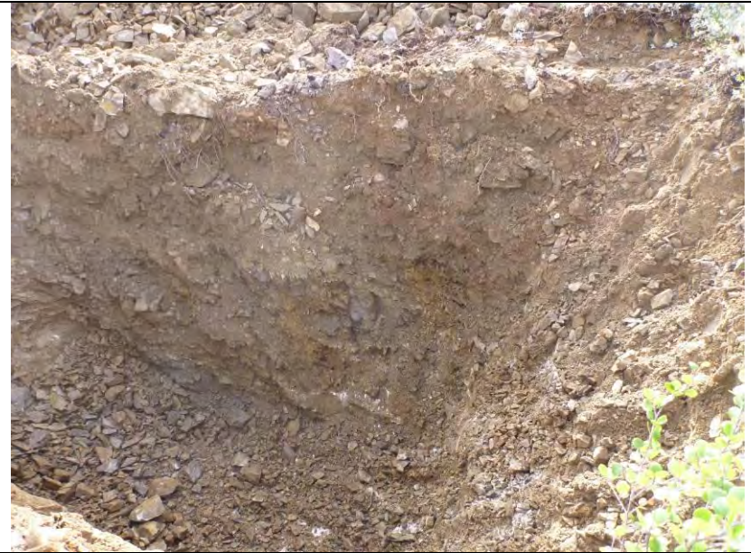
TP-BGC11-127 – Pit completed at a depth of 2.5 m.
