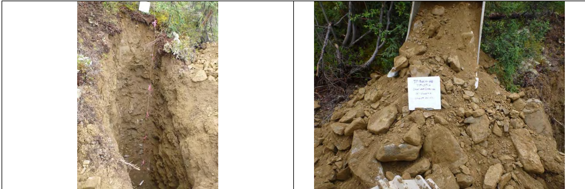
TP-BGC11-88 – Back wall of test pit; pit completed at a depth of 6.0 m.
