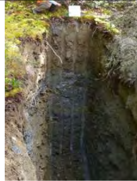
TP-BGC11-140 – Back wall of test pit; pit completed at a depth of 4.5 m.
