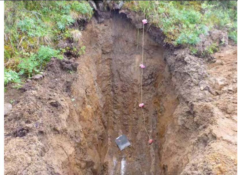
TP-BGC11-87 – Back wall of test pit; pit completed at a depth of 3.5 m.
