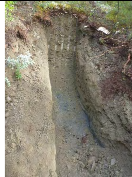
TP-BGC11-105 – Back wall of test pit; pit completed at a depth of 3.0 m.
