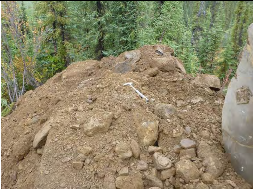
TP-BGC11-134 – Spoil pile (hammer for scale).
