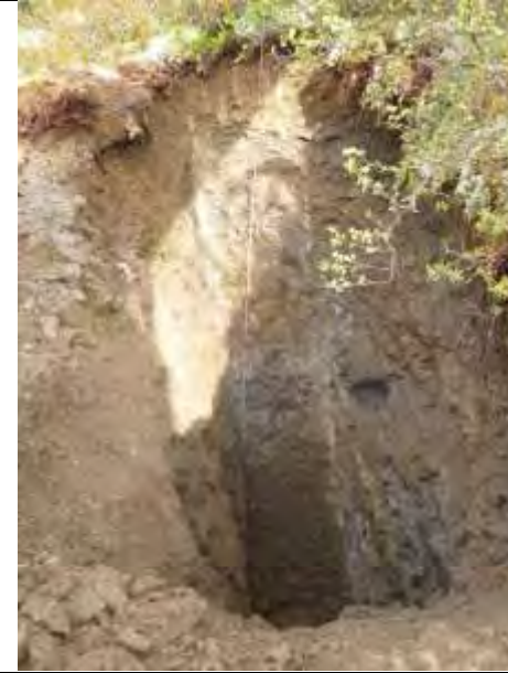
TP-BGC11-137 – Back wall completed to depth of 5.0 m.
