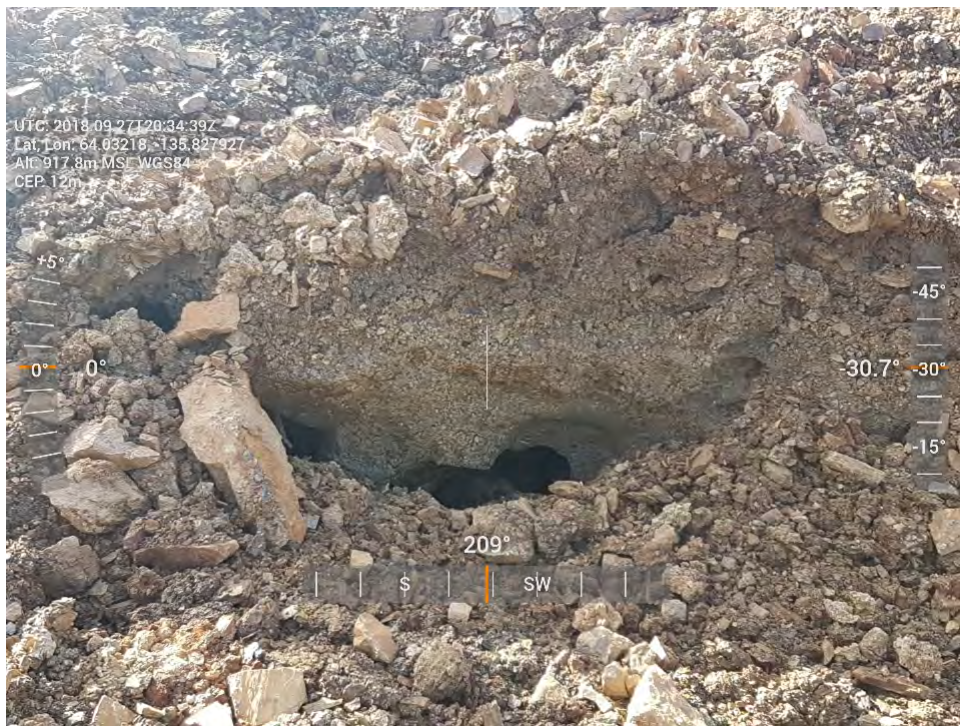
Figure 53: Stockpile B - Ice found in Northwest material flow.
