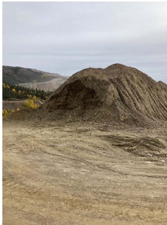
Figure 80: Some stockpiles with steep side slopes
