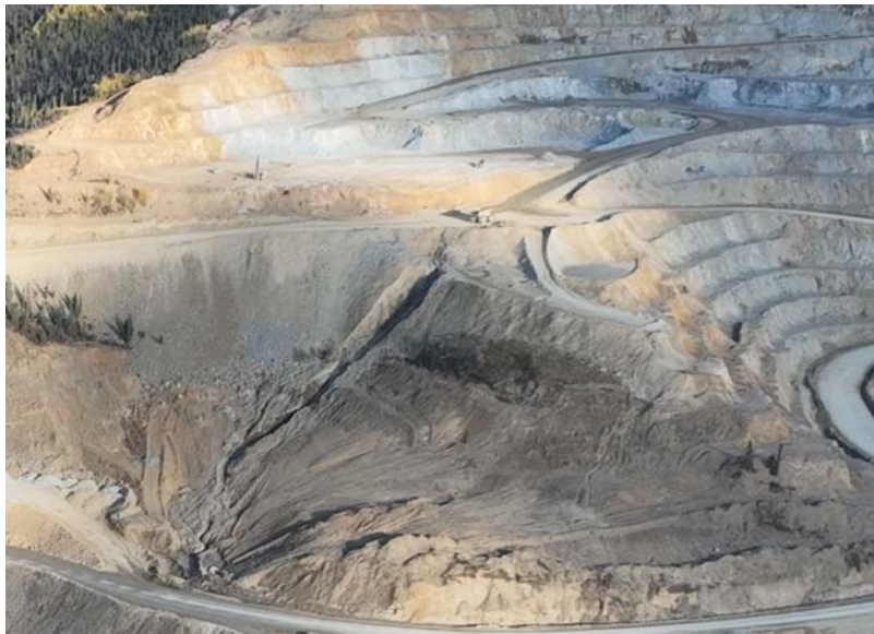
Figure 29: Open Pit Erosion – Aerial View 2022
