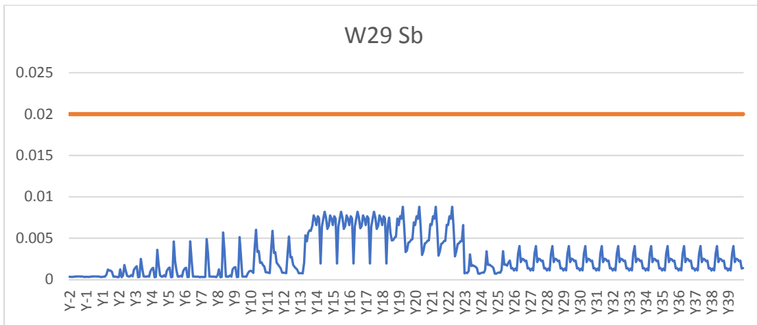
A.2-7: Time series of predicted antimony concentrations (mg/L) for W29. Water Quality Objective is shown by red line.
