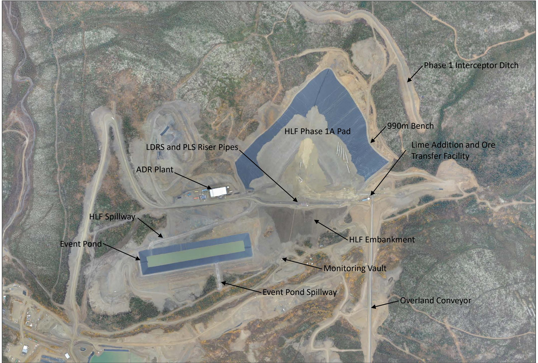
Figure A1 Site Aerial Photograph (provided by Strata Gold Corp and taken September 16, 2019)
