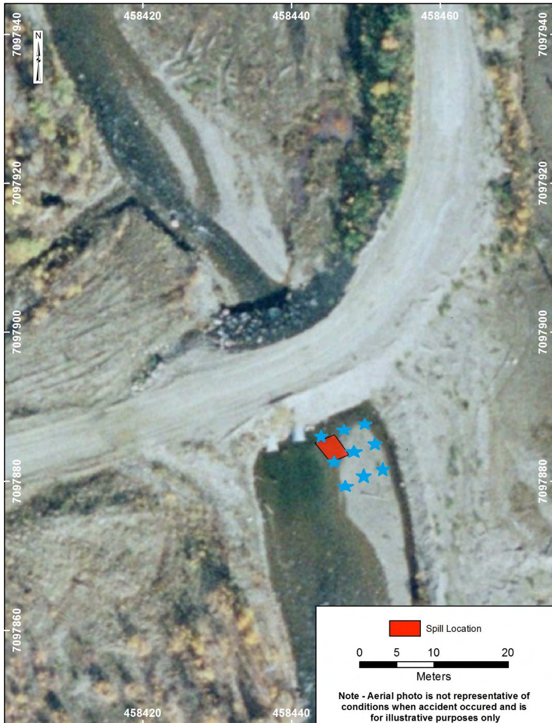
Figure 4-4: Soil Future planned soil sample locations - multiple depths in a grid pattern
