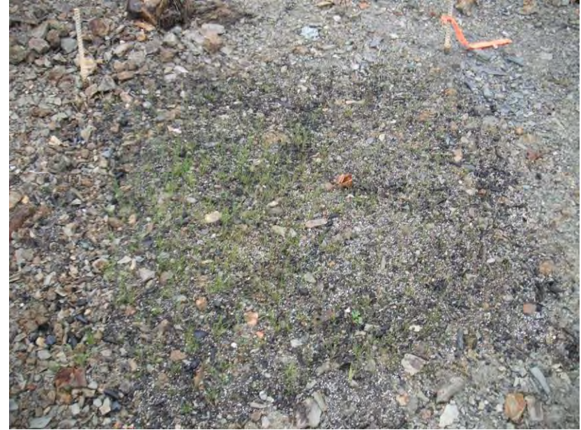
Photo #62: Waste Rock, Plot 2-4, July 2013. Dolomite granules can still be seen.
