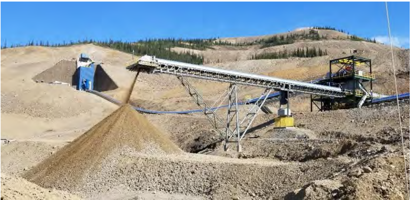
Photo 2.1-11: Primary Crusher Feed to Reclaim Stockpile - June 11, 2019
