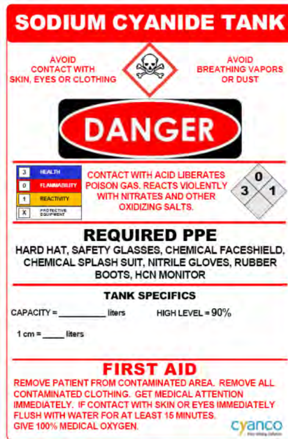
Figure 5: Example of Labeling for Transport, Storage and Use of Hazardous Materials
