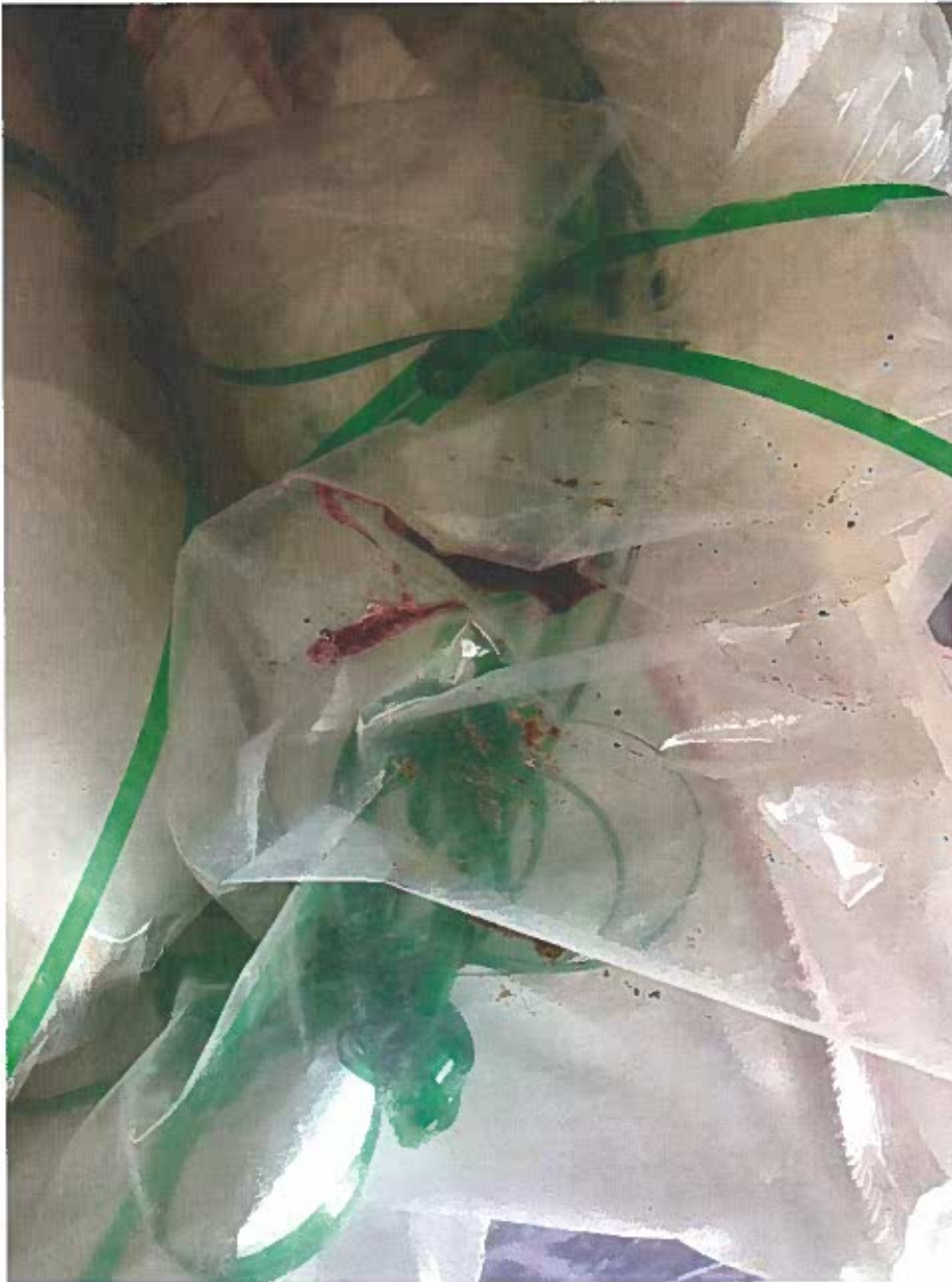
Improper – Cyanide Residue outside of clear IBC liner plastic bag
